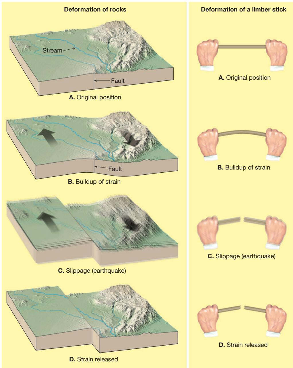
**FIGURE 11.5** Elastic rebound. As rock is deformed, it bends, storing elastic energy. Once strained beyond its breaking point, the rock cracks, releasing the stored-up energy in the form of earthquake waves.
