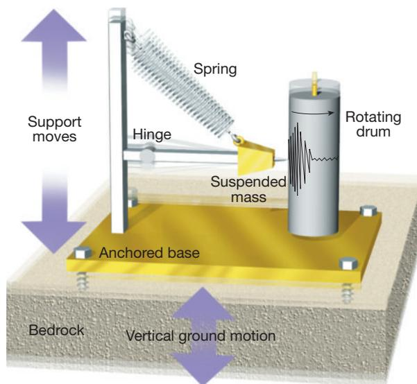
FIGURE 11.8 Seismograph designed to record vertical ground motion.
