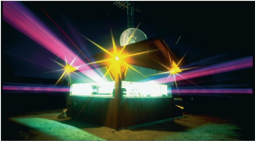
**FIGURE 11.25** Lasers used to measure movement along the San Andreas Fault. (Photo by John K. Nakata/U.S. Geological Survey)
