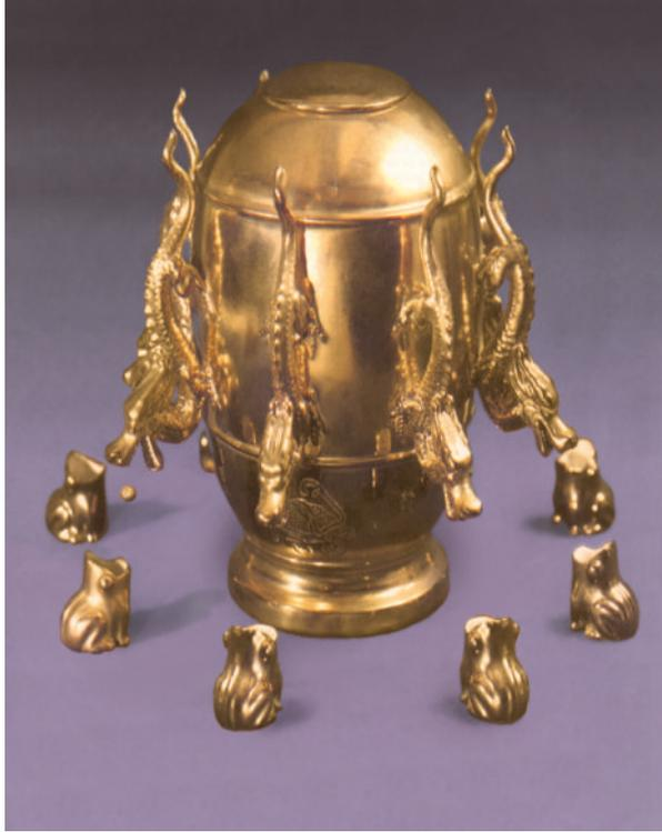
**FIGURE 11.6** Ancient Chinese seismograph. During an Earth tremor, the dragons located in the direction of the main vibrations would drop a ball into the mouths of the frogs below.
