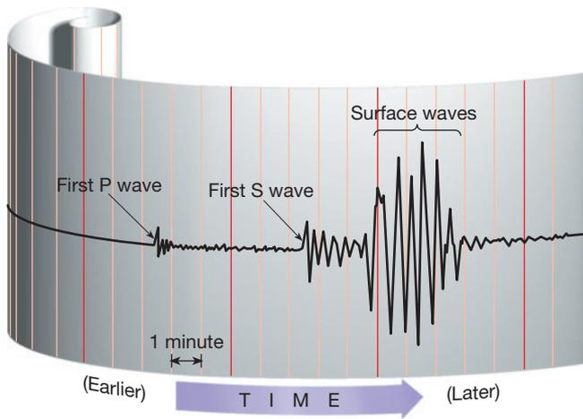
**FIGURE 11.10** Typical seismogram. Note the time interval (about 5 minutes) between the arrival of the first P wave and the arrival of the first S wave.
