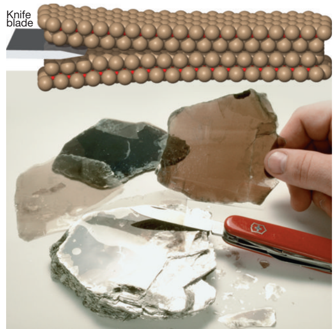
FIGURE 3.21 The thin sheets shown here were produced by splitting a mica (muscovite) crystal parallel to its perfect cleavage. (Photo by Breck P. Kent)
