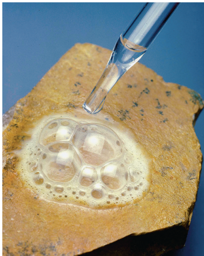
FIGURE 3.25 Calcite reacting with a weak acid. (Photo by Chip Clark)
