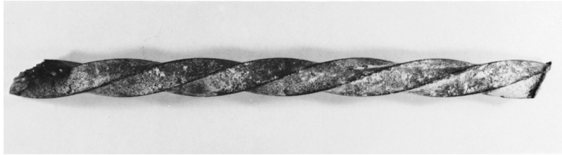
Twisted square bar, formerly used to increase bond between concrete and steel. (Courtesy of Clemson University Communications Center.)
