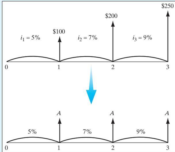
**Figure 4.13** Equivalence calculation with changing interest rates (Example 4.11).
