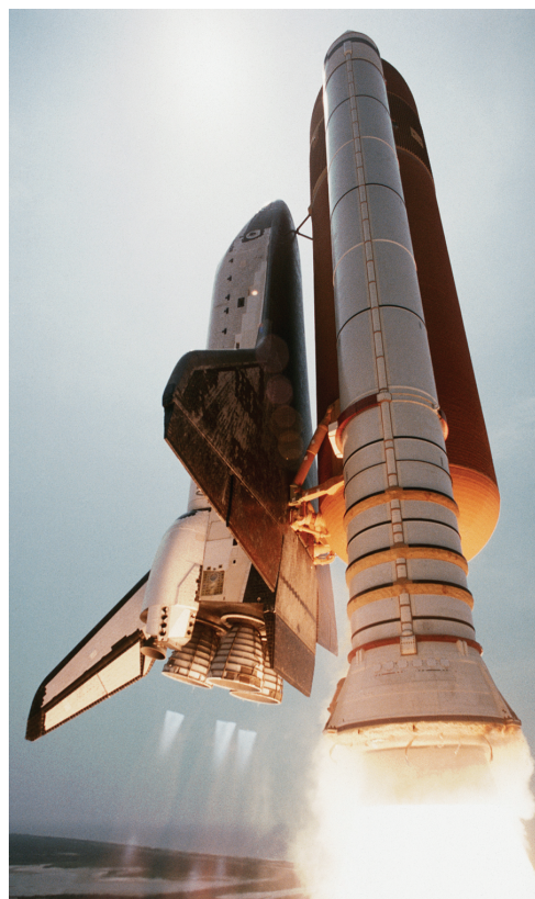
FIG. 2.14 Hydrogen reacts with oxygen to form water. The reaction of hydrogen with oxygen provides the thrust for the main rocket engines of the space shuttle shown here just after liftoff. (Corbis Images.)
