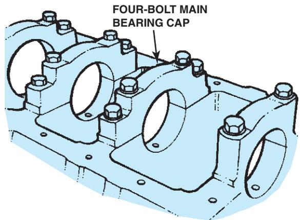
**FIGURE 26-13** High-performance and truck engines often use four-bolt main bearing caps for greater durability.
