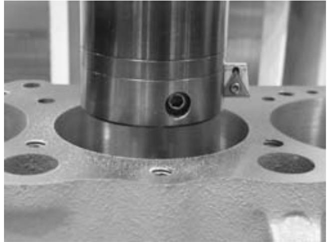
**FIGURE 26-22** A cylinder boring machine is to enlarge cylinder bore diameter so a replacement oversize piston can be used to restore a worn engine to useful service or to increase the displacement of the engine in an attempt to increase power output.
