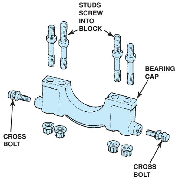
**FIGURE 26-14** Some engines add to the strength of a four-bolt main bearing cap by also using cross bolts through the bolt on the sides of the main bearing caps.
