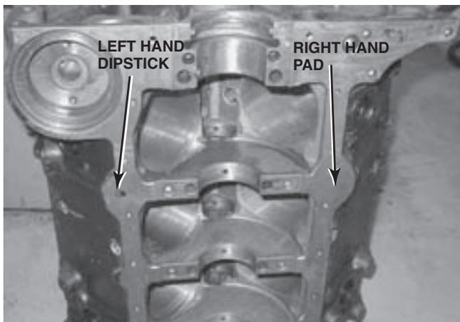
**FIGURE 26-11** Small-block Chevrolet block. Note the left-hand dipstick hole and a pad cast for a right-hand dipstick.
