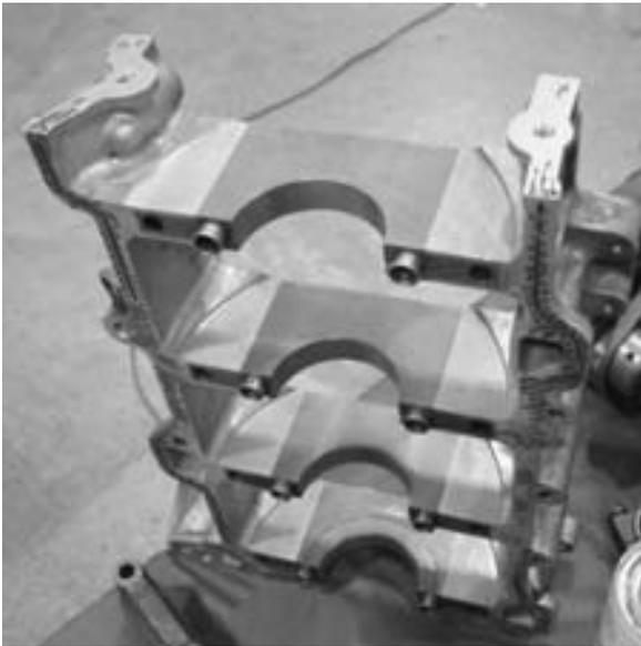
**FIGURE 26-6** A bedplate is a structural part of the engine that is attached between the block and the oil pan and supports the crankshaft.
