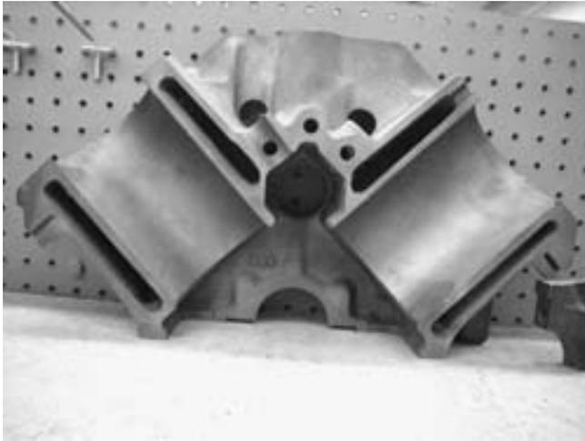
**FIGURE 26-8** Cutaway of a Chevrolet V-8 block showing all of the internal passages.
