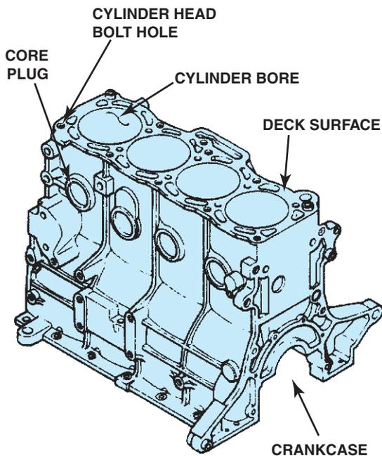
**FIGURE 26-1** The cylinder block usually extends from the oil pan rails at the bottom to the deck surface at the top.
