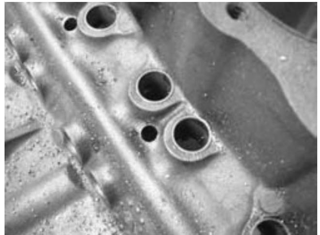
**FIGURE 26-34** High-performance engine builders will often install bronze sleeves in the valve lifter bores.
