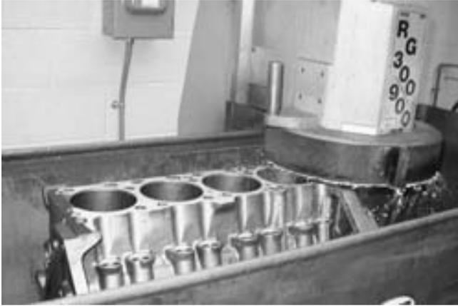
**FIGURE 26-19** Grinding the deck surface of the block.
