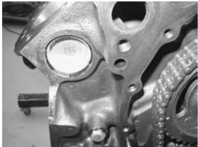
**FIGURE 26-2** An expansion plug is used to block the opening in the cylinder head or block the holes where the core sand was removed after the part was cast.
