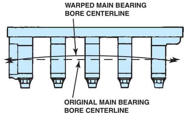
**FIGURE 26-15** The main bearing bores of a warped block usually bend into a bowed shape. The greatest distortion is in the center bores.
