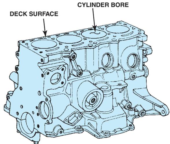
**FIGURE 26-7** The deck is the machined top surface of the block. Note all of the passages and holes that are part of the typical block.
