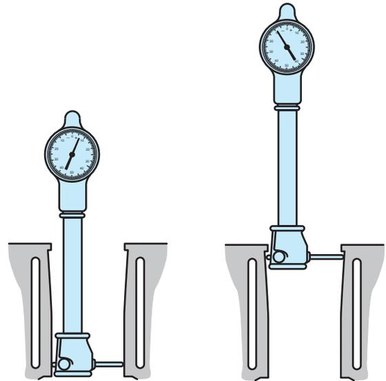
**FIGURE 26-21** Using a dial bore gauge to measure the bore diameter at the top just below the ridge and at the bottom below the ring travel. Take the measurements in line with the crankshaft and then repeat the measurements at right angles to the centerline of the block in each cylinder.
