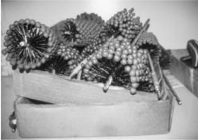
**FIGURE 26-24** An assortment of ball-type deglazing hones. This type of hone does not straighten wavy cylinder walls.
