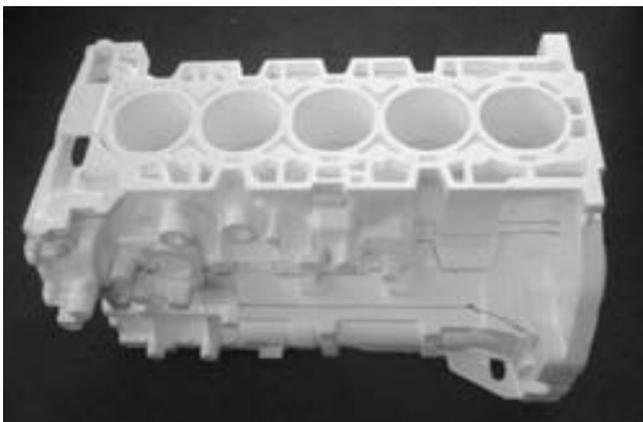
**FIGURE 26-3** A Styrofoam casting mold used to make the five-cylinder engine blocks for the Chevrolet Colorado and the Hummer H3. The brown lines are glue used to hold the various parts together. Sand is packed around the mold and molten aluminum is poured into the sand, which instantly vaporizes the Styrofoam. The aluminum then flows and fills the area of the mold.
