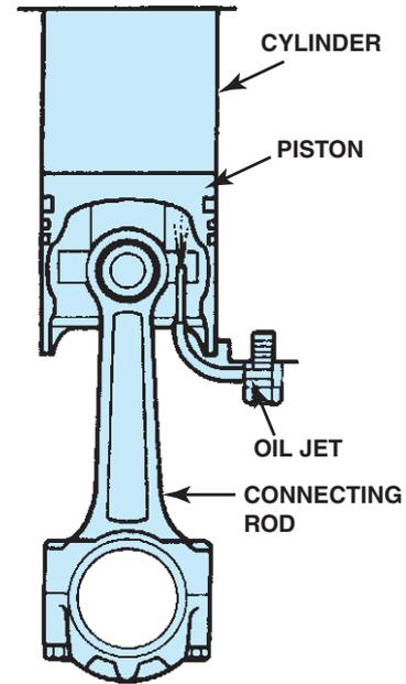
**FIGURE 26-9** Oil jets are often used in some turbocharged, and many diesel, engines to cool the pistons.
