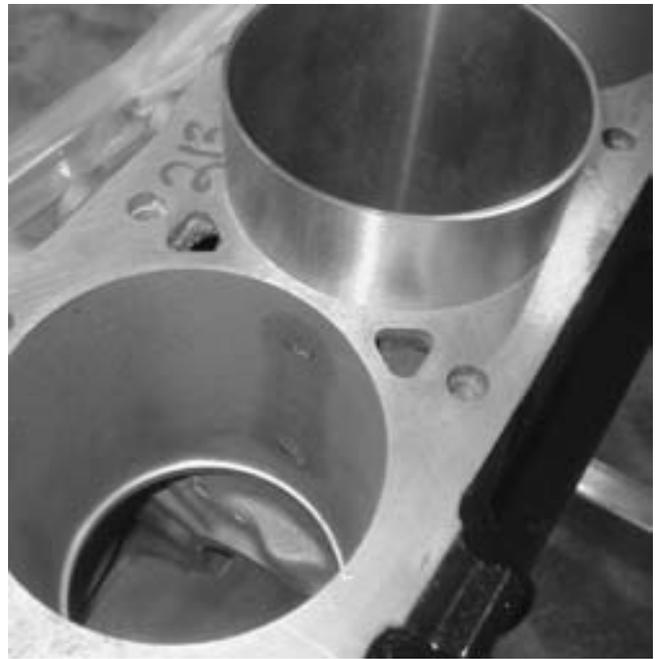
**FIGURE 26-23** A dry cylinder sleeve can also be installed in a cast-iron block to repair a worn or cracked cylinder.
