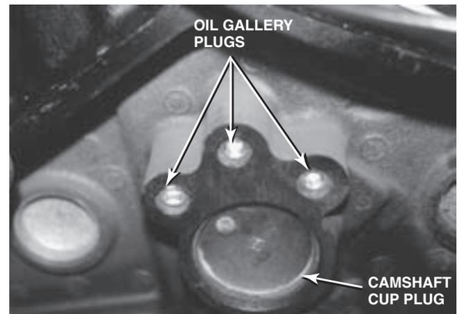
**FIGURE 26-10** Typical oil gallery plugs on the rear of a Chevrolet small-block V-8 engine.
