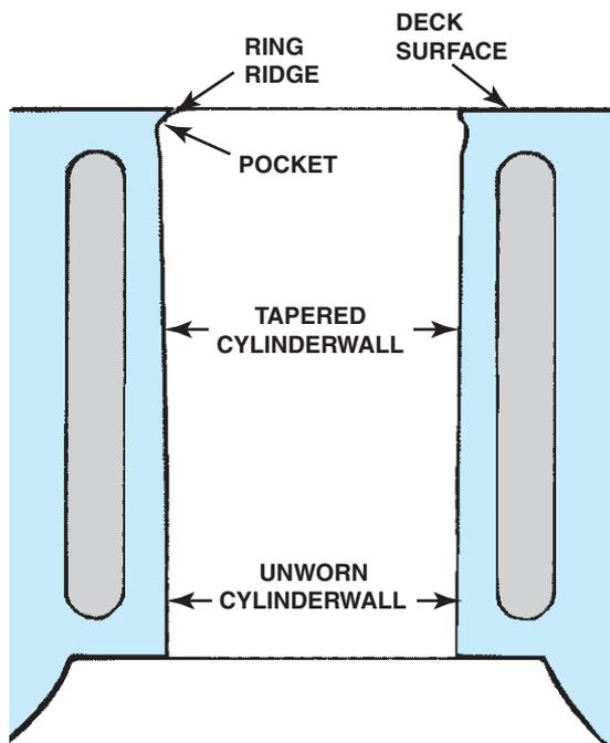
**FIGURE 26-20** Cylinders wear in a taper, with most of the wear occurring at the top of the cylinder where the greatest amount of heat is created. The ridge is formed because this very top part of the cylinder is not worn by the rings.
