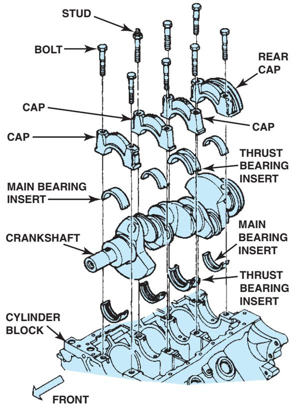
**FIGURE 26-12** Two-bolt main bearing caps provide adequate bottom end strength for most engines.
