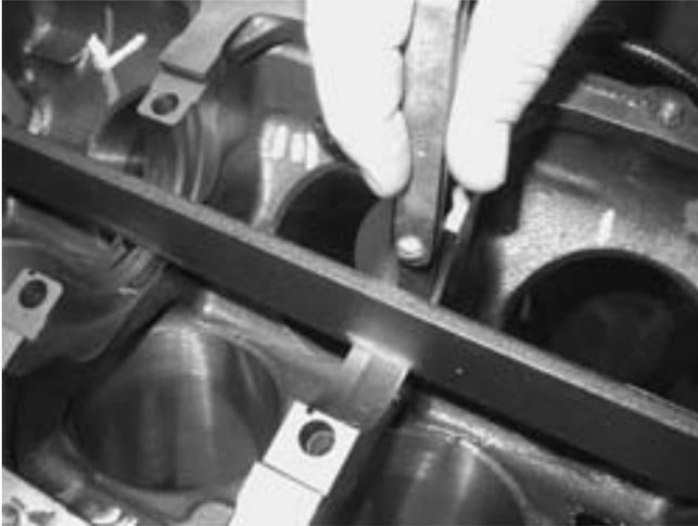
**FIGURE 26-17** The main bearing bores can be checked using a precision straightedge and a feeler gauge.
