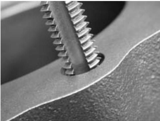
**FIGURE 26-33** A thread chaser or bottoming tap should be used in all threaded holes before assembling the engine.
