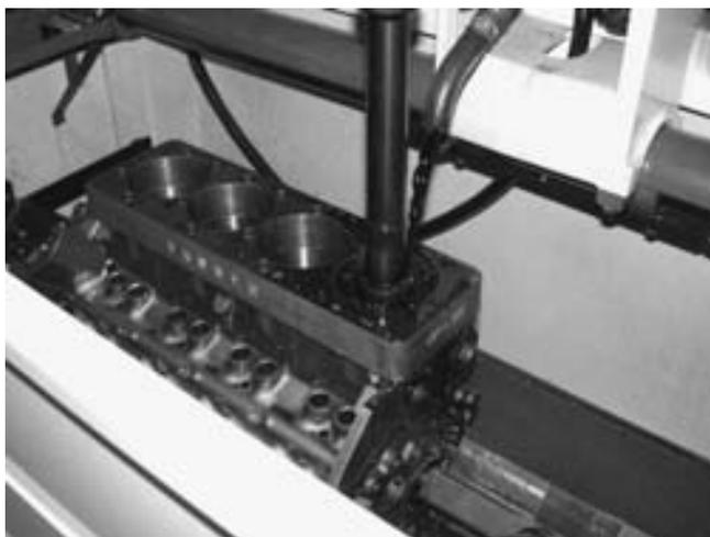
**FIGURE 26-27** A torque plate being used during a cylinder honing operation. The thick piece of metal is bolted to the block and simulates the forces exerted on the block by the head bolts when the cylinder head is attached.
