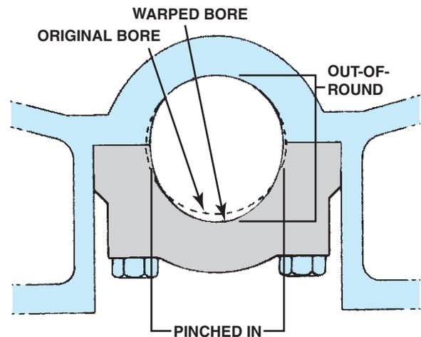
**FIGURE 26-16** When the main bearing caps bow downward, they also pinch in at the parting line.
