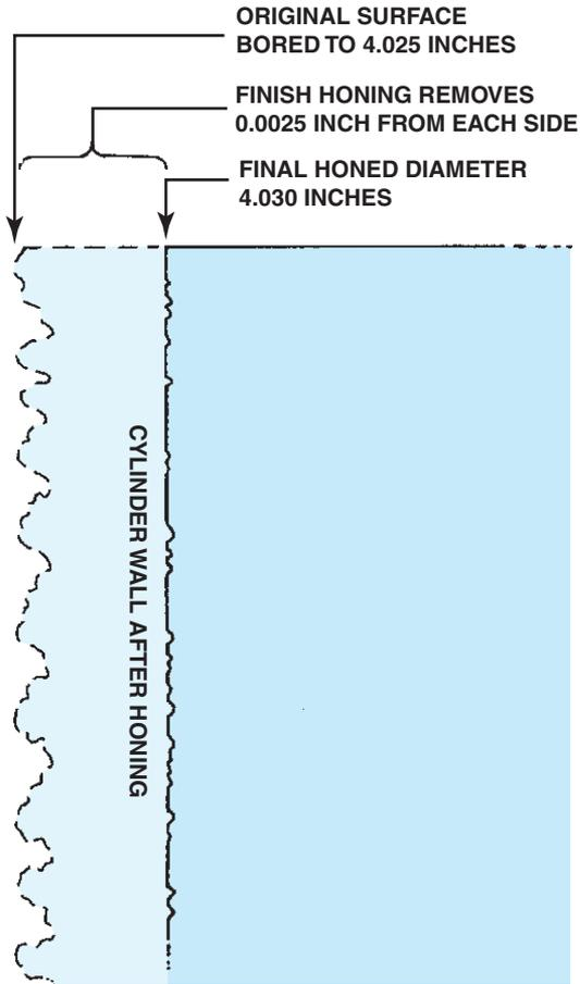
**FIGURE 26-26** Honing enlarges the cylinder bore to the final size and leaves a plateau surface finish that retains oil.
