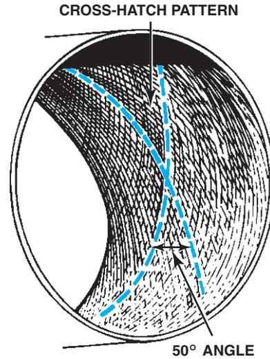
**FIGURE 26-28** The crosshatched pattern holds oil to keep the rings from wearing excessively, and also keeps the rings against the cylinder wall for a gas-tight fit.
