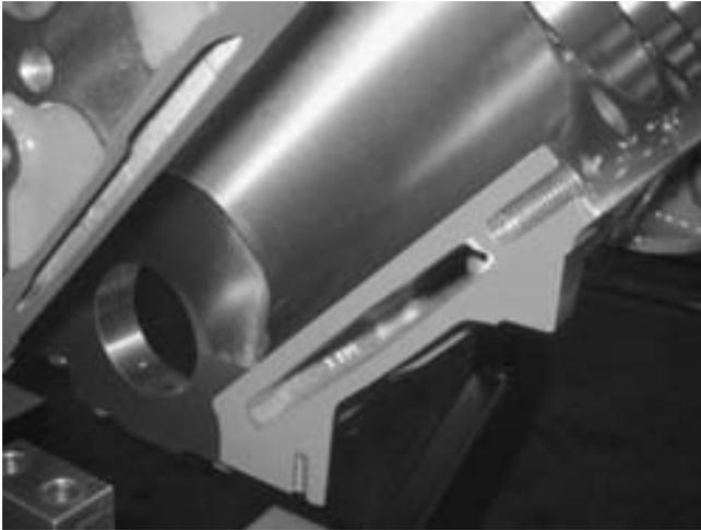
**FIGURE 26-32** Notice on this cutaway engine block that some of the head bolt holes do not extend too far into the block and dead end. Debris can accumulate at the bottom of these holes and it must be cleaned out before final assembly.
