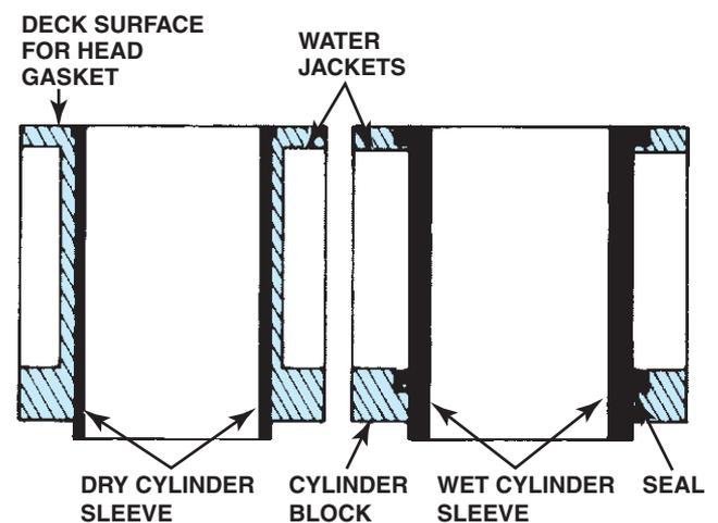
**FIGURE 26-5** A dry sleeve is supported by the surrounding cylinder block. A wet sleeve must be thicker to be able to withstand combustion pressures without total support from the block.
