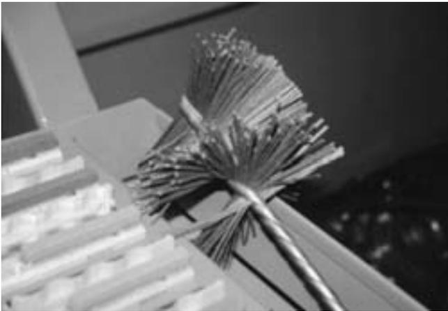
**FIGURE 26-30** To achieve a finer surface finish, use a soft hone that is made from nylon bristles with impregnated abrasive. This hone is ideal for engines using low tension piston rings and provides a smooth surface that allows the rings to seal immediately.
