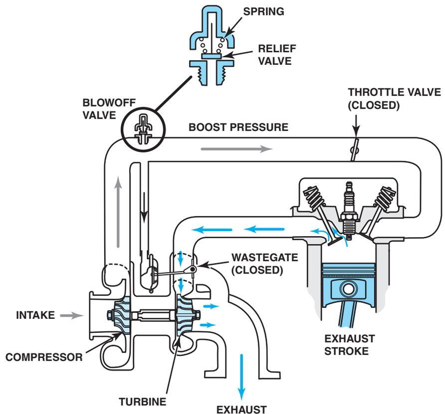
**FIGURE 19-12** A blow-off valve is used in some turbocharged systems to relieve boost pressure during deceleration.
