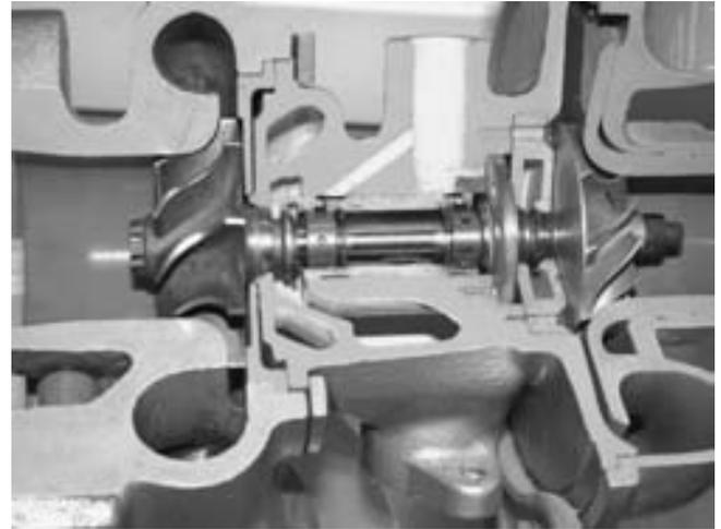
**FIGURE 19-9** The exhaust drives the turbine wheel on the left, which is connected to the impeller wheel on the right through a shaft. The bushings that support the shaft are lubricated with engine oil under pressure.
