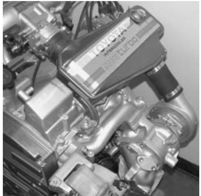
**FIGURE 19-2** A turbocharger on a Toyota engine.
