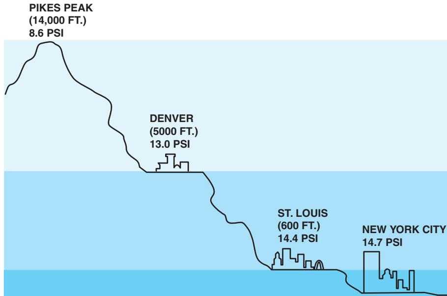
**FIGURE 19-4** Atmospheric pressure decreases with increases in altitude.
