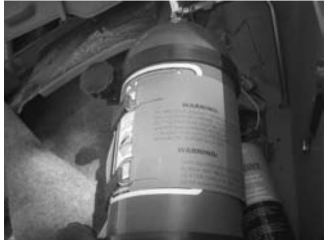
**FIGURE 19-15** An electrical heating mat is installed on the bottle of nitrous oxide to increase the pressure of the gas inside.
