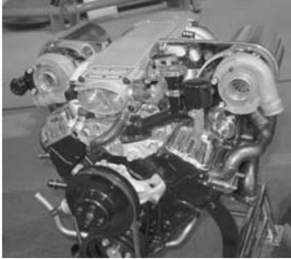
**FIGURE 19-13** A dual turbocharger system installed on a small block Chevrolet V-8 engine.
