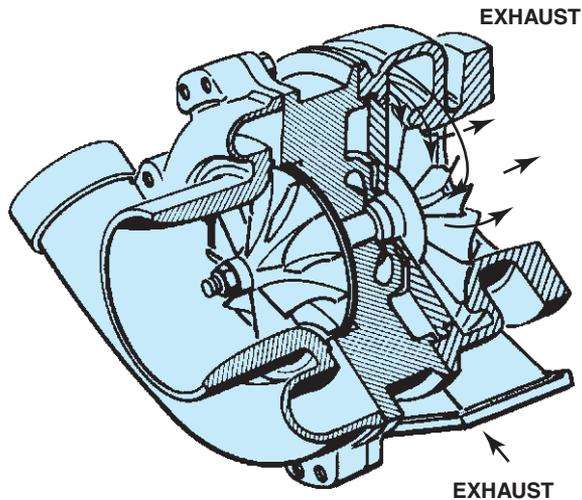
**FIGURE 19-8** A turbine wheel is turned by the expanding exhaust gases.
