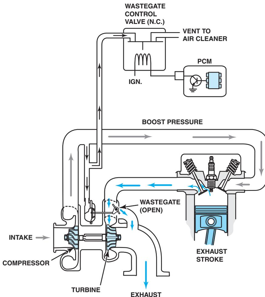
**FIGURE 19-11** A wastegate is used on the first-generation Duramax diesel to control maximum boost pressure.
