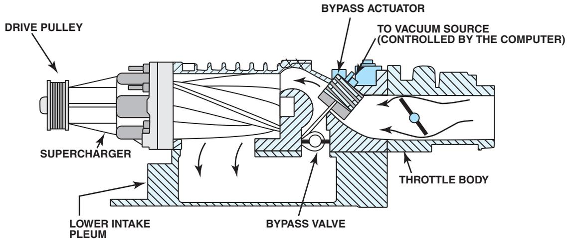
**FIGURE 19-6** The bypass actuator opens the bypass valve to control boost pressure.
