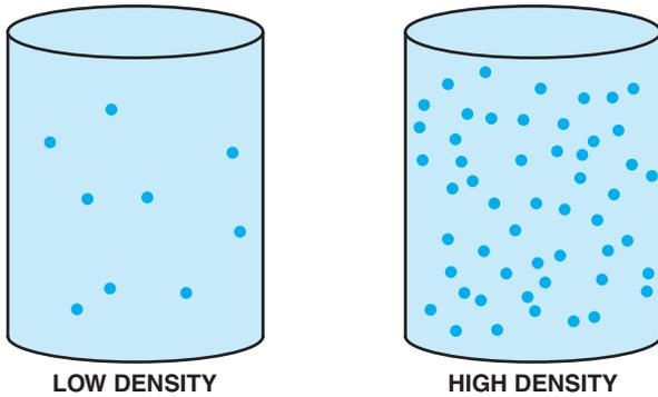
**FIGURE 19-3** The more air and fuel that can be packed in a cylinder, the greater the density of the air–fuel charge.
