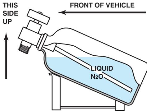
**FIGURE 19-14** Nitrous bottles have to be mounted at an angle to ensure that the pickup tube is in the liquid  $N_2O$ .
