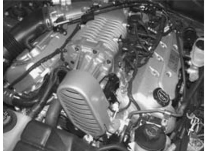
**FIGURE 19-1** A supercharger on a Ford V-8.
