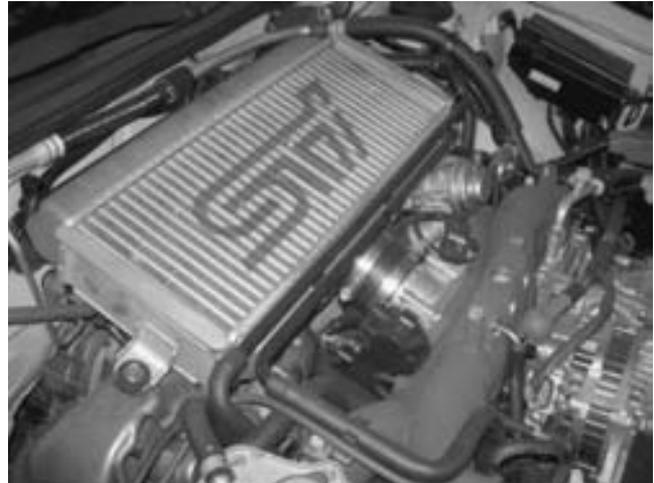
**FIGURE 19-10** The unit on top of this Subaru that looks like a radiator is the intercooler, which cools the air after it has been compressed by the turbocharger.
