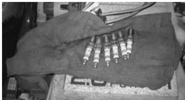
**FIGURE 16-32** When removing spark plugs, it is wise to arrange them so that they can be compared and any problem be identified with a particular cylinder.
