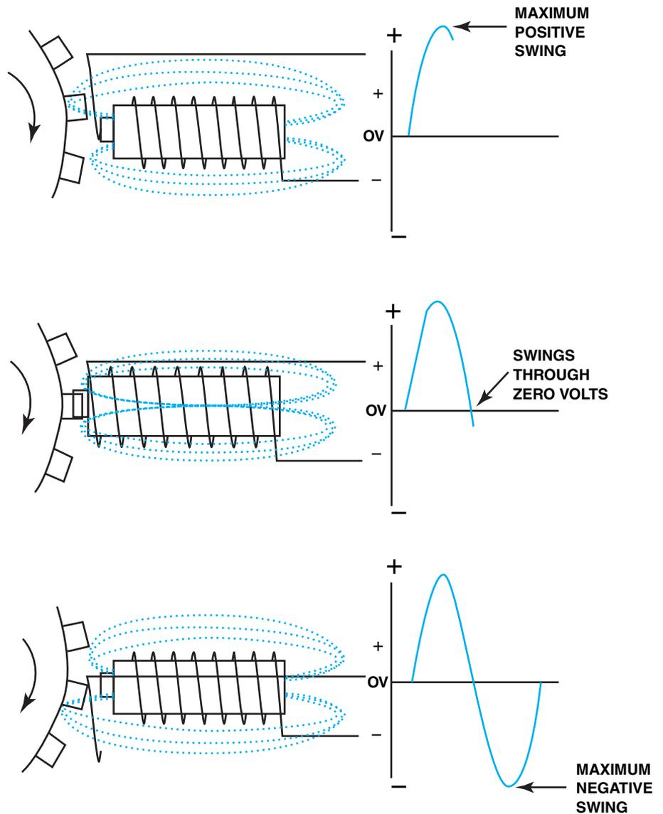
**FIGURE 16-9** A magnetic sensor uses a permanent magnet surrounded by a coil of wire. The notches of the crankshaft (or camshaft) create a variable magnetic field strength around the coil. When a metallic section is close to the sensor, the magnetic field is stronger because metal is a better conductor of magnetic lines of force than air.
