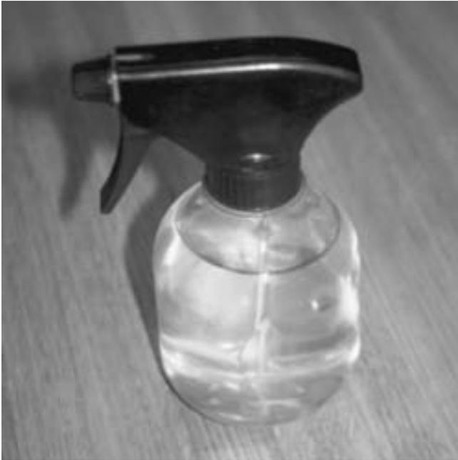
**FIGURE 16-36** A water spray bottle is an excellent diagnostic tool to help find an intermittent engine miss caused by a break in a secondary ignition circuit component.
