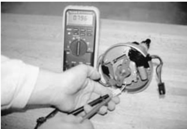
**FIGURE 16-23** Measuring the resistance of an HEI pickup coil using a digital multimeter set to the ohms position. The reading on the face of the meter is 0.796 KΩ or 796 ohms right in the middle of the 500 to 1500 ohm specifications.
