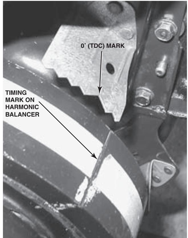
**FIGURE 16-37** Typical timing marks. The degree numbers are on the stationary plate and the notch is on the harmonic balancer.
