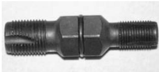
**FIGURE 16-33** A spark plug thread chaser is a low-cost tool that hopefully will not be used often, but is necessary to use to clean the threads before new spark plugs are installed.
