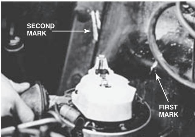
**FIGURE 16-40** The first mark indicates the direction the rotor is pointing when the distributor is in the engine. The second mark indicates where the rotor is pointing just as it is pulled from the engine.
