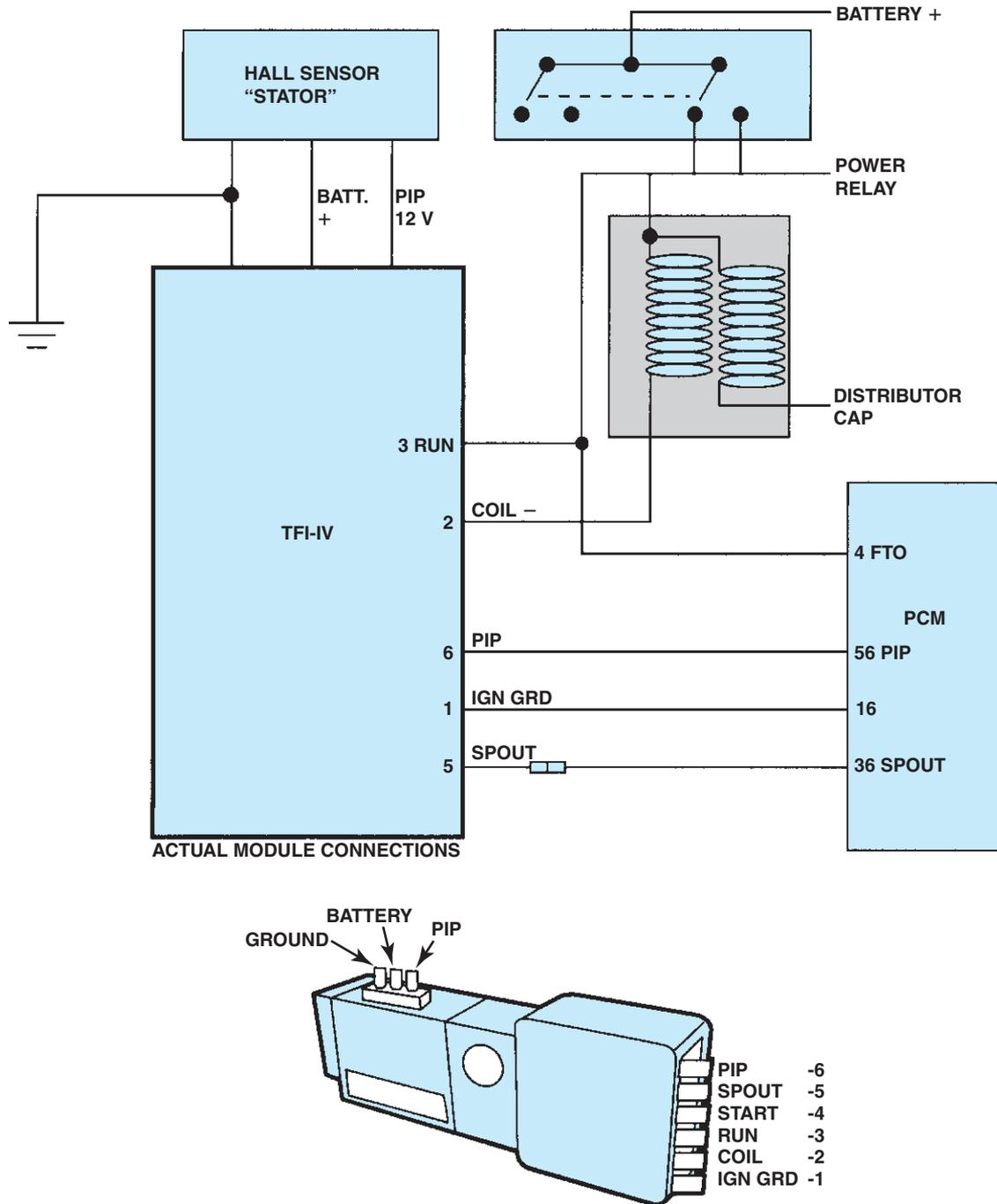
**FIGURE 16-15** Schematic of a Ford TFI-IV ignition system. The SPOUT connector is unplugged when ignition timing is being set.
