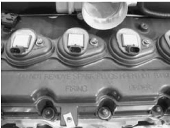
**FIGURE 16-21** Individual coils with modules shown on the General Motors 4.2L inline 6-cylinder light truck engine. Note the aluminum cooling fins (heat sink) on top of each assembly.
