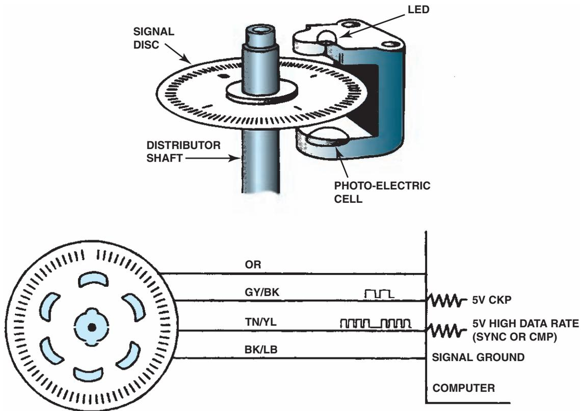
**FIGURE 16-10** The small holes (slots) in the signal disc create a high-data rate used for ignition timing. The larger slots represent crankshaft position top dead center for each of the cylinders on a V-6 engine.
