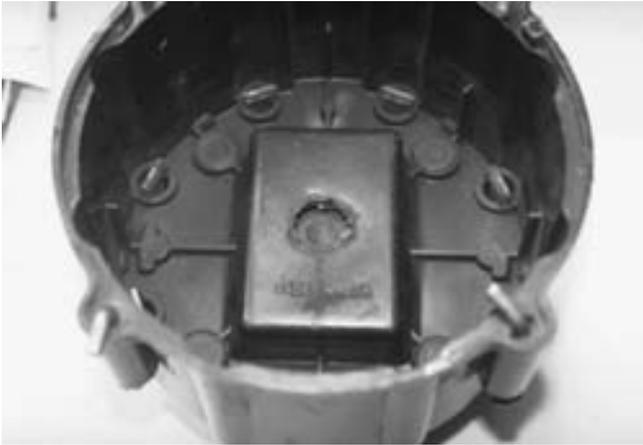
**FIGURE 16-27** This distributor cap came off a GM V-8 engine that was starting and running okay. The only problem seemed to be a “snapping” noise heard in the distributor.
