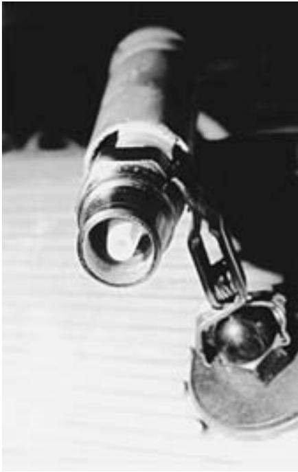
**FIGURE 16-22** Using a spark tester on an engine with direct-fire (distributorless) ignition. The spark tester is grounded to the rocker cover stud. This is the recommended type of spark tester, with the center electrode recessed into the center insulator.
