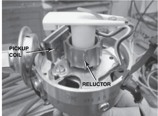
**FIGURE 16-17** A Chrysler electronic ignition distributor. This unit is equipped with a vacuum advance mechanism that advances the ignition timing under light engine load conditions.
