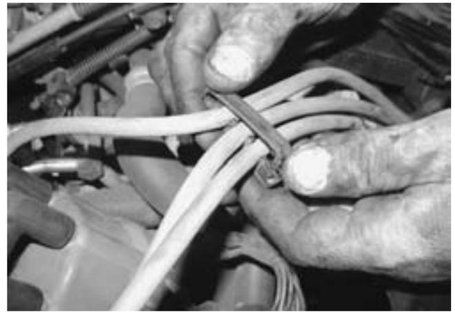
**FIGURE 16-25** Always take the time to install spark plug wires back into the original holding brackets (wiring combs).
