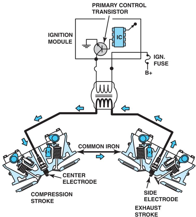
**FIGURE 16-18** A waste-spark system fires one cylinder while its piston is on the compression stroke and into paired or companion cylinders while it is on the exhaust stroke. In a typical engine, it requires only about 2 to 3 kV to fire the cylinder on the exhaust strokes. The remaining coil energy is available to fire the spark plug under compression (typically about 8 to 12 kV).
