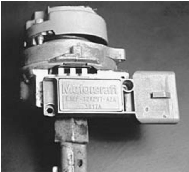
**FIGURE 16-16** Thick-film-integrated type of Ford EI. Note how the module plugs into the Hall-effect switch inside the distributor. Heat-conductive silicone grease should be used between the module and the distributor mounting pad to help keep the electronic circuits inside the module cool.
