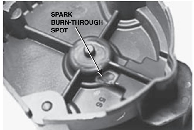
**FIGURE 16-26** Note where the high voltage spark jumped through the plastic rotor to arc into the distributor shaft. Always check for a defective spark plug(s) whenever a defective distributor cap or rotor is discovered. If a spark cannot jump to a spark plug, then it tries to find a ground path wherever it can.
