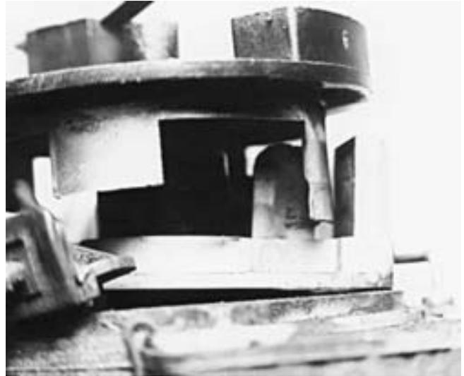
**FIGURE 16-8** Shutter blade of a rotor as it passes between the sensing silicon chip and the permanent magnet.
