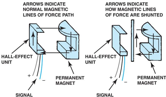
**FIGURE 16-7** Hall-effect switches use metallic shutters to shunt magnetic lines of force away from a silicon chip and related circuits. All Hall-effect switches produce a square wave output for every accurate triggering.
