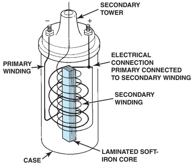
**FIGURE 16-1** Internal construction of an oil-cooled ignition coil. Notice that the primary winding is electrically connected to the secondary winding. The polarity (positive or negative) of a coil is determined by the direction in which the coil is wound.
