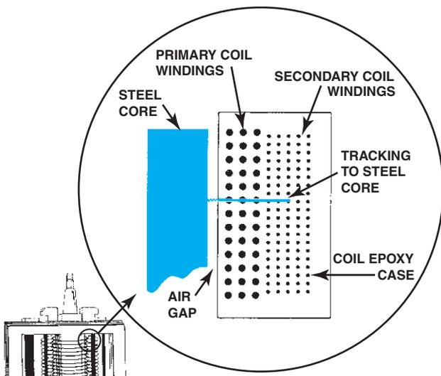
**FIGURE 16-24** A track inside an ignition coil is not a short, but rather a low-resistance path or hole that has been burned through from the secondary wiring to the steel core.
