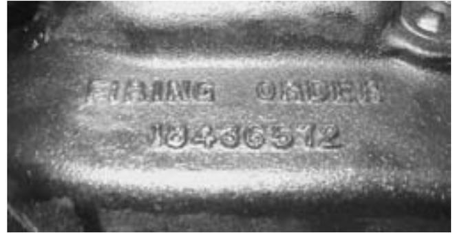
**FIGURE 16-29** The firing order is cast or stamped on the intake manifold on most engines that have a distributor ignition.
