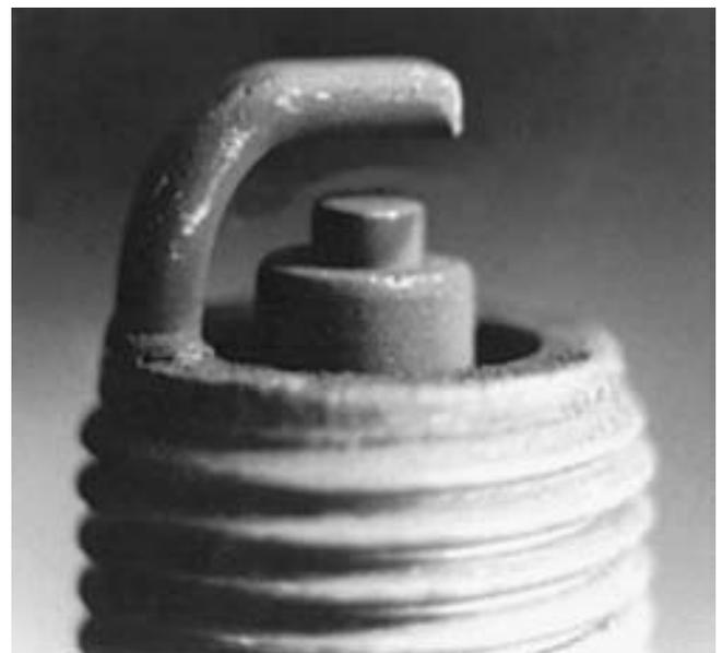
**FIGURE 16-35** New spark plug that was fouled by a too-rich air–fuel mixture. The engine from which this spark plug came had a defective (stuck partially open) injector on this one cylinder only.
