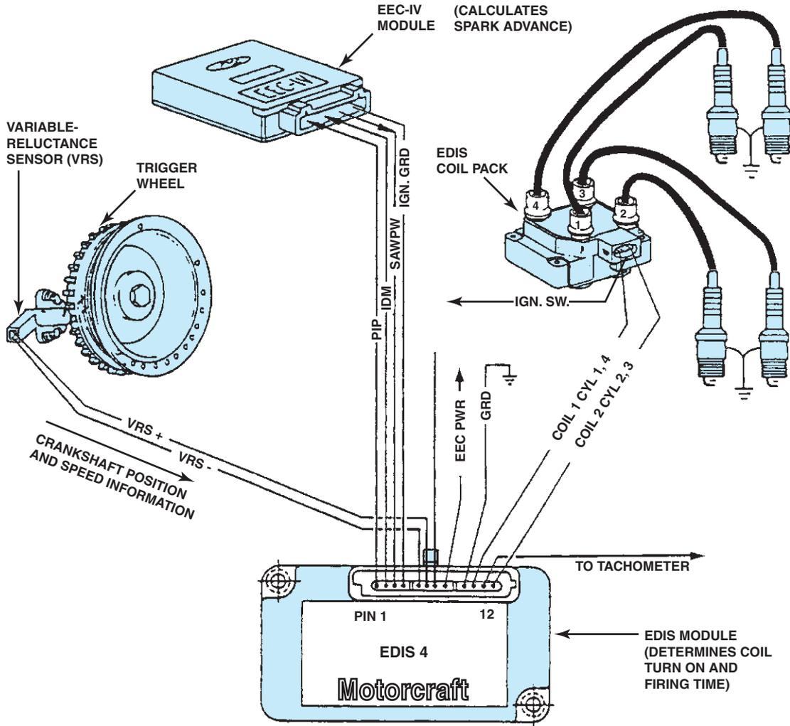
**FIGURE 16-19** Typical Ford EDIS 4-cylinder ignition system. The crankshaft sensor, called a variable-reluctance sensor (VRS), sends crankshaft position and speed information to the EDIS module. A modified signal is sent to the computer as a profile ignition pickup (PIP) signal. The PIP is used by the computer to calculate ignition timing, and the computer sends a signal back to the EDIS module as to when to fire the spark plug. This return signal is called the spark angle word (SAW) signal.
