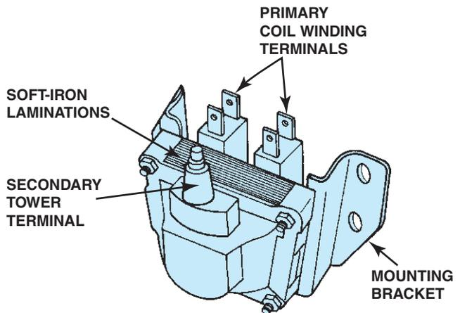
**FIGURE 16-2** Typical air-cooled epoxy-filled E coil.
