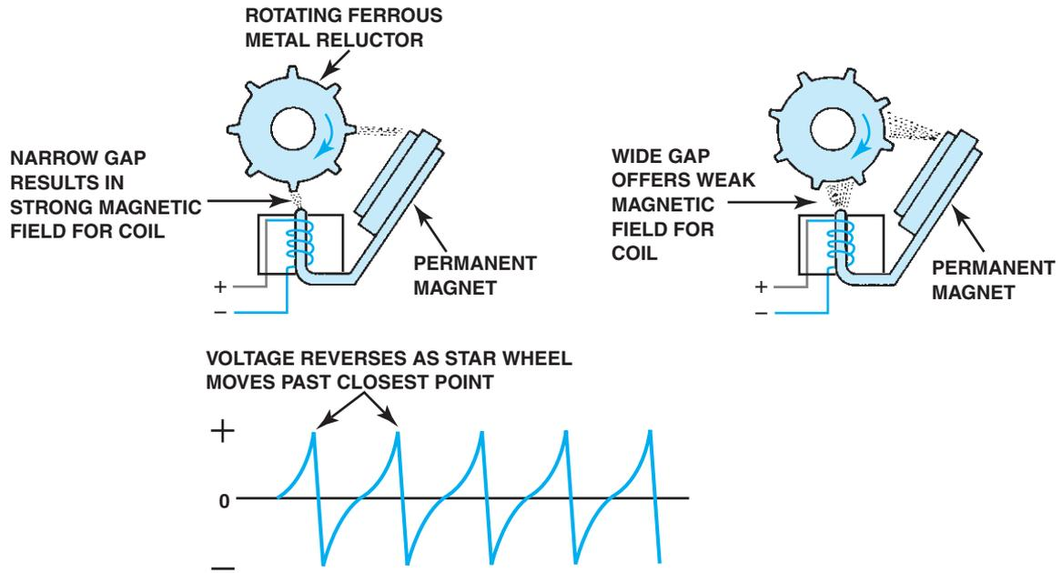
**FIGURE 16-5** Operation of a typical pulse generator (pickup coil). At the bottom is a line drawing of a typical scope pattern of the output voltage of a pickup coil. The module receives this voltage from the pickup coil and opens the ground circuit to the ignition coil when the voltage starts down from its peak (just as the reluctor teeth start moving away from the pickup coil).
