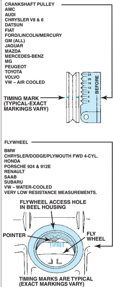
**FIGURE 16-38** Cylinder 1 and timing mark location guide.
