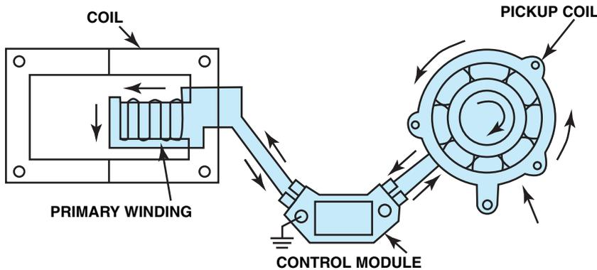
**FIGURE 16-6** The varying voltage signal from the pickup coil triggers the ignition module. The ignition module grounds and ungrounds the primary winding of the ignition coil, creating a high-voltage spark.
