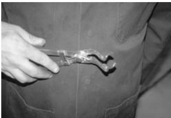
**FIGURE 16-31** Spark plug wire boot pliers are a handy addition to any toolbox.
