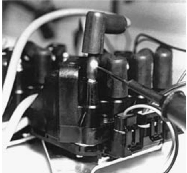
**FIGURE 16-28** Using a vacuum hose and a grounded test light to ground one cylinder at a time on a DIS. This works on all types of ignition systems and provides a method for grounding out one cylinder at a time without fear of damaging any component.
