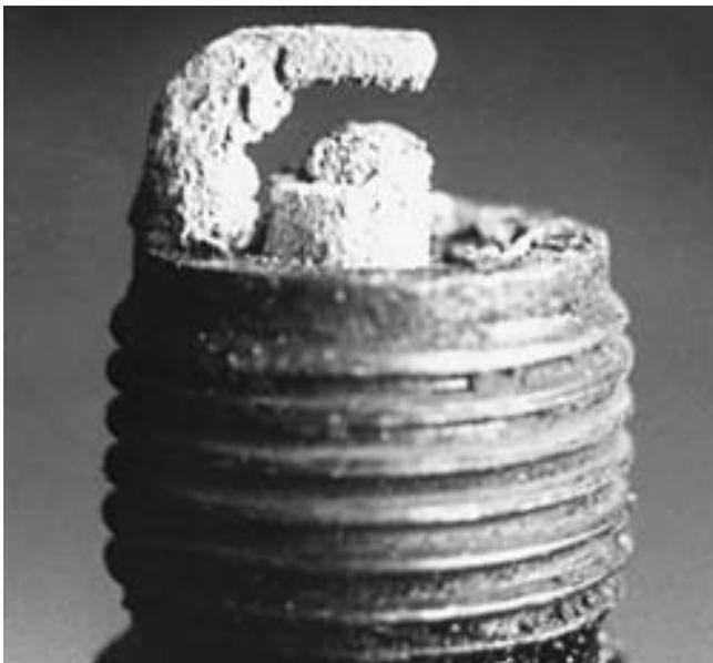
**FIGURE 16-34** Typical worn spark plug. Notice the rounded center electrode. The deposits indicate a possible oil usage problem.
