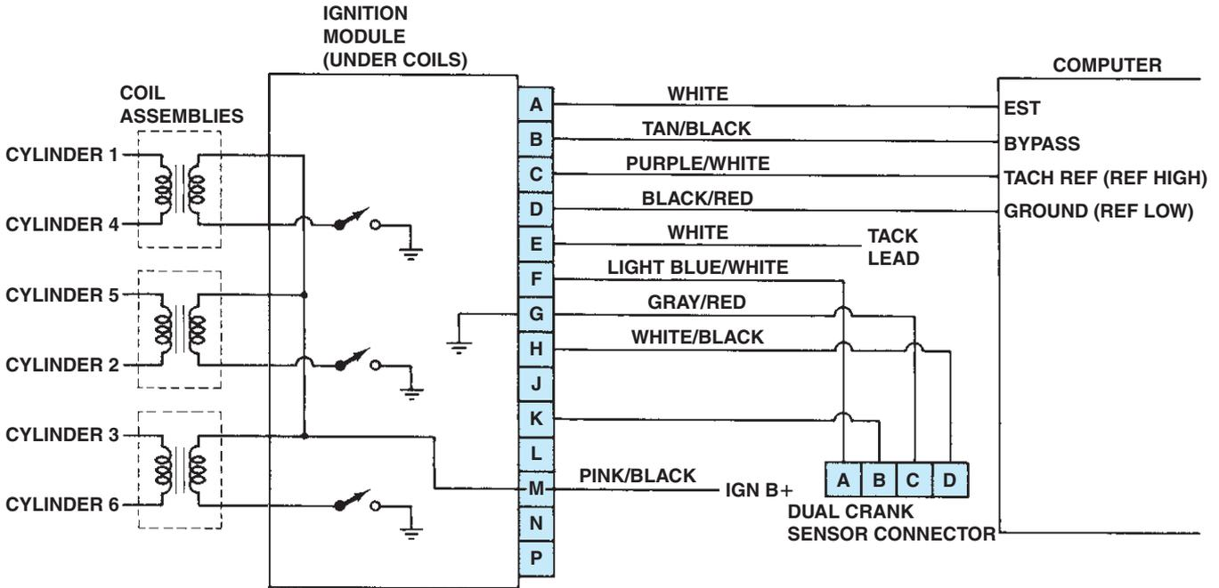
**FIGURE 16-20** Typical wiring diagram of a V-6 distributorless (direct fire) ignition system.
