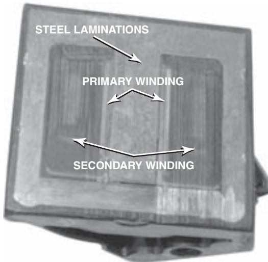
**FIGURE 16-3** Cutaway of a General Motors Type II distributorless ignition coil. Note that the primary windings are inside of the secondary windings.
