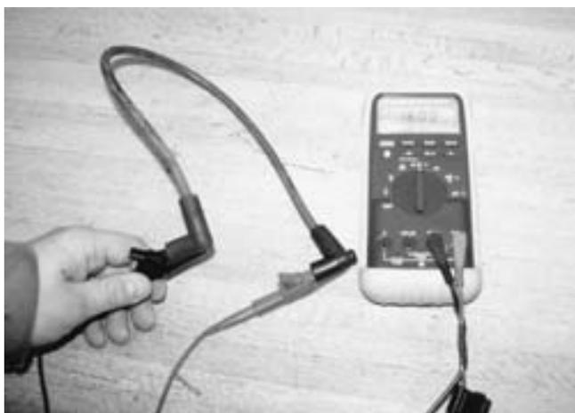
**FIGURE 16-30** Measuring the resistance of a spark plug wire with a multimeter set to the ohms position. The reading of 16.03 k $\Omega$  (16,030 ohms) is okay because the wire is about 2 ft long. Maximum allowable resistance for a spark plug wire this long would be 20 k $\Omega$  (20,000 ohms).
