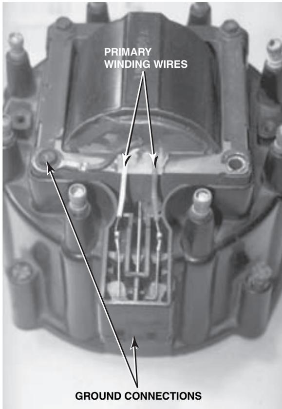
**FIGURE 16-13** A typical General Motors HEI coil installed in the distributor cap. When the coil or distributor cap is replaced, check that the ground clip is transferred from the old distributor cap to the new. Without proper grounding, coil damage is likely. There are two designs of HEI coils. One uses red and white wire and the other design, which has reversed polarity, uses red and yellow wire for the primary coil.
