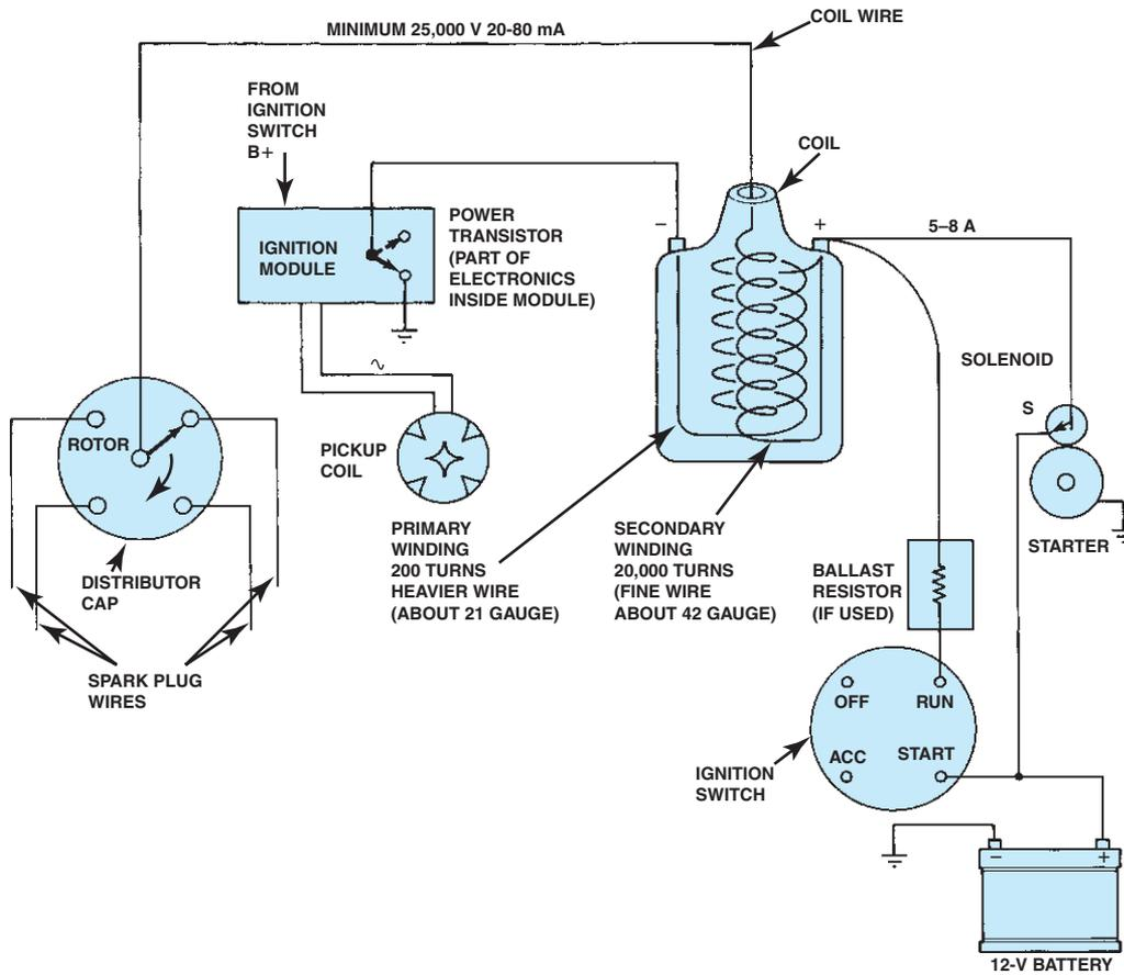
**FIGURE 16-4** Typical primary and secondary electronic ignition using a ballast resistor and a distributor. To protect the ignition coil from overheating at lower engine speeds, many electronic ignitions do not use a ballast resistor, but use electronic circuits within the module.
