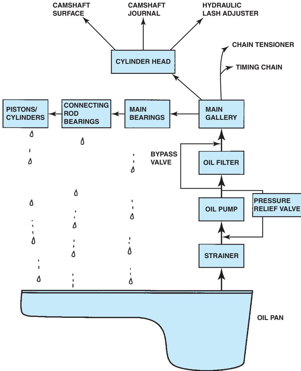
**FIGURE 14-26** Oil flow through an engine starts at the oil pump pickup and eventually ends up with the oil dropping back into the oil pan.
