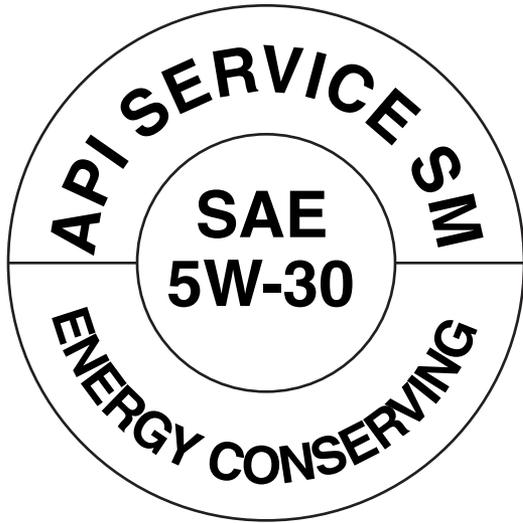
**FIGURE 14-5** API doughnut for a SAE 5W-30, SM engine oil. When compared to a reference oil, the “energy conserving” designation indicates a 1.1% better fuel economy for SAE 10W-30 oils and 0.5% better fuel economy for SAE 5W-30 oils.
