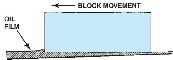
**FIGURE 14-2** Wedge-shaped oil film developed below a moving block.
