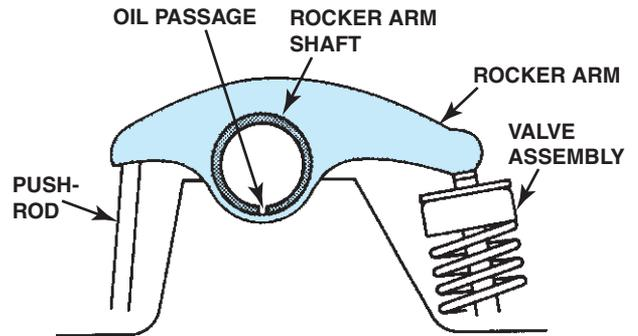
**FIGURE 14-28** The rocker arm pivot is lubricated through the oil passage in the bottom of the rocker shaft. Other rocker arm styles are usually lubricated through a hollow pushrod.
