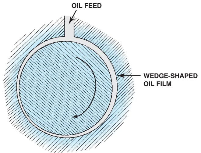
**FIGURE 14-3** Wedge-shaped oil film curved around a bearing journal.
