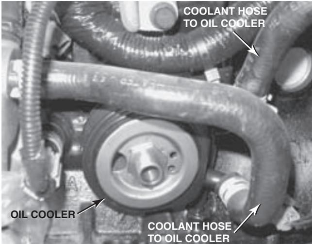
**FIGURE 14-31** Typical engine oil cooler. Engine oil is cooled by passing coolant from the radiator through the auxiliary housing. The oil filter screws to the cooler.
