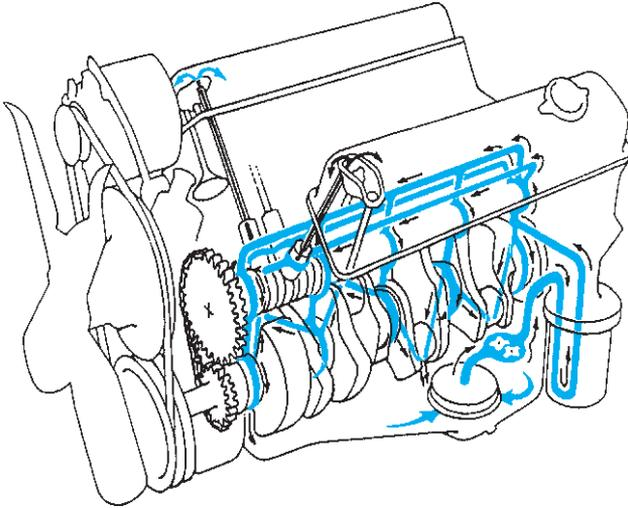
**FIGURE 14-4** Typical V-8 engine lubrication system. Oil is stored in the oil pan (sump), drawn into the oil pump, and moves through the oil filter and on through the oil passages (oil galleries).
