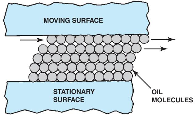
**FIGURE 14-1** Oil molecules cling to metal surfaces but easily slide against each other.
