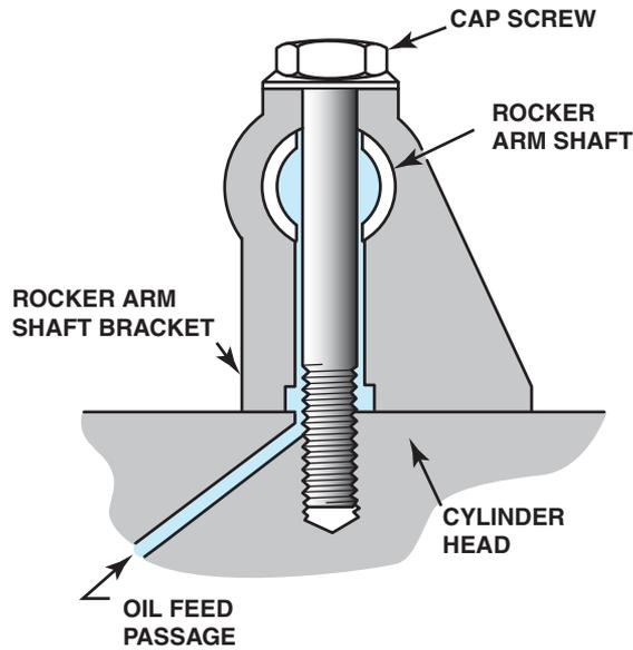
**FIGURE 14-27** Clearance around the rocker shaft bracket cap screw makes a passage for oil to get into the rocker shaft. (Courtesy of Dana Corporation)
