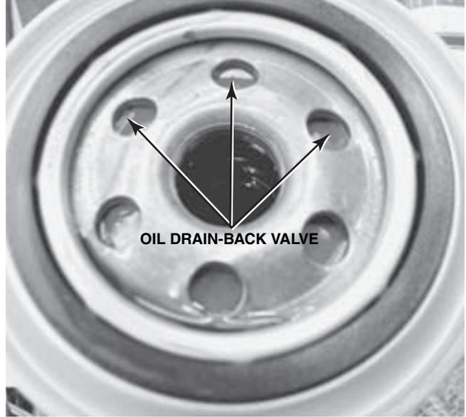
**FIGURE 14-12** A rubber diaphragm acts as an antidrainback valve to keep the oil in the filter when the engine is stopped and the oil pressure drops to zero.
