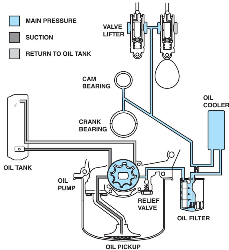
**FIGURE 14-30** A dry sump system that is used on the Chevrolet Corvette.
