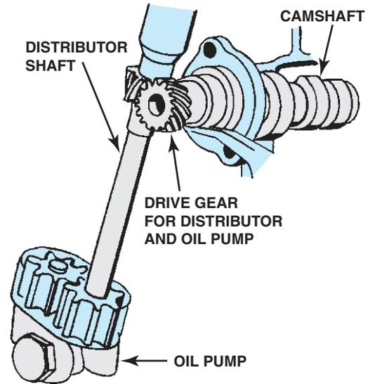
**FIGURE 14-15** An oil pump driven by the camshaft.
