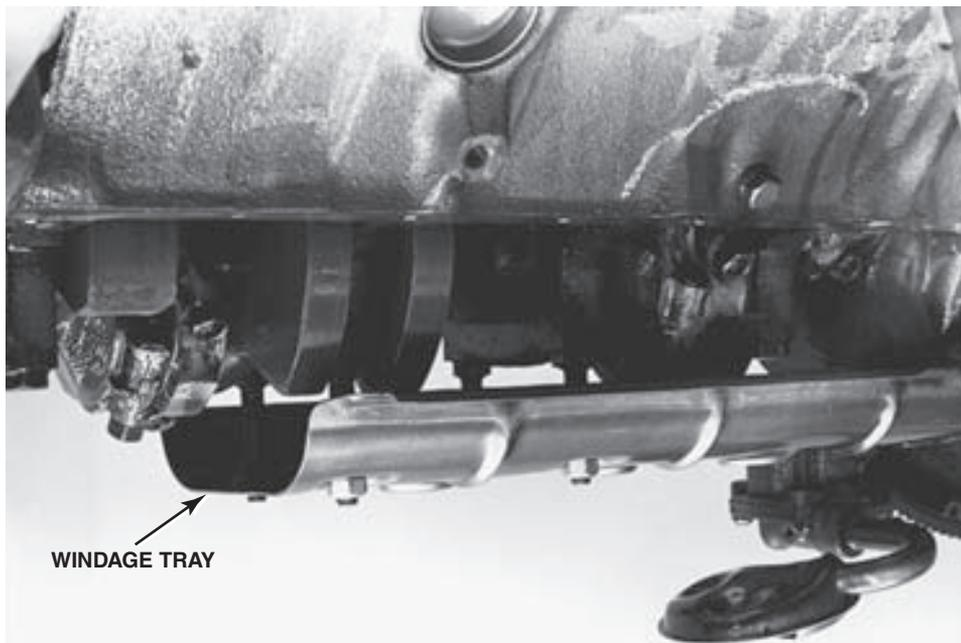
**FIGURE 14-29** Windage tray attached between the crankshaft and the oil pan.
