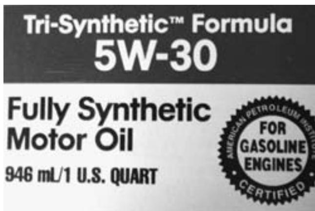
**FIGURE 14-8** Container of oil with the ILSAC starburst symbol on the front. The tri-synthetic label indicates that it contains Group IV (POA) as well as Group V (diesters) to swell seals, and some Group III (hydrocracked oil).
