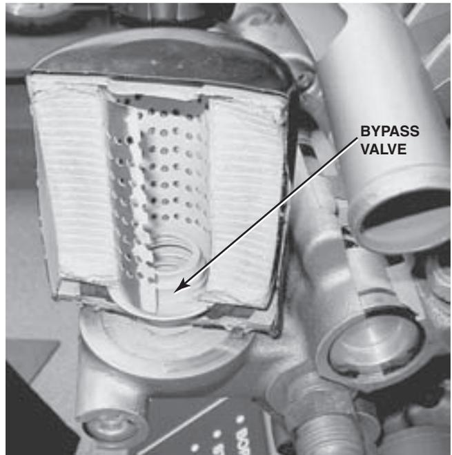
**FIGURE 14-13** A cutaway of an oil filter showing the location of a typical bypass valve. When the oil filter becomes clogged, the bypass valve opens, allowing the engine to receive oil even though it is not filtered.
