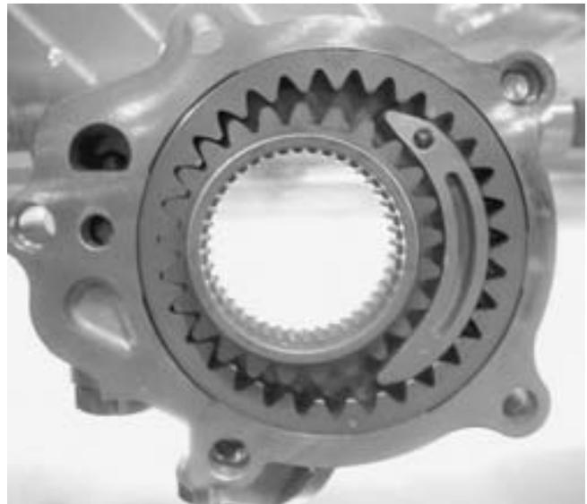
**FIGURE 14-16** A typical oil pump mounted in the front cover of the engine that is driven by the crankshaft.
