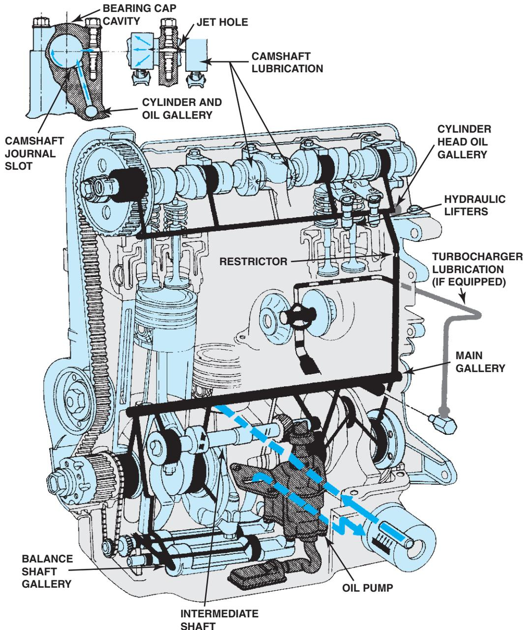
**FIGURE 14-21** An intermediate shaft drives the oil pump on this overhead camshaft engine. Note the main gallery and other drilled passages in the block and cylinder head.
