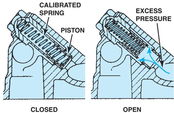
**FIGURE 14-19** Oil pressure relief valves are spring loaded. The stronger the spring tension, the higher the oil pressure.
