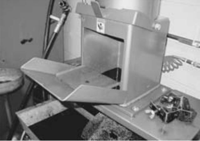
**FIGURE 14-14** A typical oil filter crusher. The hydraulic ram forces out most of the oil from the filter. The oil is trapped underneath the crusher and is recycled.
