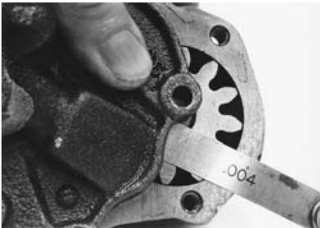
**FIGURE 14-25** Measuring the gear-to-cover clearance of an oil pump.
