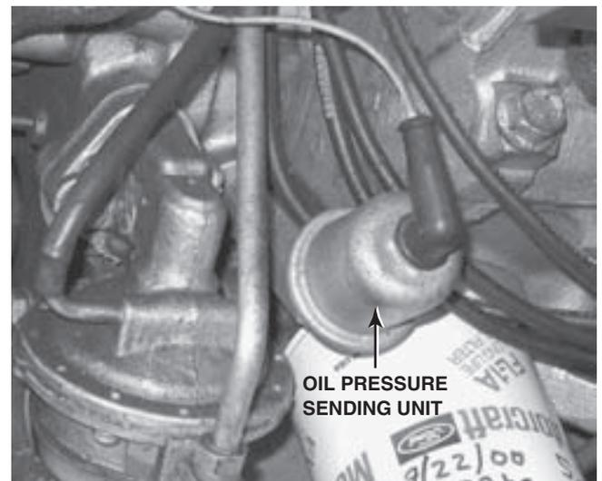
**FIGURE 14-33** A typical oil pressure sending unit on a Ford V-8.
