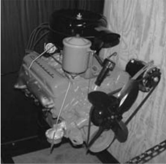
**FIGURE 14-11** This early Chevrolet V-8 has what was an optional oil filter, which is connected to an oil gallery and return oil flows into the oil pan.
