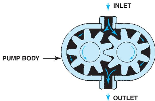
**FIGURE 14-18** In a gear-type oil pump, the oil flows through the pump around the outside of each gear. This is an example of a positive displacement pump, wherein everything entering the pump must leave the pump.
