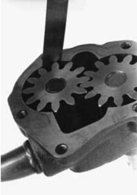
**FIGURE 14-24** Gear-type oil pump being checked for tooth clearance in the housing.
