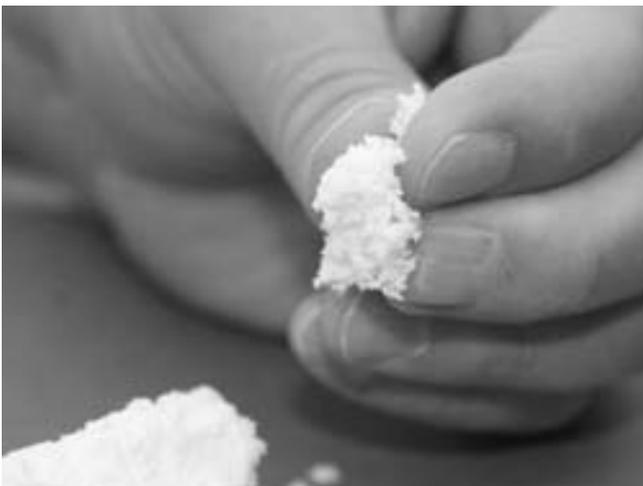
**FIGURE 14-7** VI improver is a polymer and feels like finely ground foam rubber. When dissolved in the oil, it expands when hot to keep the oil from thinning.
