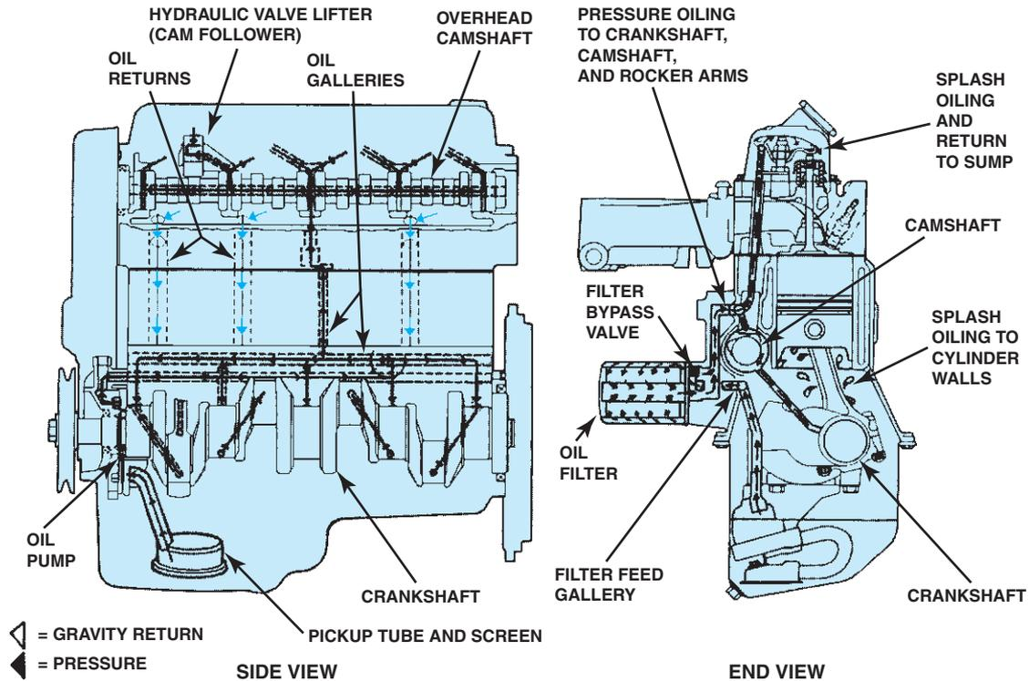
**FIGURE 14-20** A typical engine design that uses both pressure and splash lubrication. Oil travels under pressure through the galleries (passages) to reach the top of the engine. Other parts are lubricated as the oil flows back down into the oil pan or is splashed onto parts.
