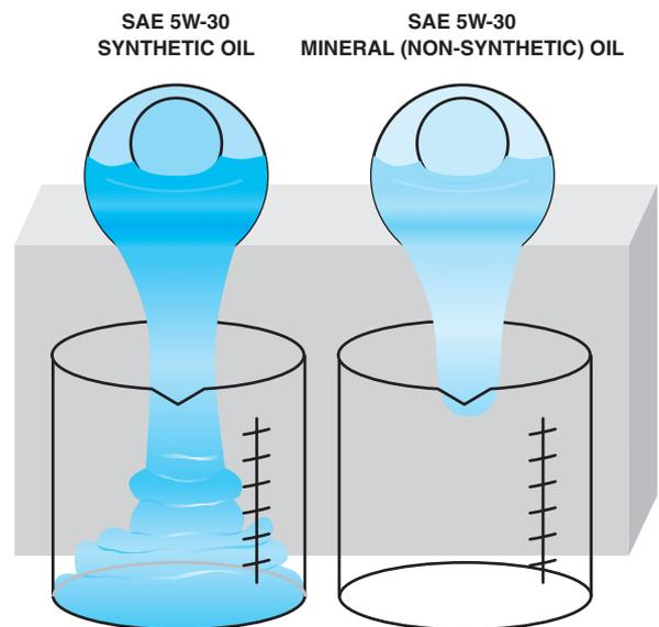
**FIGURE 14-9** Both oils have been cooled to  $-20^{\circ}\text{F}$  ( $-29^{\circ}\text{C}$ ). Notice that the synthetic oil on the left flows more freely than the mineral oil on the right even though they are both SAE 5W-30.
