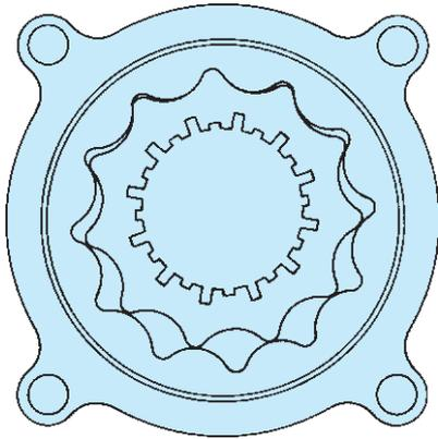
**FIGURE 14-17** Gerotor-type oil pump driven by the crankshaft.
