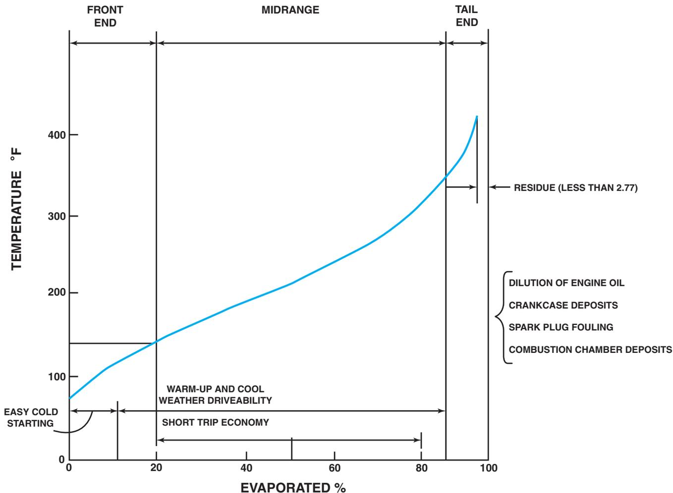
**FIGURE 11-4** A typical distillation curve. Heavier molecules evaporate at higher temperatures and contain more heat energy for power, whereas the lighter molecules evaporate easier for starting.
