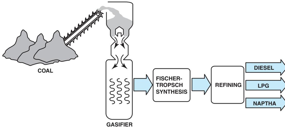
**FIGURE 11-30** A typical coal-to-liquid plant.
