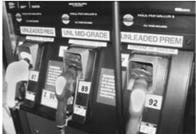
**FIGURE 11-7** A typical fuel pump showing regular (87 octane), midgrade (89 octane), and premium (92 octane). These ratings can vary with brand as well as in different parts of the country, especially in high-altitude areas where the ratings are lower.
