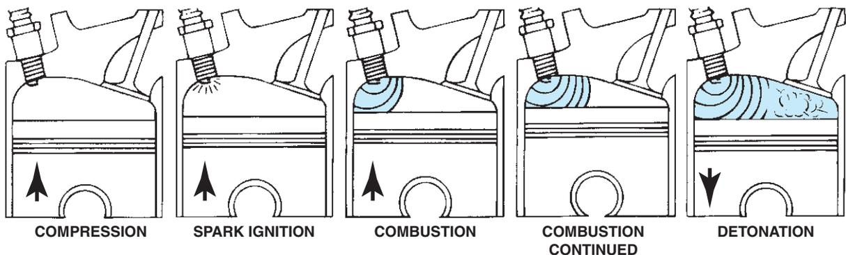
**FIGURE 11-6** Detonation is a secondary ignition of the air–fuel mixture. It is also called spark knock or pinging.
