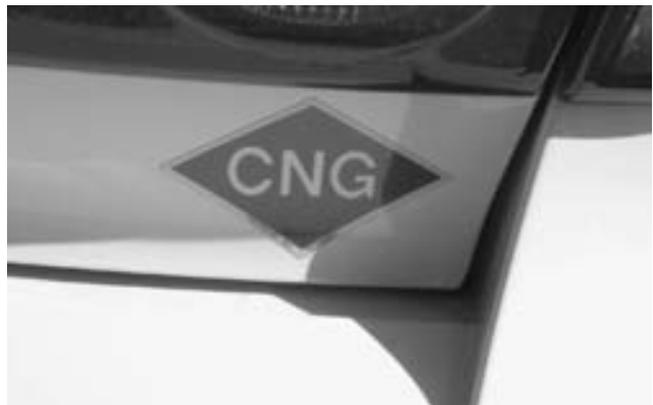
**FIGURE 11-24** The blue sticker on the rear of this vehicle indicates that it is designed to use compressed natural gas.
