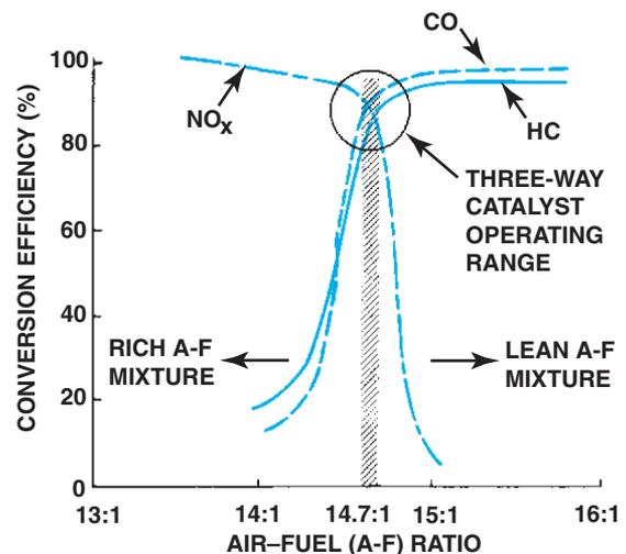
**FIGURE 11-11** With a three-way catalytic converter, emission control is most efficient with an air-fuel ratio between 14.65:1 and 14.75:1.
