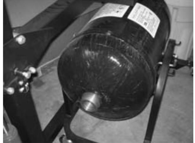
**FIGURE 11-26** A CNG storage tank from a Honda Civic GX shown with the fixture used to support it while it is being removed or installed in the vehicle. Honda specifies that three technicians be used to remove or install the tank through the rear door of the vehicle due to the size and weight of the tank.
