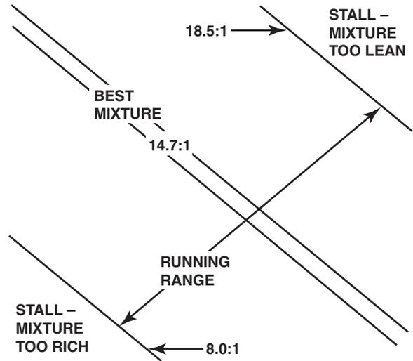
**FIGURE 11-10** An engine will not run if the air-fuel mixture is either too rich or too lean.
