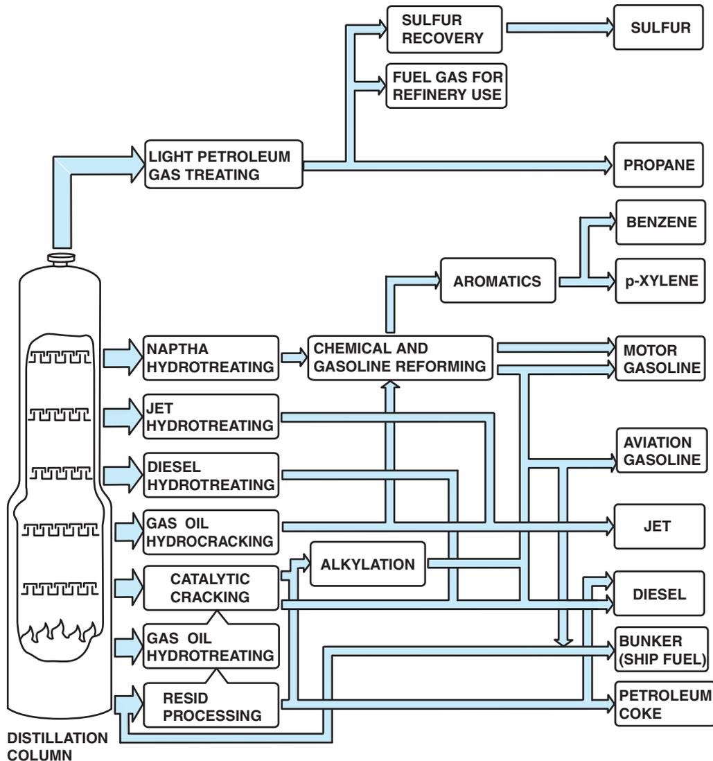
**FIGURE 11-1** The crude oil refining process showing most of the major steps and processes.
