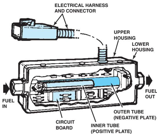
**FIGURE 11-19** A cutaway view of a typical variable fuel sensor.
