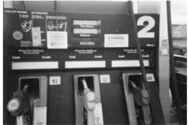
**FIGURE 11-12** Photo of gasoline pump taken in a high-altitude area. Note the lower-than-normal octane ratings. The “ethanol” sticker reads that all grades contain 10% ethanol from November 1 through February 28 each year to help reduce CO exhaust emissions.
