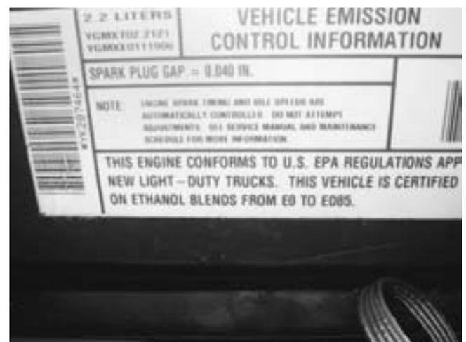
**FIGURE 11-17** A vehicle emission control information (VECI) sticker on a flexible fuel vehicle indicating the percentage of ethanol with which it is able to operate.
