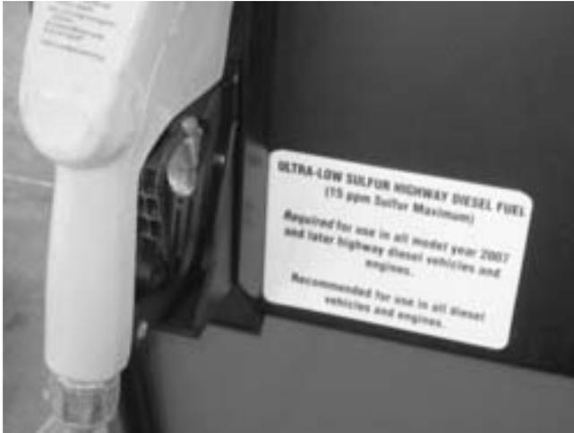
**FIGURE 11-28** A pump decal indicating that the diesel fuel is ultra-low-sulfur diesel (ULSD) and must be used in 2007 and newer diesel vehicles.
