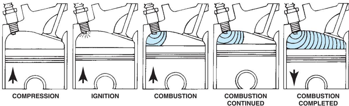
**FIGURE 11-5** Normal combustion is a smooth, controlled burning of the air–fuel mixture.
