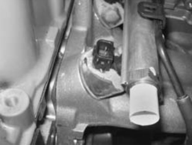
**FIGURE 11-25** The fuel injectors used on this Honda Civic GX CNG engine are designed to flow gaseous fuel instead of liquid fuel and cannot be interchanged with any other type of injector.
