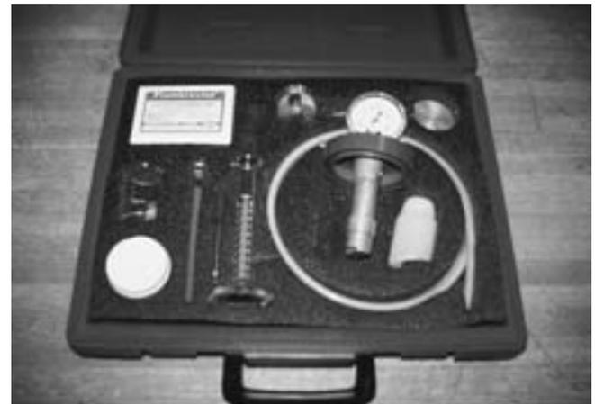
**FIGURE 11-3** A gasoline testing kit. Included is an insulated container where water at 100°F is used to heat a container holding a small sample of gasoline. The reading on the pressure gauge is the Reid vapor pressure (RVP).
