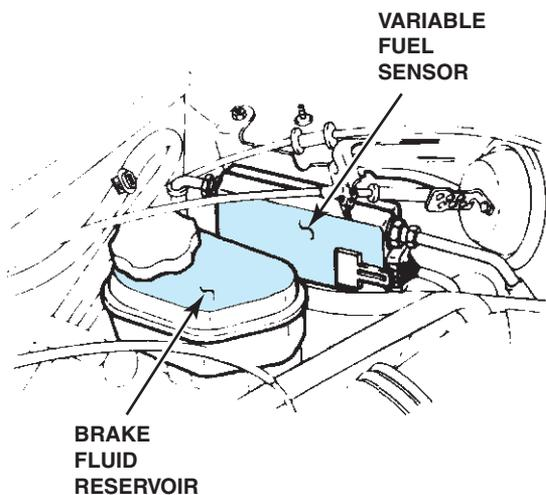
**FIGURE 11-18** The location of the variable fuel sensor can vary, depending on the make and model of vehicle, but it is always in the fuel line between the fuel tank and the fuel injectors.
