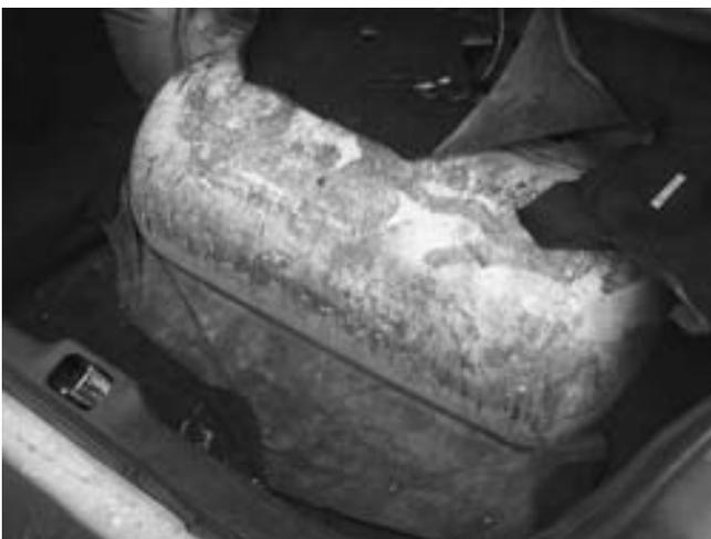
**FIGURE 11-23** Propane fuel storage tank in the trunk of a Ford taxi.
