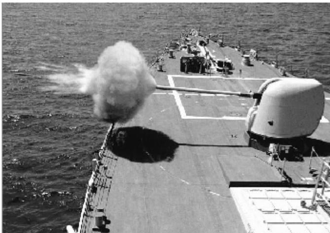
**Figure D-2. USN MK45 Lightweight Gun System**
