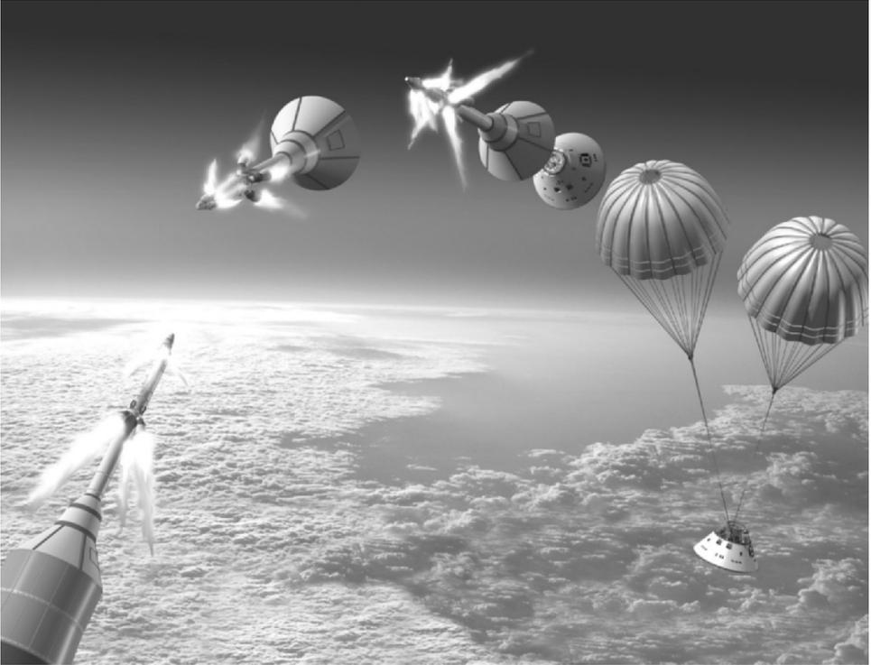
**Figure 7.3** Launch abort system. Courtesy NASA.
