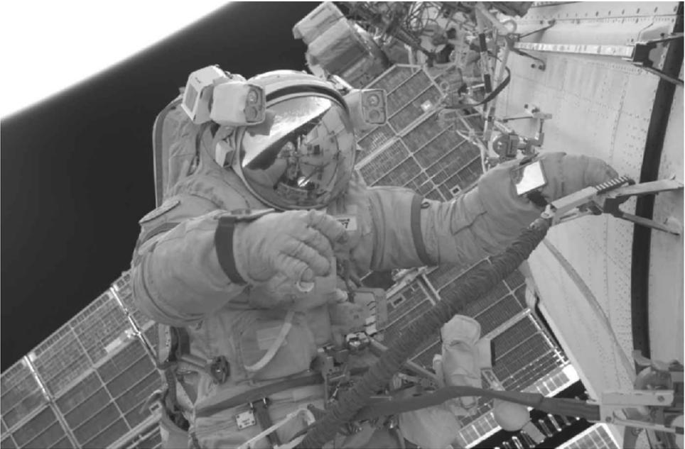
**Figure 7.12** Orlan space suit. Courtesy NASA (*see colour section*).
