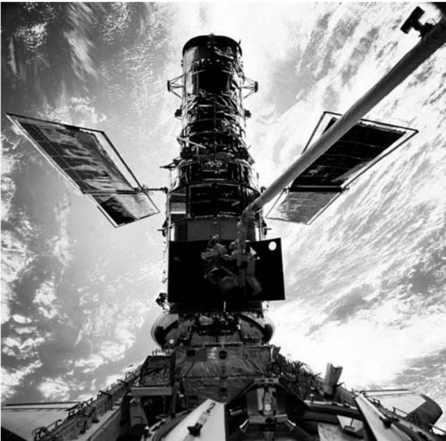
**Fig. 2.** Exchange of three Rate Sensor Units (RSUs) on HST, or HST SM-3A, December 1999 (source: NASA Picture).
