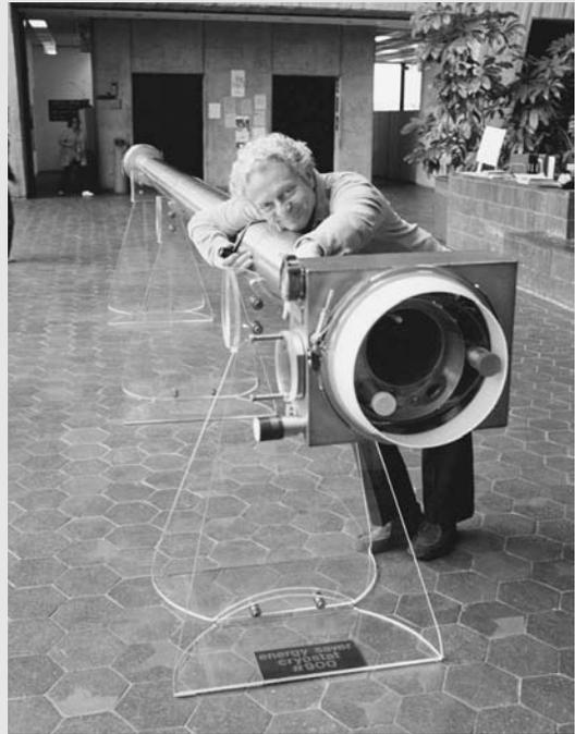
*Leon Lederman shows his playful side while posing with a Fermilab exhibit of a cryostat, a device necessary to maintain very low temperatures necessary for the superconducting electromagnets used to create the fields that control paths of subatomic particles in accelerators. (Fermilab Visual Media Services)*
