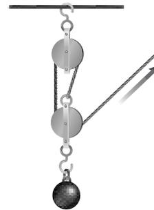
5. The pulley system in the illustration above uses several pulleys to increase the mechanical advantage. What is the mechanical advantage of this system?
