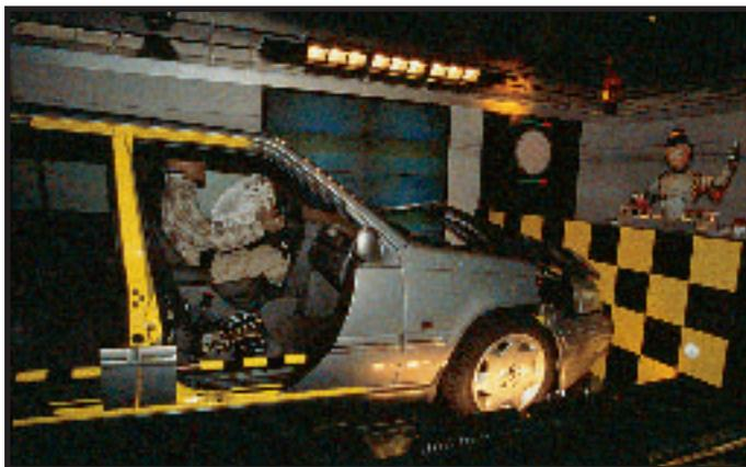
**A test measures the speed at which an air bag deploys.**
