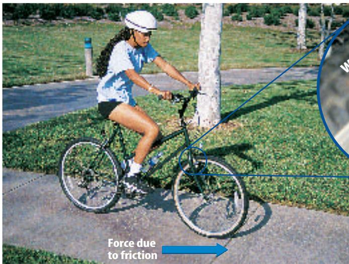
**Figure 6** A bicycle uses sliding friction and rolling friction.
