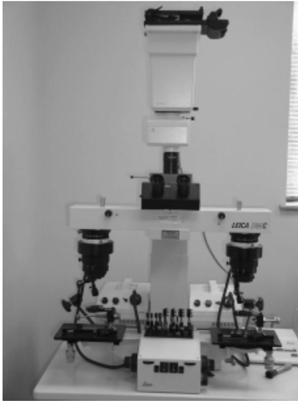
FIGURE S.14 Stereomicroscope used in ballistics examination.
