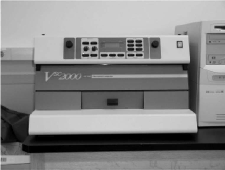
**FIGURE V.2** Video spectral comparator.
