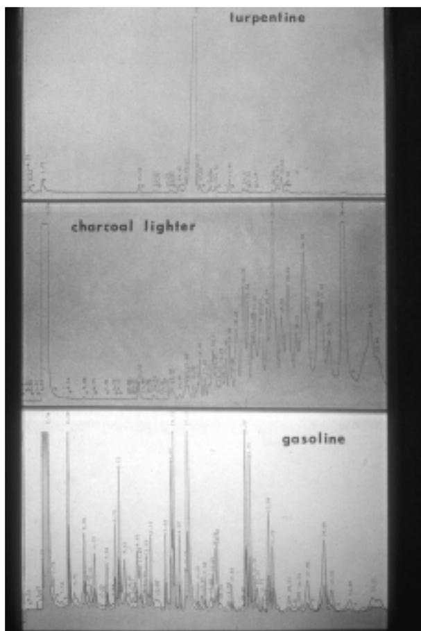
**FIGURE C.14** Gas chromatograms of turpentine, charcoal lighter fluid, and gasoline. A special high-resolution column known as a capillary column was used. The mixture of hydrocarbon is separated into its components, with the peaks representing at least one different component.
