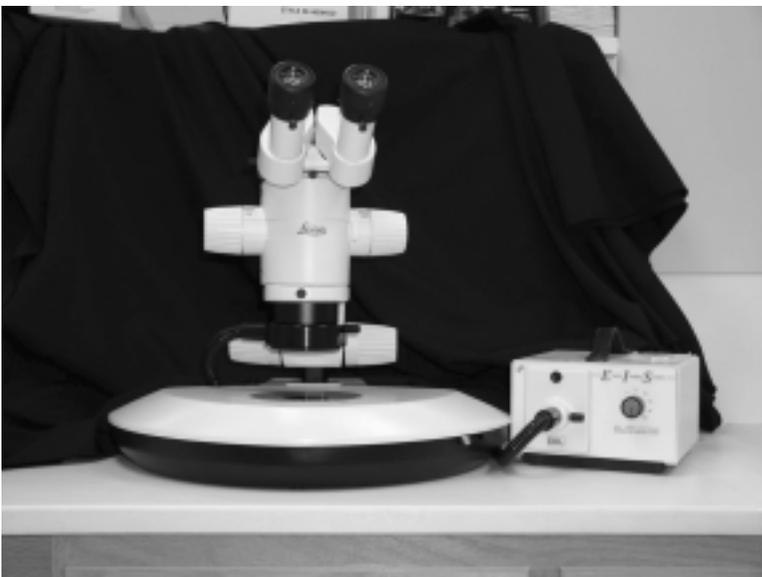
**FIGURE S.13B** Stereomicroscope used for the screening of trace evidence (fingernail scrapings, hairs, fibers, etc.).
