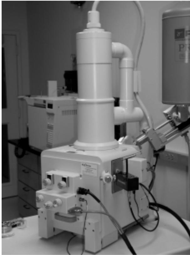
**FIGURE S.1** Scanning electron microscope.
