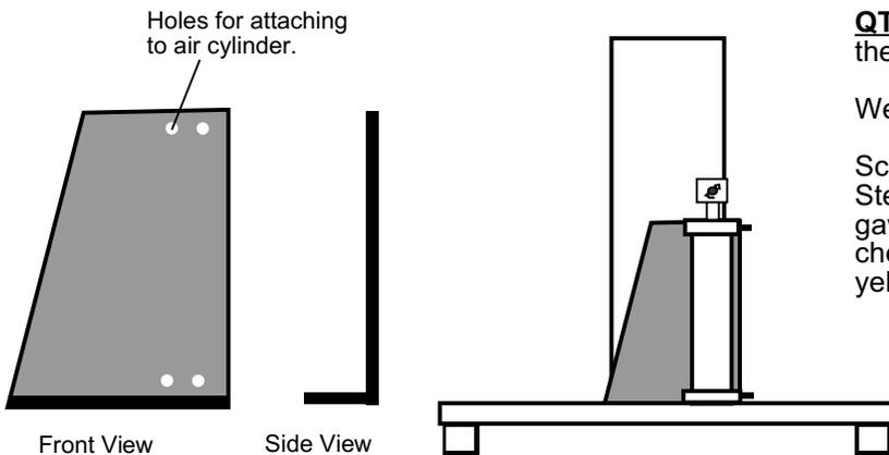
**QTY-1** This is side to base steel attachment for the air cylinder to hook on to.
