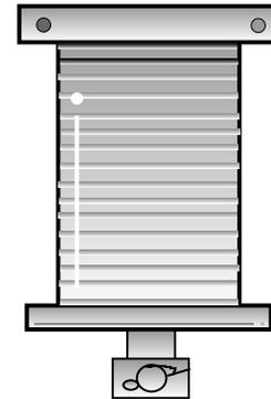
Polarity will depend on if the plunger pushes out or in. Build a small toy model first. It is best if you can build the solenoid to attract as in Figure B. Use #27 copper coated wire 66 lbs there of for larger motors and # 34 for a small toy motor, coil should weigh about 6 lbs. I do not know how many winds that is? Wind from left to right. Glue PVC bobbins with PVC glue that you can buy online or at any hardware stor. PVC sheets can be baought at any sign shop or sign supply company.
