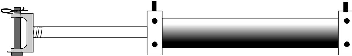
NOTE: If air cylinder stroke is more than or less than 8" you can have some problems, if it is more or less you will need to adjust the length of part #5 & #6 or you can simply adjust the length of part# 7.
