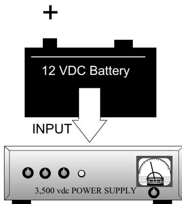
OUTPUT 3,500 VDC to 5,000 VDC
