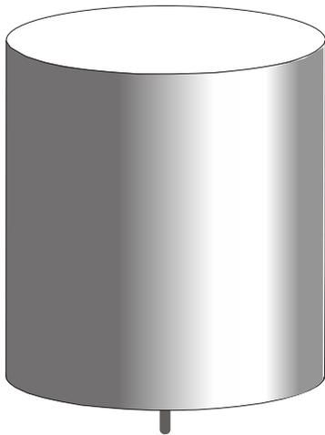
Inner Drum: Paint Can, 1 gal. 7 5/8" tall x 6 5/8" diameter.
