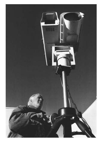
An electronics technician for the U.S. Border Patrol uses a crank to manually turn two surveillance cameras, a thermo imager, right, and a daytime camera, left. AP/WIDE WORLD PHOTOS.
