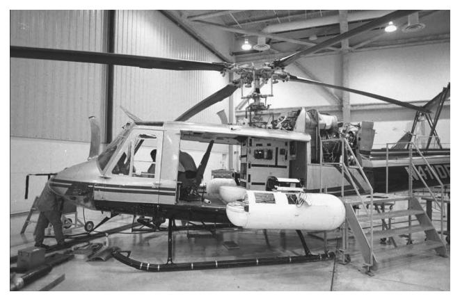
Nuclear Emergency Search Team members install radiation-sensing equipment into a helicopter at the NEST facility at Nellis Air Force Base in Nevada. AP/WIDE WORLD PHOTOS.
