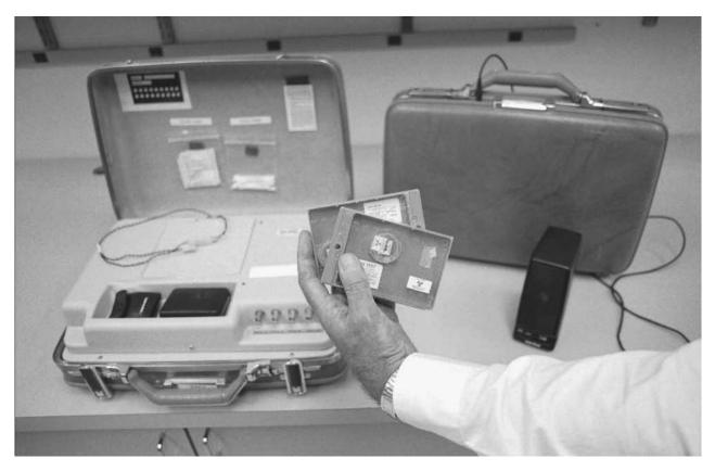
A Nuclear Emergency Search Team (NEST) member shows portable sensing equipment used to detect radioative sources. The briefcase design allows NEST members to carry the sensing device undetected in crowded environments. AP/WIDE WORLD PHOTOS.
