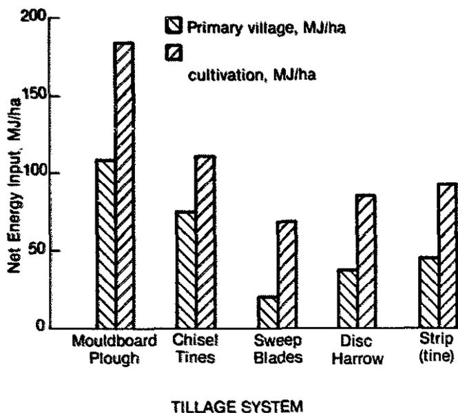
Fig.3 Tillage net energy inputs per ha under semi-arid conditions (Willcocks, T.J., 'Tillage of clod-forming sandy loam soils in the semi-arid climate of Botswana'. *Soil & Tillage Research* 7 (1980-81) pp.323-350 (Elsevier).
