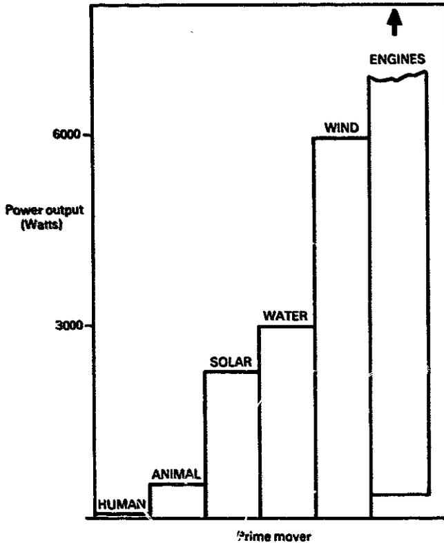
Fig.2 Available power output from various prime movers.
