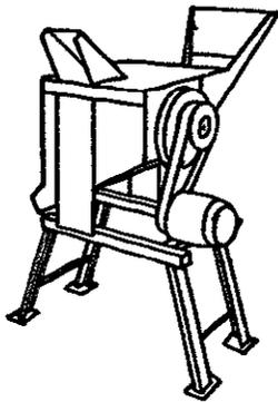
**CORN HUSKER SHELLER** This machine is fitted with an axial flow motor capable of husking and shelling up to 600kg of maize per hour. It has a pneumatic box-windrowing system and is driven by a 2hp electric motor or engine. (Illustrated).
