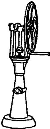
The provision of a single or pair of ungeared flywheels on these models permits pumping from very deep wells by one or more operators.
