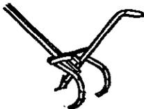
**VIKAS JR. CULTIVATOR** The Vikas Jr. is a simpler version of the R.N. Cultivator above. The width of the 3 tines is easily adjustable. A mouldboard plough, seeding attachments, and sweeps of various sizes can be supplied. The area covered by the Vikas Jr. is 1.2-1.6ha per day.
