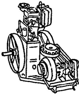
**VIJAY PUMPSETS** These consist of a vertical water cooled single-cylinder diesel engine from 5 to 10hp coupled either directly or by belt drive to a variety of centrifugal pumps — self priming, end-suction, split casing and volute types, shown right. Total head range from 6 to 26m with outputs from 135 to 36m<sup>3</sup>/h respectively. Electric motor driven options also available.
