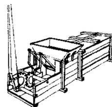
produces bales of approximately the same size but, as can be seen, the feed arrangement and the compression mechanism are different allowing for a more rapid formation of denser bales. There are similar slits in the sides through which the bale twine can be placed.
