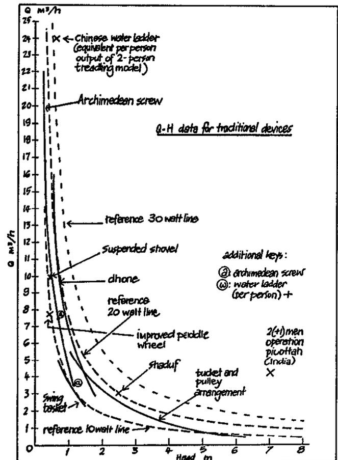
Fig.3 Discharge versus head performance: traditional human-powered pumps.
