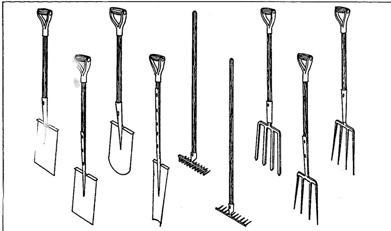
*From left: solid socket treaded spade; strapped treaded spade; open socket treaded round nose spade; strapped treaded drainage spade; shaped-tine rake; tang and ferrule broad-tine digging fork; strapped fork; solid socket digging fork.*
