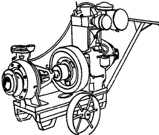
100mm (pump outlet diameter). Total head ranges from 9 to 18m with corresponding outputs from 144 to 40m<sup>3</sup>/h. Weight 168kg. Larger twin-cylinder model, DE-14 has approximately double the capacity.
