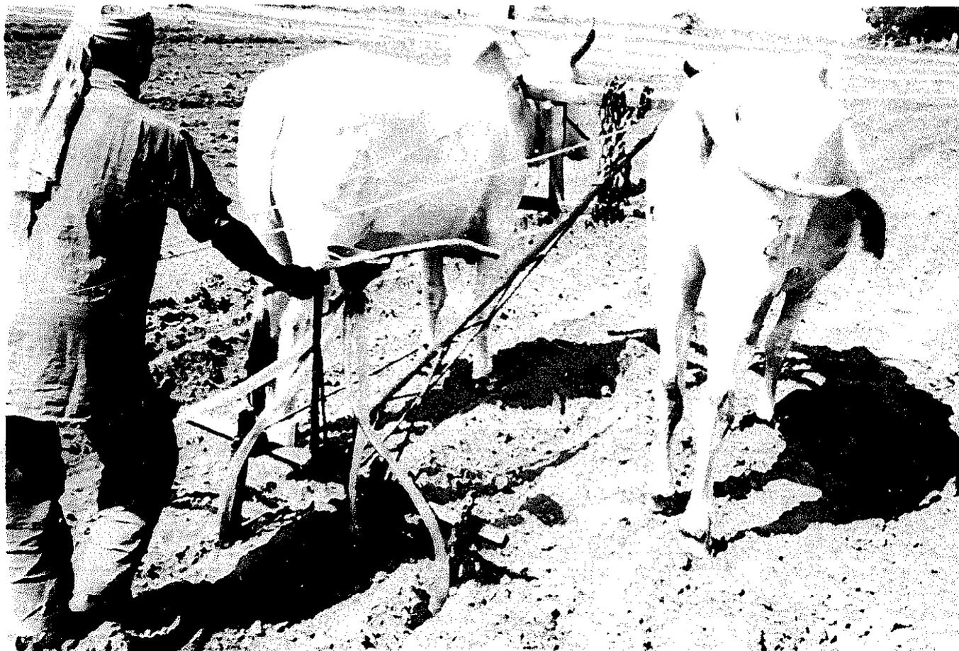
*Innovative equipment can be simple in construction: a four-furrow row seeder.*
