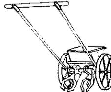
This type of hand-pushed, 2-row rice seed drill is equipped with 2x25 cm sowing ploughshares. The distributors are mounted on the wheel axes and can be adjusted for up to 130 seeds per meter.
