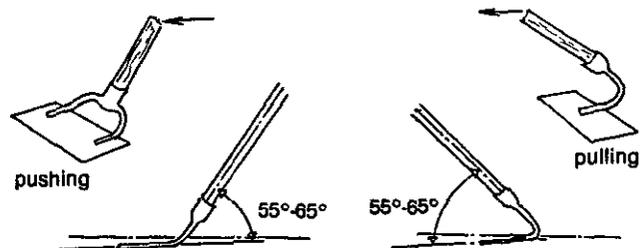
Fig.1 Pushing and pulling hoes, showing working angles.
