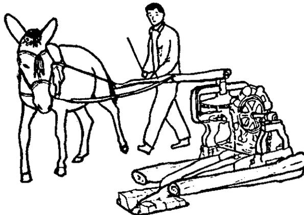
**ANIMAL POWERED MONOLIFT PUMP** This rotary pump is an adaptation of the Monolift borehole pump. Suitable for maximum lifts from 30 to 110m depending on type and number of animals used. Maximum output ranges from 1.2 to 4.6m<sup>3</sup>/h.
