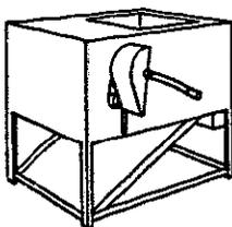
**RÖBER HAND WINNOWER (Illustrated left)** This is a hand-driven winnower featuring 3 sieves, and a built-in ventilator. It has a capacity of 1.5 tonnes/h.
