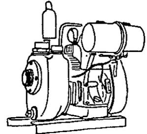
priming 50mm models are available, the 4250 and 4256. They can be close coupled to a choice of power units — petrol, kerosene, and diesel engine or electric motor up to 2.2kW. Typical performance 15m<sup>3</sup>/h at 18m total head. 80 and 100mm sizes also available skid or trolley-mounted.
