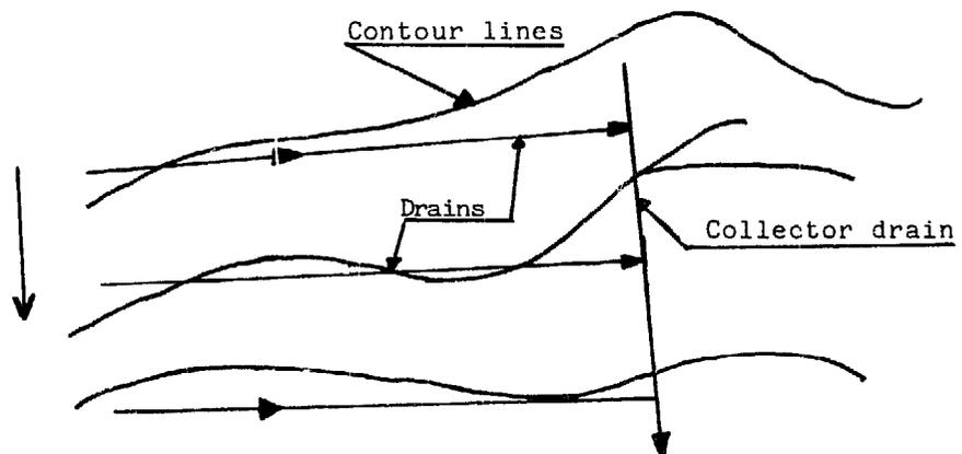
The collectors are always laid out along the line of greatest slope. The main collectors are situated in the main thalwegs and the secondary collectors in the secondary thalwegs.
