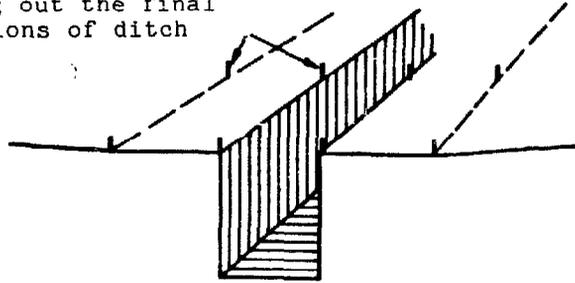
Phase 1: Staking out the final width and vertical excavation down to specified depth
