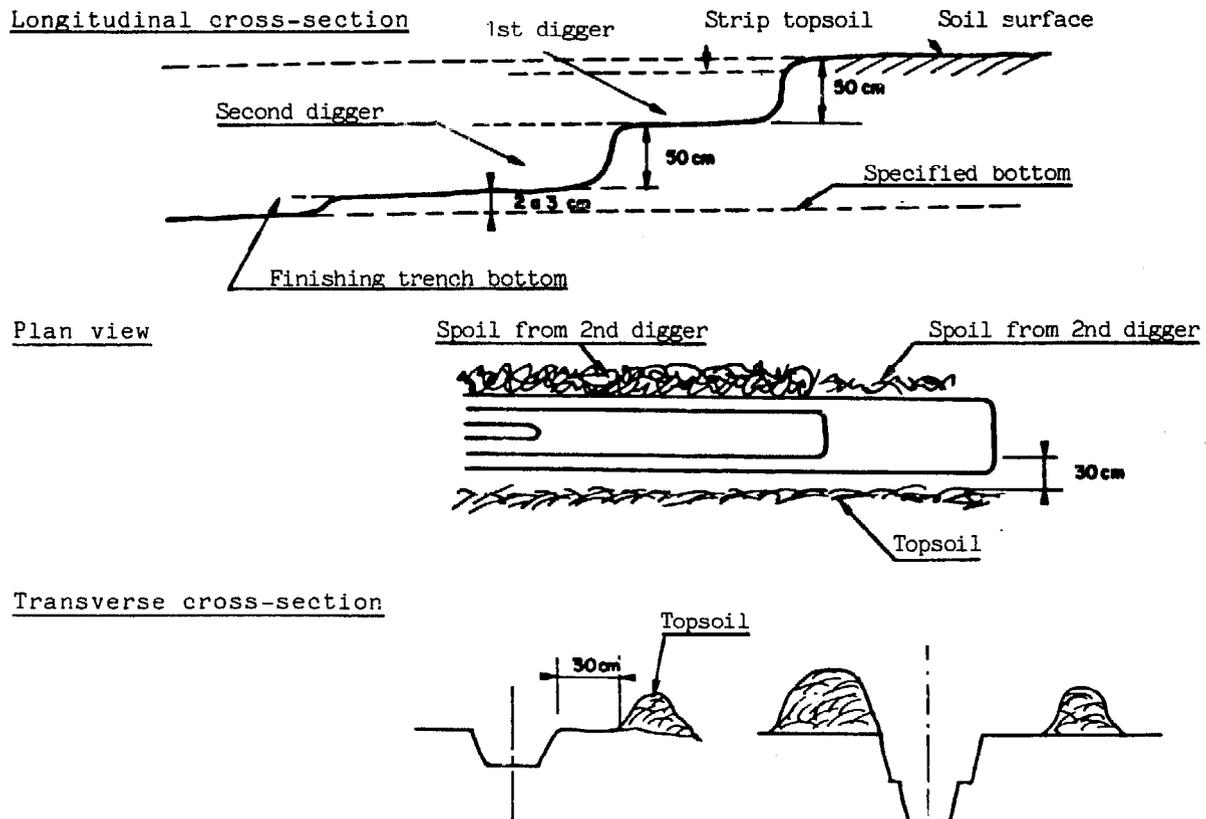
The first digger cuts up the sod and removes the topsoil. This topsoil is placed on the right of the trench about 30 cm from the trench edge leaving a pathway for the pipe layer. This topsoil is the first to be used when the trench is backfilled.
