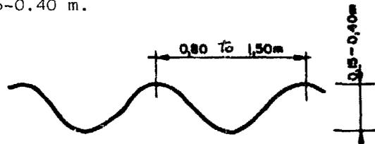
In low-rainfall areas, contour ridges may be tied by clods of earth at intervals of 3-15 m, which ensures total infiltration and increases the soil's water reserve.
