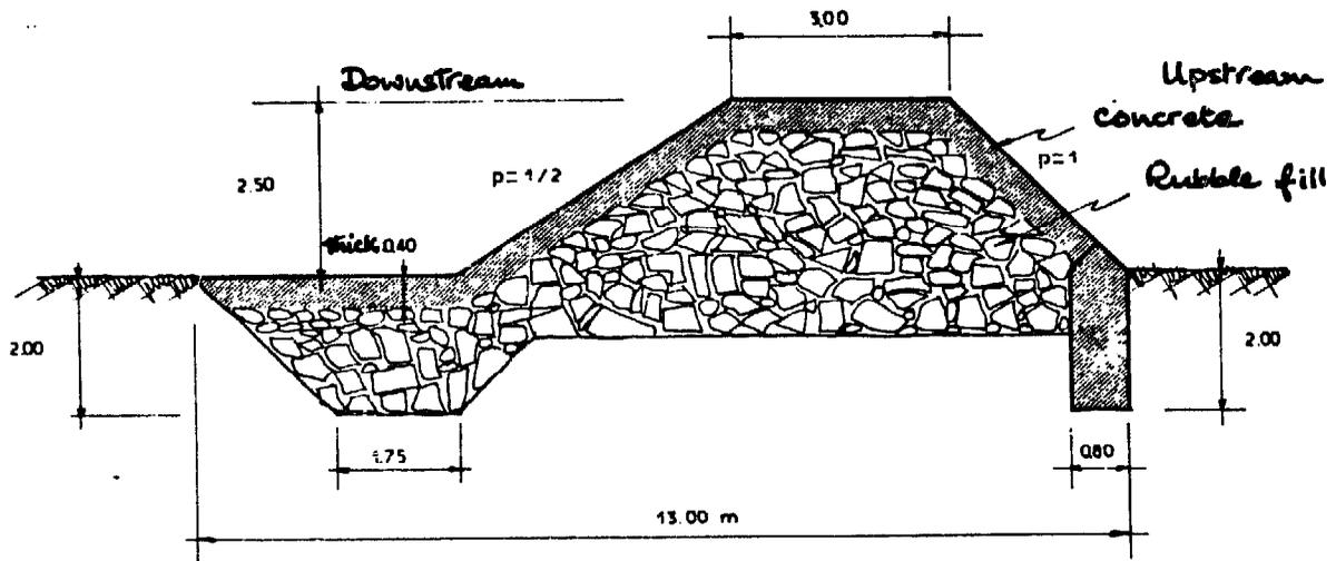
WEIR MADE FROM RUBBLE FILL FACED WITH CONCRETE
