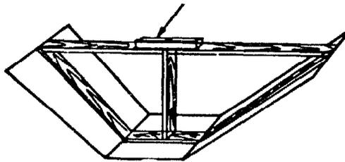
Phase 4: Checking the cross-section with a spirit level
