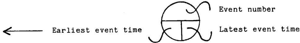
Task or activity: shown by a line, the length of which is independent of the actual time required to complete it. This line ends in an arrow which shows task sequence.
