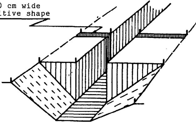
Phase 2: Excavation of a trench to final width of the ditch
