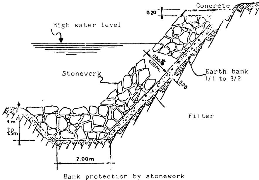
If the base of the bank is accessible at low water, a footing is installed at the stonework base in a trapezoidal trench 1-1.50 m deep and 1-2 m wide at the base.
