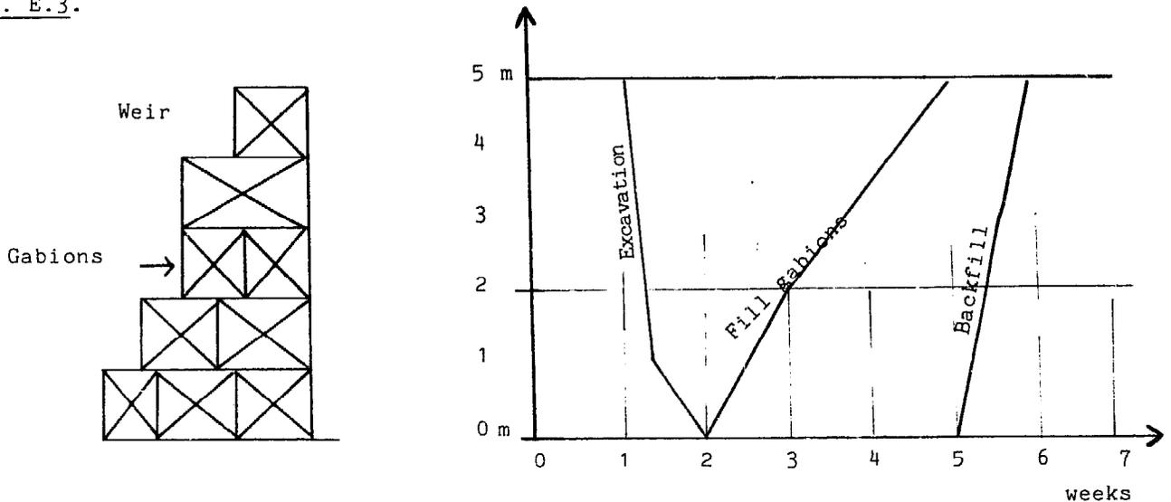
The example of the construction of an embankment and irrigation channel previously plotted on a GANTT-type bar chart looks as follows when plotted on a time and location chart.
