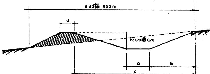
**CHANNEL-TYPE FLATTENED CROSS-SECTION TERRACE (CROPPING TERRACE)**
