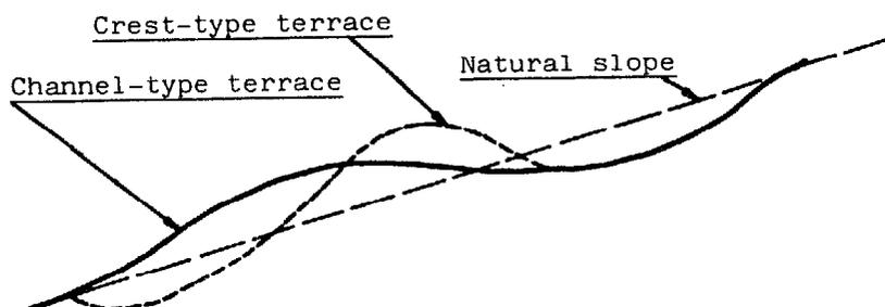
Fig. B.3: Main types of tiering and terracing
