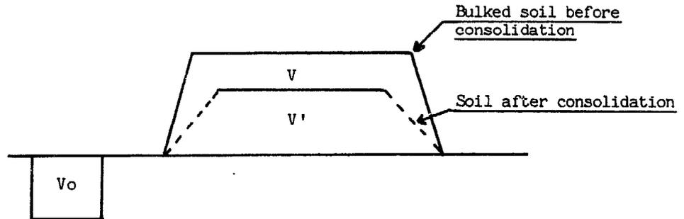
Fig. E.17: Values of coefficients of bulking and consolidation
