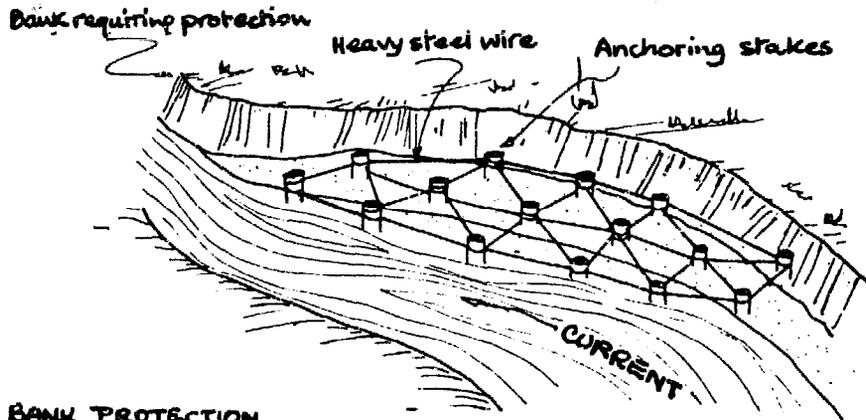
BANK PROTECTION BY ANCHORING STAKES intertwined with steel wire
