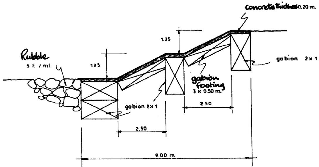
WEIR MADE FROM GABIONS AND CONCRETE
