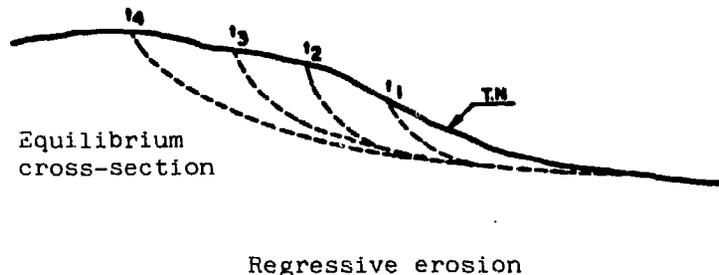
Regressive erosion gradually moving downhill in a watershed may finally result in all the soil of a watershed being stripped away before the equilibrium cross-section is reached. In order to conserve this cultivation soil, it is necessary to prevent the progression of this form of erosion.
