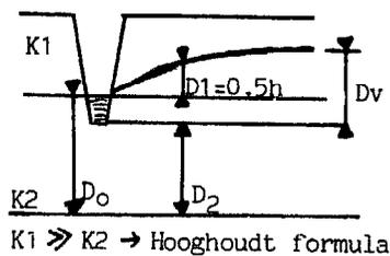
Drain at the boundary of two layers of different permeability
