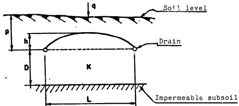
The optimum level of the water table ( $p-h$ ) is the basic datum in drainage problems and it is dependent on crop requirements. The other data are input rate or "characteristic flow rate"  $q$ , the depth  $D$  and the permeability  $K$  of the drained layer.
