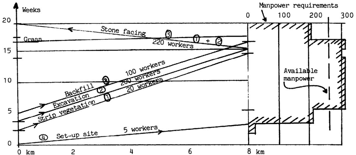
Reading this type of chart poses no major difficulty. The main components of the project are shown, the operations are located in time and space, and the logic behind the programming and scheduling of tasks is indicated. The actual advance of the work can be plotted on the chart in dotted lines and any delays will show up clearly. A diagram showing resource requirements (manpower, materials, equipment) can be added to the right of the chart.
