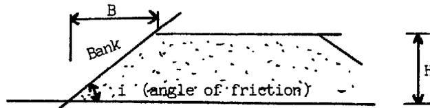
Knowledge of the angle of repose is essential in ensuring the stability of earthworks and in estimating the area they will occupy and the volume of earth to be moved.
