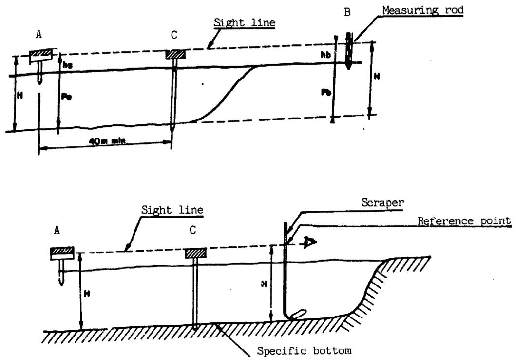
At point A marked by a stake, where the depth  $P_a$  of the trench is known, one places a fixed boning rod adjusted to height  $h_a$  above the ground. The height of the boning rod above the bottom of the trench is equal to  $P_a + h_a = H$ .
