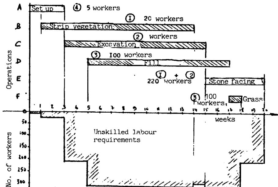
To the lower section of the planning chart it is possible to add a diagram indicating labour, tool, equipment, etc, requirements. Improvements can also be made by joining up the various operations by arrows (linked GANTT chart) to show gang movements during operation of the site.
