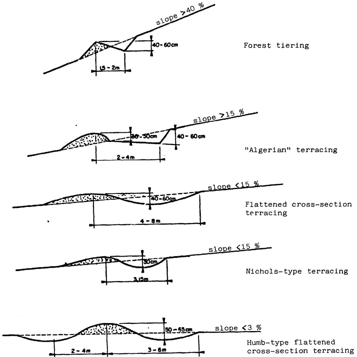
Crest-type terraces are kept on the level. They are used for lightly sloping ground ( $\leq 3-4\%$ ) which is very permeable (sandy).
