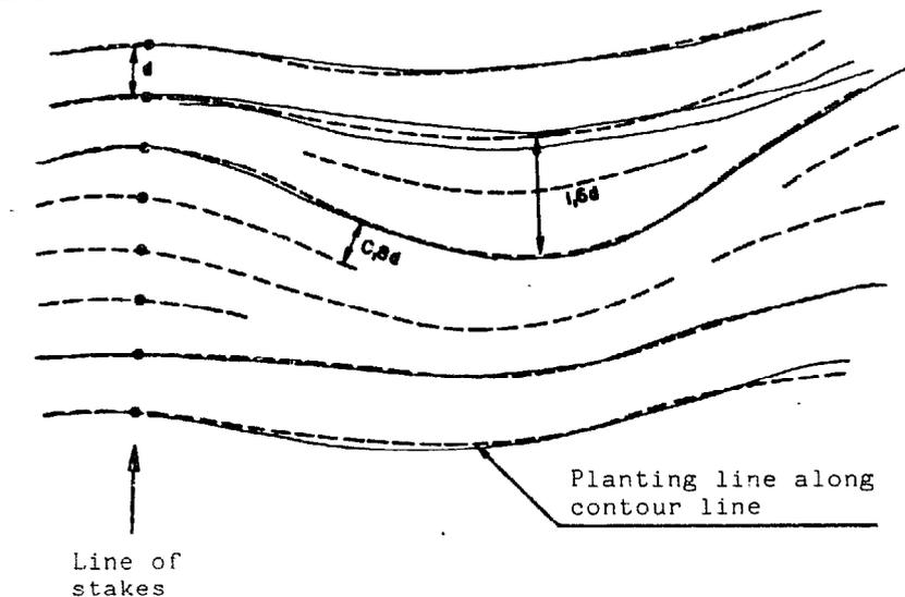
With an interval  $d$  between plants, a line of stakes is inserted perpendicular to the slope and spaced at  $d$  from each other.
