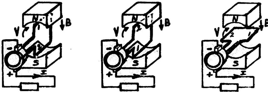
Fig. B.6. Electric machine with commutator
