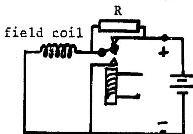
Fig. 4.21. A field current relay with 3 contacts. When the generator voltage is only slightly too high contact a-b will open and the (diminished) field current flows through the resistor R. When the voltage rises still further, contact b-c closes and the field coil is short-circuited.
