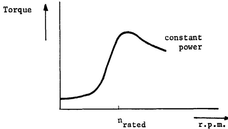
Fig. 4.17. The idealized torque speed curve of a generator
