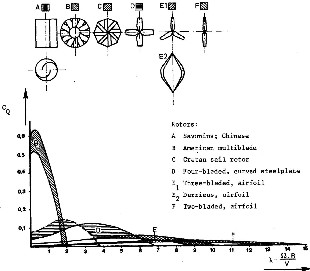
Fig. 4.6. The corresponding torque coefficients of the rotors in fig. 4.5.
