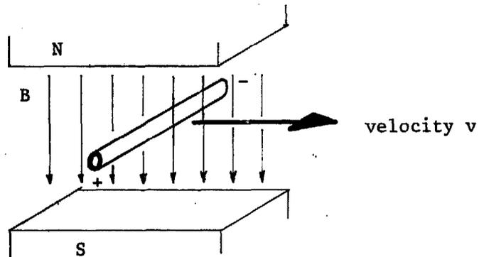
Figure B.2. A moving conductor placed in a magnetic field.
