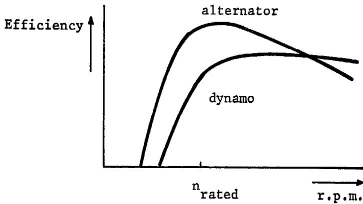
Fig. 4.15. The efficiency speed curve of a dynamo and an alternator
