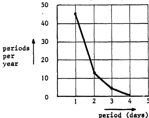
Fig. 3.12. The number of periods per year during which the wind speed was lower than 2 m/s.
