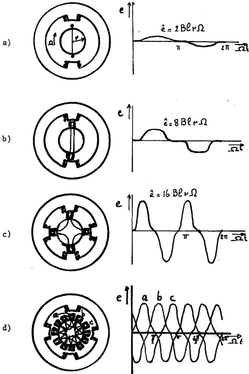
Fig. B.8 Examples to demonstrate how to use the magnetic field in a generator more effectively
