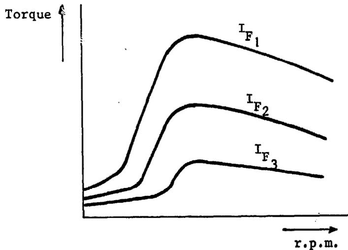
Fig. 4.19. The torque speed curves of an alternator for different values of the field current ( $I_{F1} > I_{F2} > I_{F3}$ )
