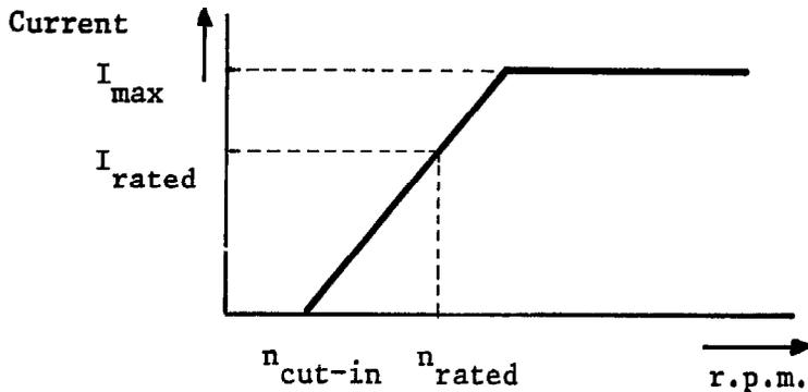
Fig. 4.16. The idealized current speed curve of a generator equipped with a current limiting device
