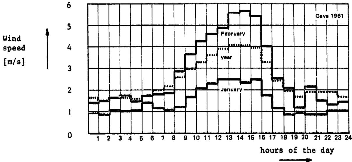
Fig. 3.4. The monthly and annual mean hourly wind speeds during the day at Gaya (India) in 1961. The mean monthly wind speed in January is 1.4 m/s, in February 2.7 m/s, while the mean annual speed is 2.4 m/s.
