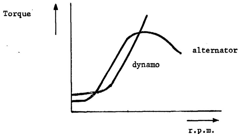
Fig. 4.13. The torque speed curve of a dynamo and an alternator
