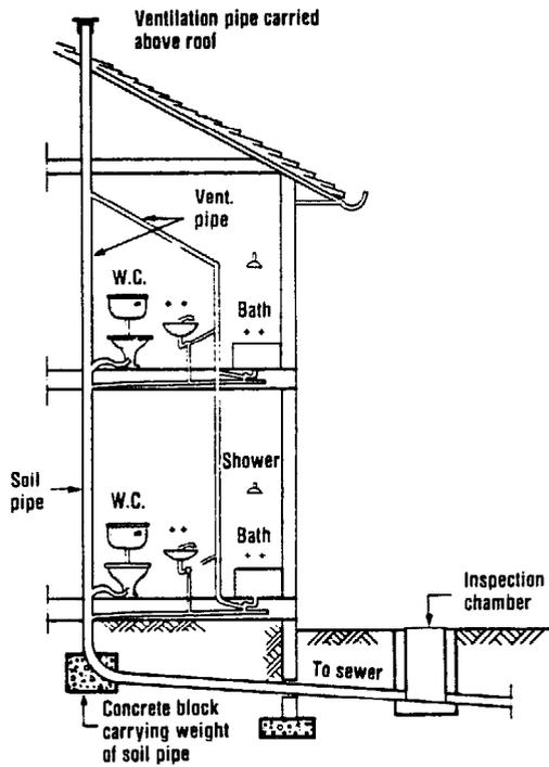
B. Principle of the 'two-pipe' system.
