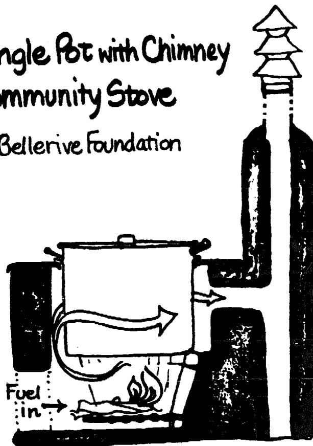
A long flame path is created by resting the pot on a semi-circle of bricks. The flame travels across the bottom, toward the front, and around the sides of the pot before reaching the chimney.
