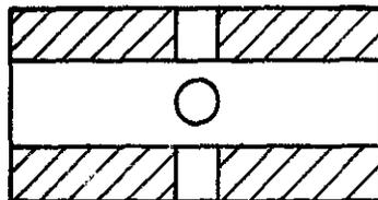
Cross section of the finished oil-soaked wood bearing showing grease reservoir holes.
