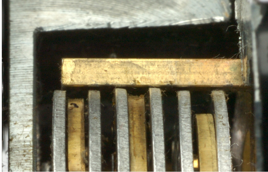
Figure 13: Imperfections in wheel pack and fence. Only the “largest” wheel actually determines the depth to which the fence lowers. Sometimes the wheels are of slightly different diameter (as shown here), and sometimes the fence is not exactly parallel with the wheel pack. In this cutaway view of an off-the-shelf S&G 6730, the middle wheel is slightly larger.
