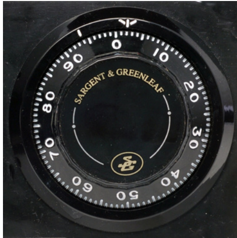
Figure 2: External dial (user interface) of common Group 2 lock (again, a Sargent & Greenleaf model R6730). The actual dial , with 100 graduations, rotates; the surrounding dial ring is fixed to the container. The main index mark at 12 o'clock (shown here at dial position 2) is used for dialing the combination to open the lock; the smaller index mark at 11 o'clock (at 94) is used only when setting a new combination.
