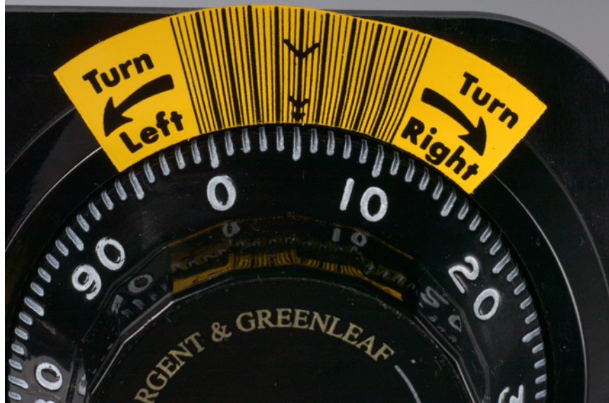
Figure 15: A simple manipulation aid – a sticker marked with a 1/4 graduation scale.
