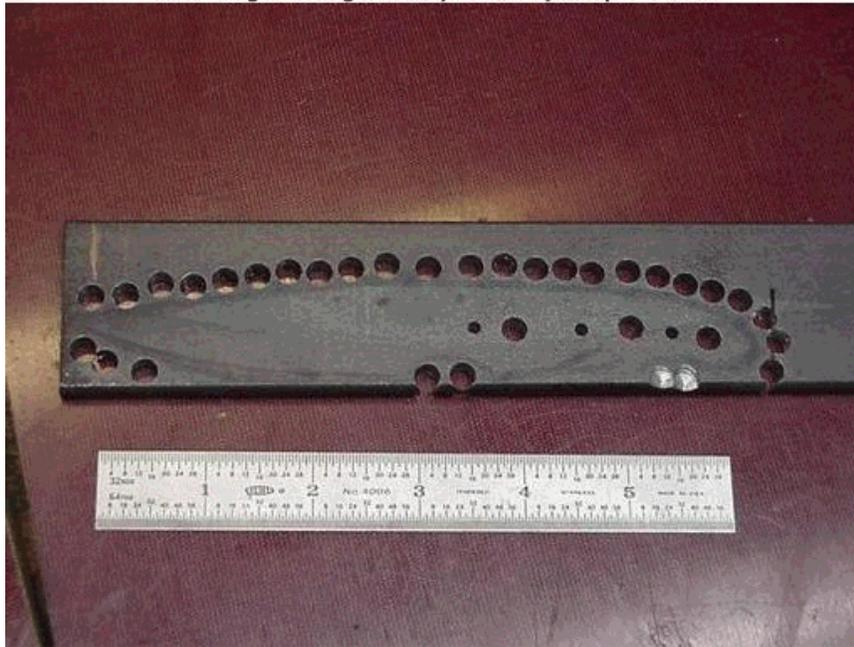
pic #2 Screw the blade to a bench or stump or whatever you have and cut out the handle portion only. Remove the material so you can file the handle to shape. Do this first because you won't have any way to screw the blade to the bench if you cut out the entire blade. do the handle work first! Once the handle is to a pretty good shape remove and screw to the bench through the handle and cut out blade.
