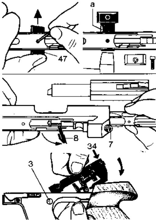
Push the spring-loaded pin inward, at the same time pushing the cocking knob (47) out (see arrow). On Model OSP, Cal. .32 S & W lg., first remove one cocking knob by loosening the Allen screw, then push the spring-loaded pin inward and tap the tight-fitting cocking grip out sideways. When inserting the cocking grip, the liner (a) must point to the rear.
