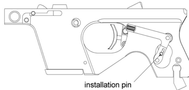
When assembling the weapon, the correct fit of the **installation pin** has to be absolutely checked and verified.
