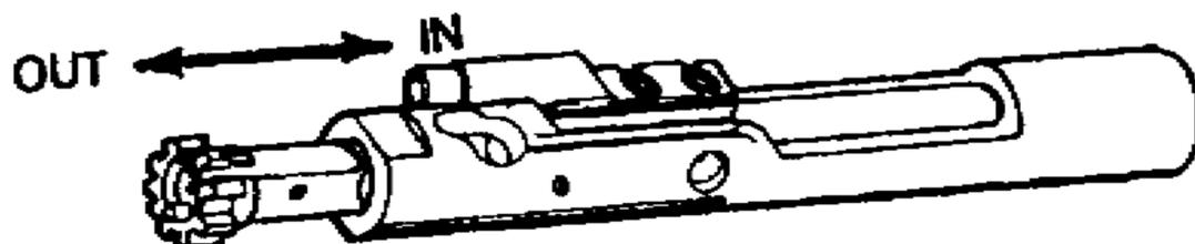
Check for proper fit with cam pin removed. Turn bolt carrier assembly and suspend so the bolt assembly is pointed down.
