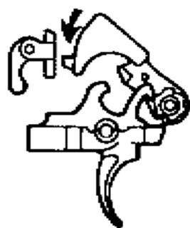
f. As the bolt carrier assembly moves to the rear, the hammer is forced to the rear.
