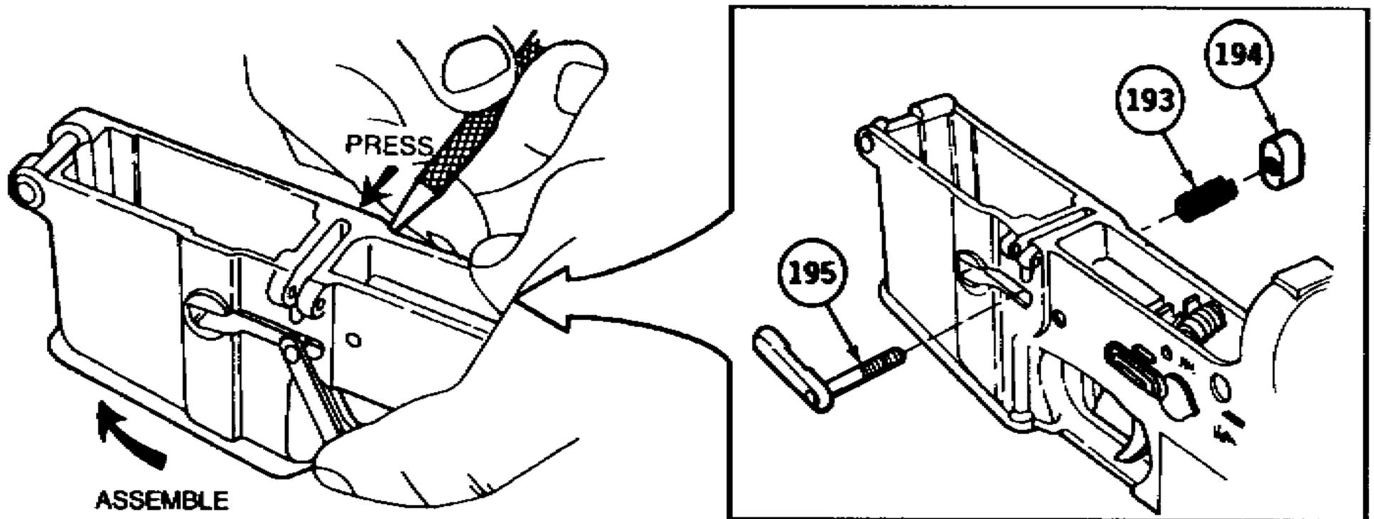
j. Helical spring (196), bolt catch plunger (197), and bolt catch (198).
