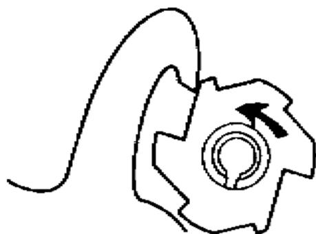
g. The clutch spring of the burst cam clutches the cam and causes it to rotate one notch as the hammer is forced back.
