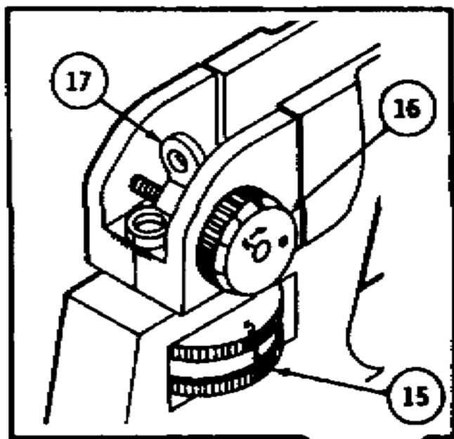
Rear sight elevation (15) and windage (16) knobs must rotate freely with distinct "clicks". Rotate elevation knob counter clockwise until the rear sight is all the way down. If a whole click is not felt as the sight stops, the sight has bottomed out and will not pivot freely.
