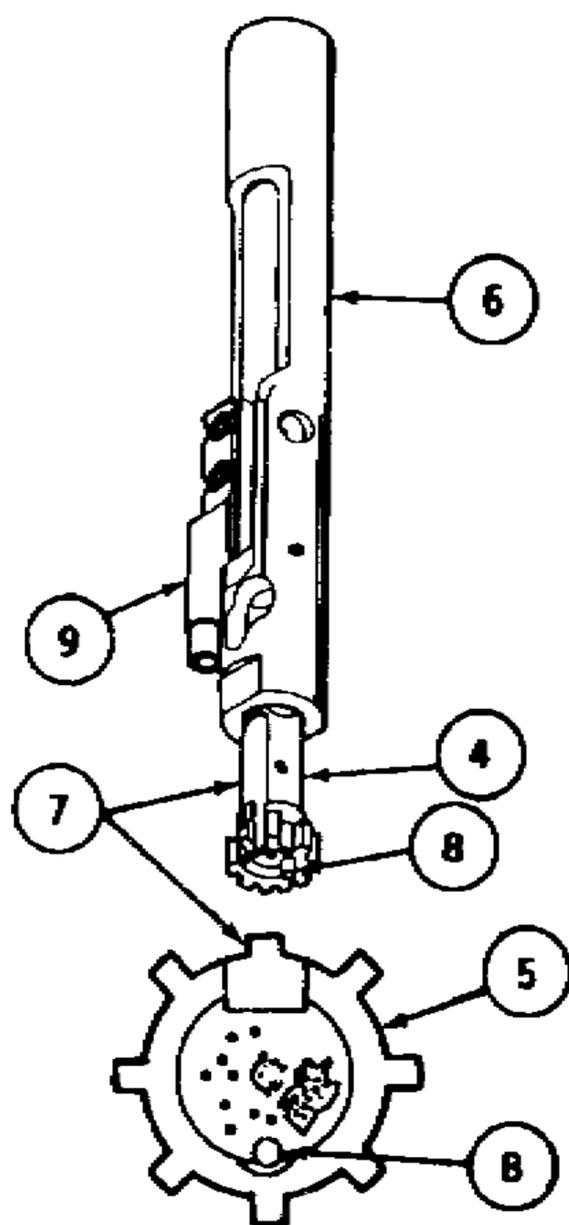
Check for worn bolt rings. Insert the bolt assembly (4) into the bolt carrier (do not insert cam pin) and exercise in and out to check for binding. Turn bolt carrier assembly (6) so the bolt assembly (4) points down. The bolt must not drop out. If the bolt assembly drops out of the bolt carrier due to its own weight, evacuate to intermediate maintenance for repair (usually bolt ring replacement).
