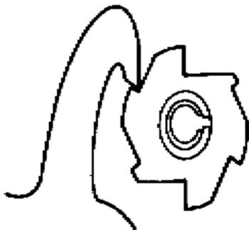
o. The front hook of the burst disconnect is now fully in the third notch.
