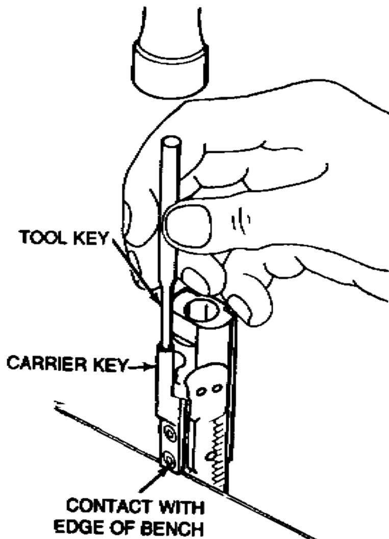
Place the key and bolt carrier assembly in a vertical position, supported in a manner that contact is made with the rear surface of the key.
