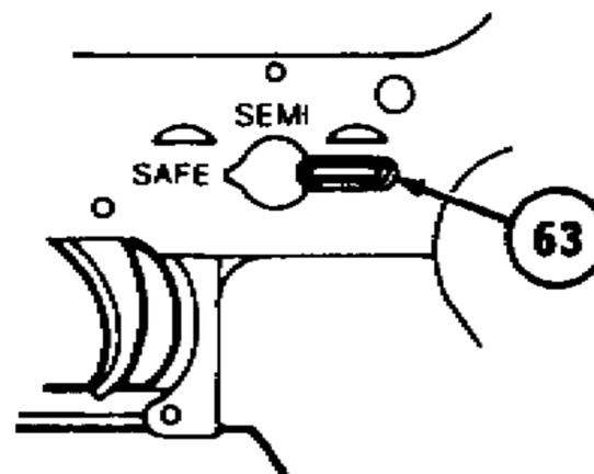
12. FIRES TWO ROUNDS WITH ONE SQUEEZE OF TRIGGER WITH SELECTOR LEVER (63) SET ON SEMI (DOUBLE FIRING).
