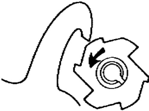
m. The clutch spring of the burst cam clutches against the cam and causes it to rotate one notch as the hammer is forced back.
