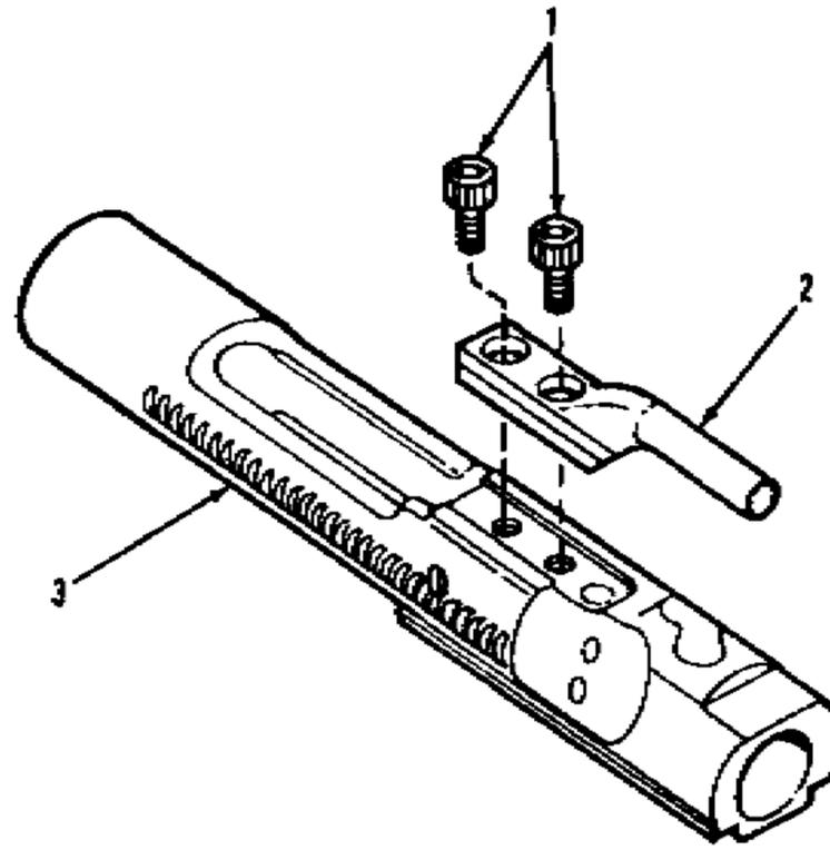
**Figure C-4. Key and bolt carrier assembly 8448505**
