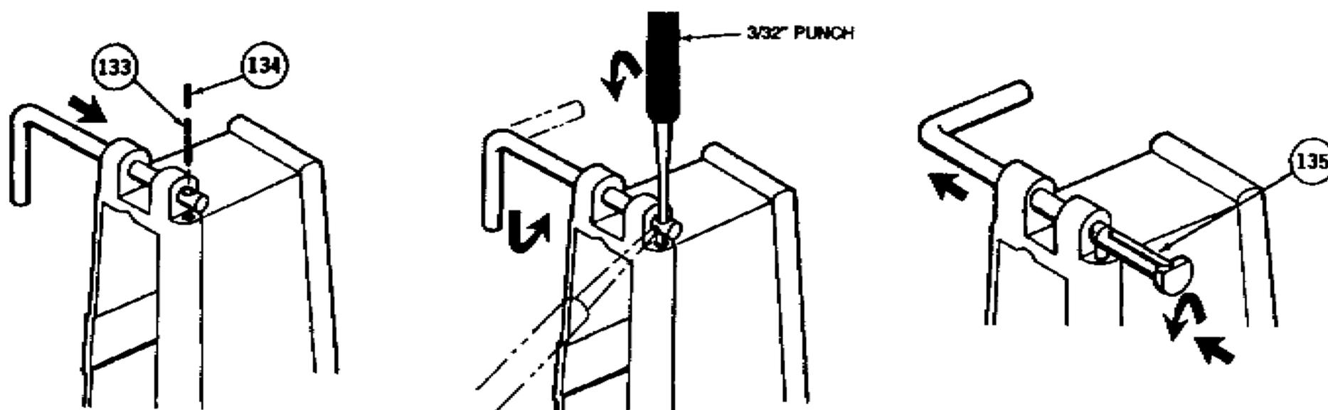
Remove punch. Push out tool using pivot pin (135)
