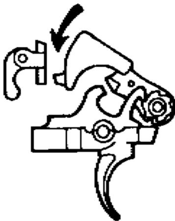
r. As the bolt carrier moves to the rear, the hammer is forced back to the rear.
