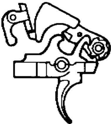
n. When the hammer is fully to the rear, the automatic sear catches it.
