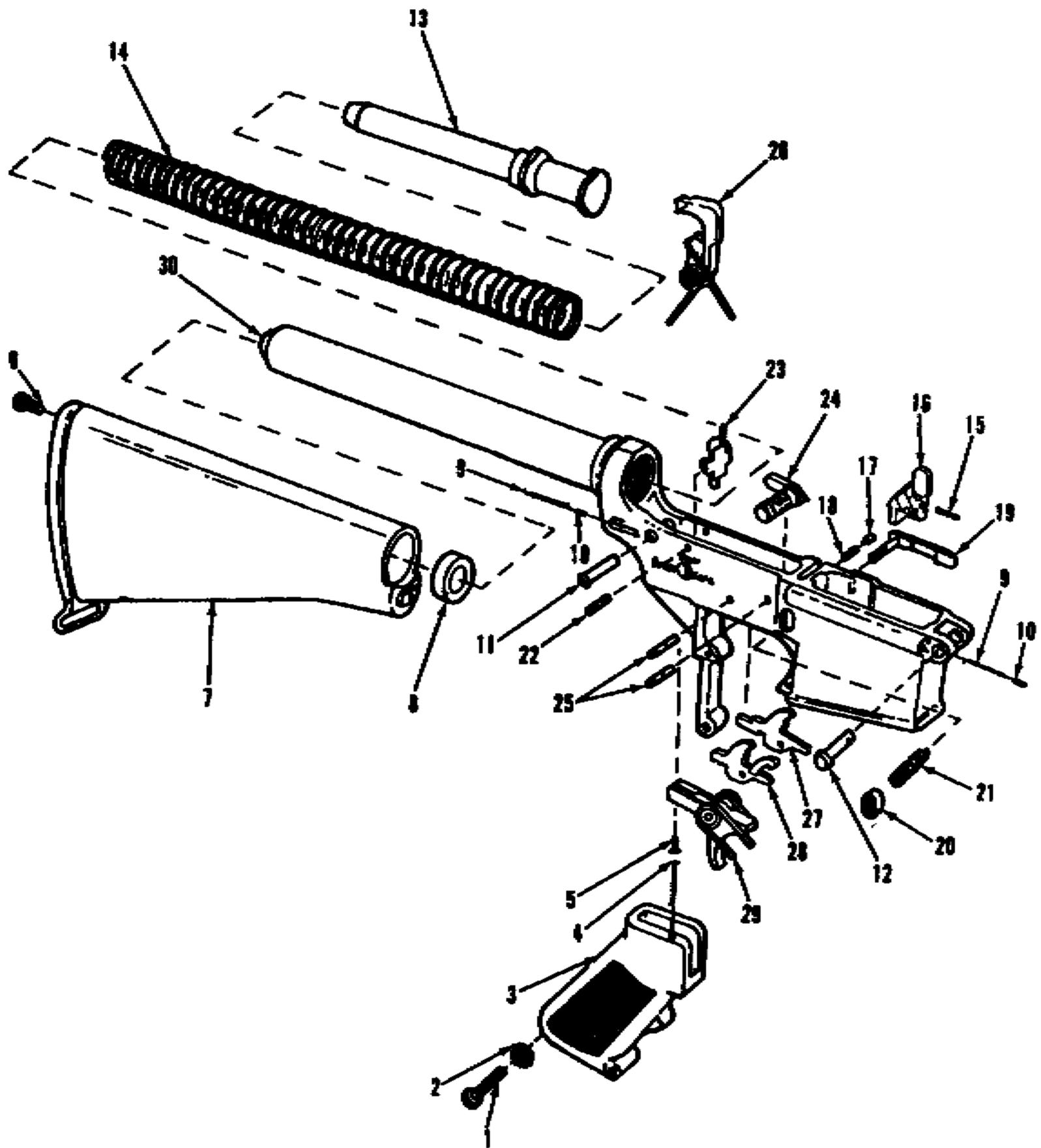
**Figure C-10. Lower receiver and buttstock assembly 9349100**
