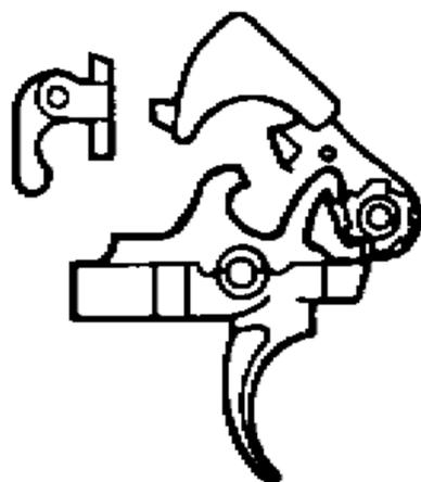
t. When the hammer is fully to the rear, it is initially caught by the automatic sear. However, the front hook
