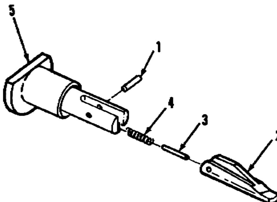
**Figure C-9. Forward assist assembly 9349086**
