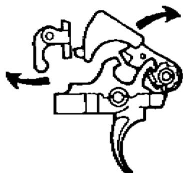
j. As the bolt carrier assembly travels forward, the automatic sear releases the hammer and the hammer falls.
