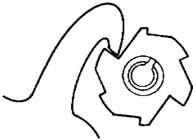
of the burst disconnector is now fully in the next stop notch which is deeper than the others.
