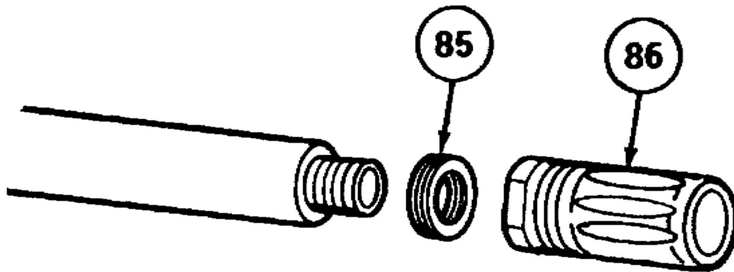
Torque to 15-20 ft-lb using combination wrench and 1/2" drive torque wrench. Torque is measured when both wrenches are used together.
