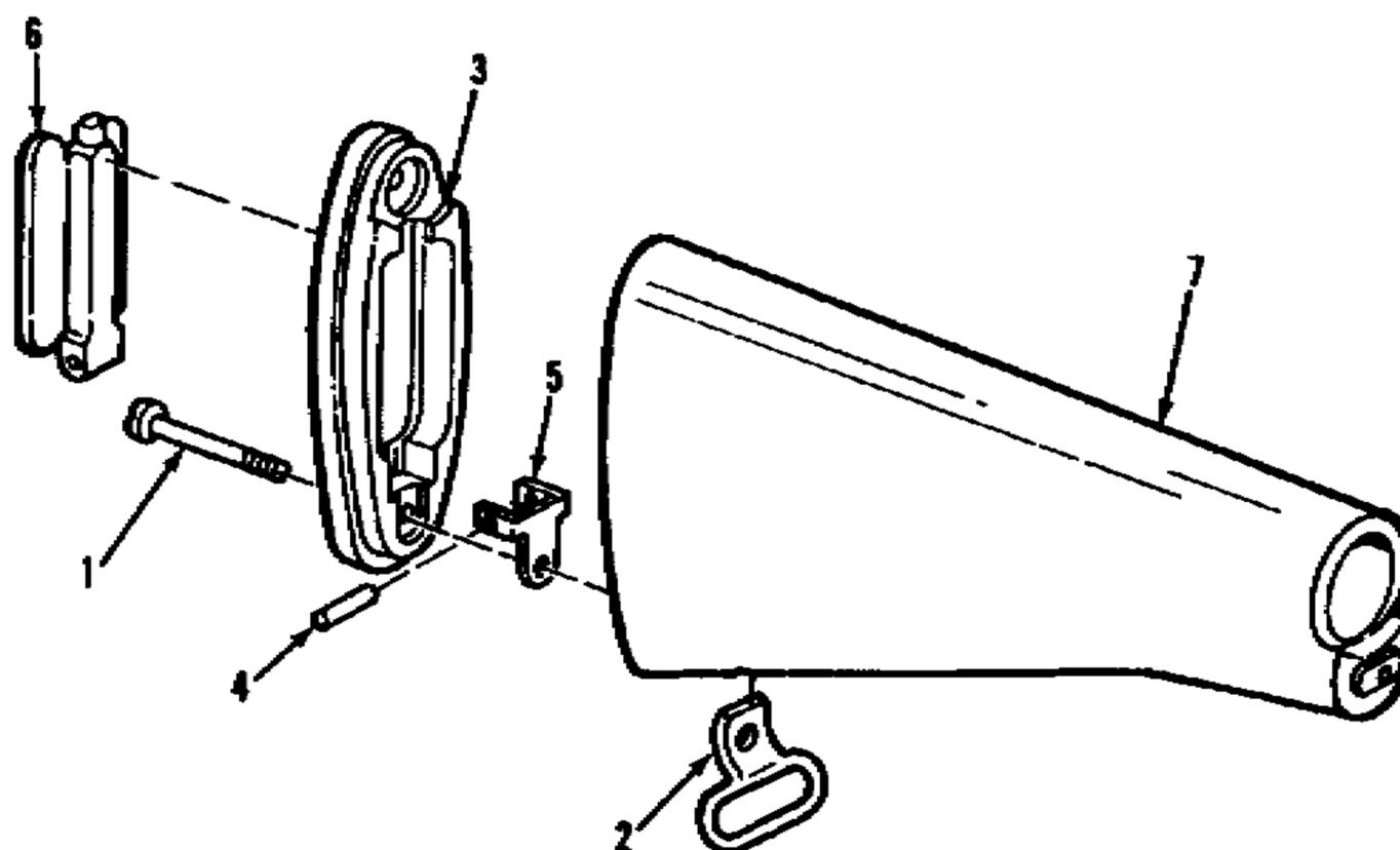
Figure C-11. Buttstock assembly 9349119
