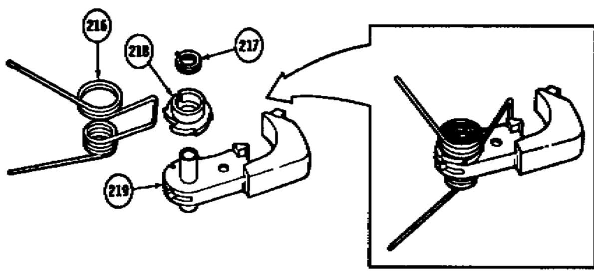
**3-18. TRIGGER ASSEMBLY (INTERMEDIATE).**
