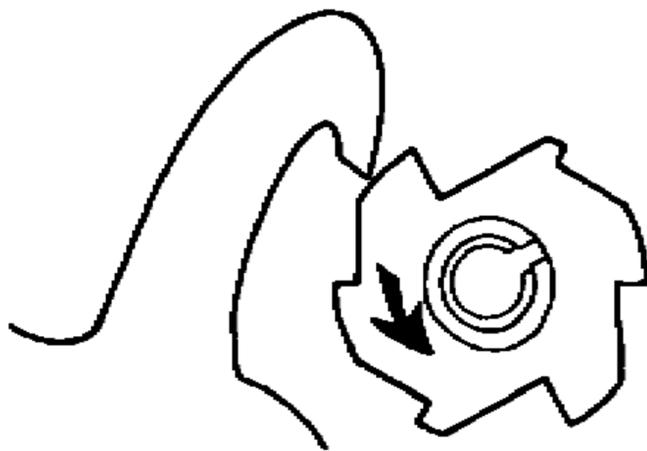
s. The clutch spring of the burst cam clutches against the cam and causes it to rotate one notch as the hammer is forced back.
