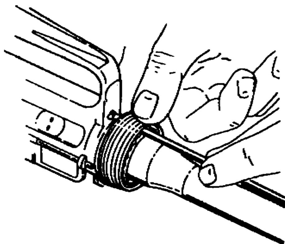
If necessary, tighten nut to next hole to allow proper alignment. Remove upper receiver and barrel assembly from barrel remover fixture.
