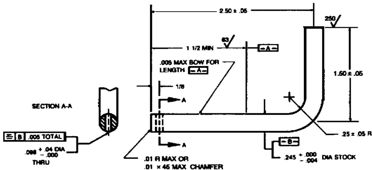
FABRICATE FROM .245 IN. STEEL A1S1 1095 OR EQUIVALENT. HARDEN AND TEMPER TO RC-57-61 FOR LENGTH - A-. FINISH 5.3.1.2 OR 5.3.2.2 OF MIL-STD-171.
