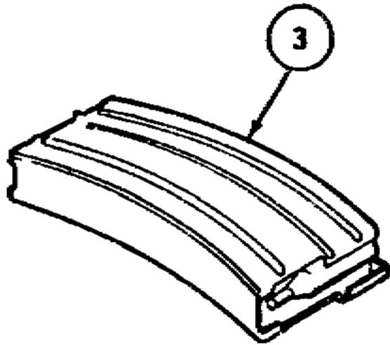
Disassemble as in TM 05538C-10/1. Inspect tube for bulges, dents, or damaged feeder lips. Inspect spring and follower for kinks or damage. Replace the magazine if any of the above conditions exist. Floor plate must be positively retained when reassembled.
