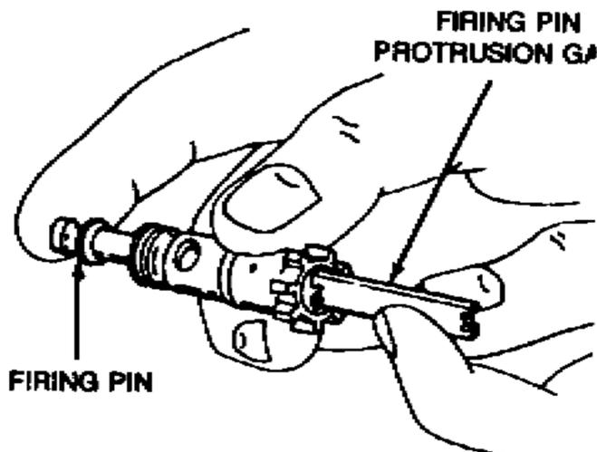
Insert firing pin through bolt assembly.
