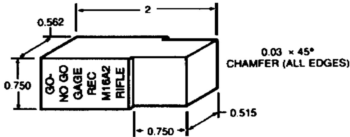
FABRICATE FROM 0.750 SQUARE METAL BAR, QQ-T-580, GRADE C, CLASS W2-09 OR CLASS 62-10 NSN 9510-00-541-958 OR EQUIVALENT.
