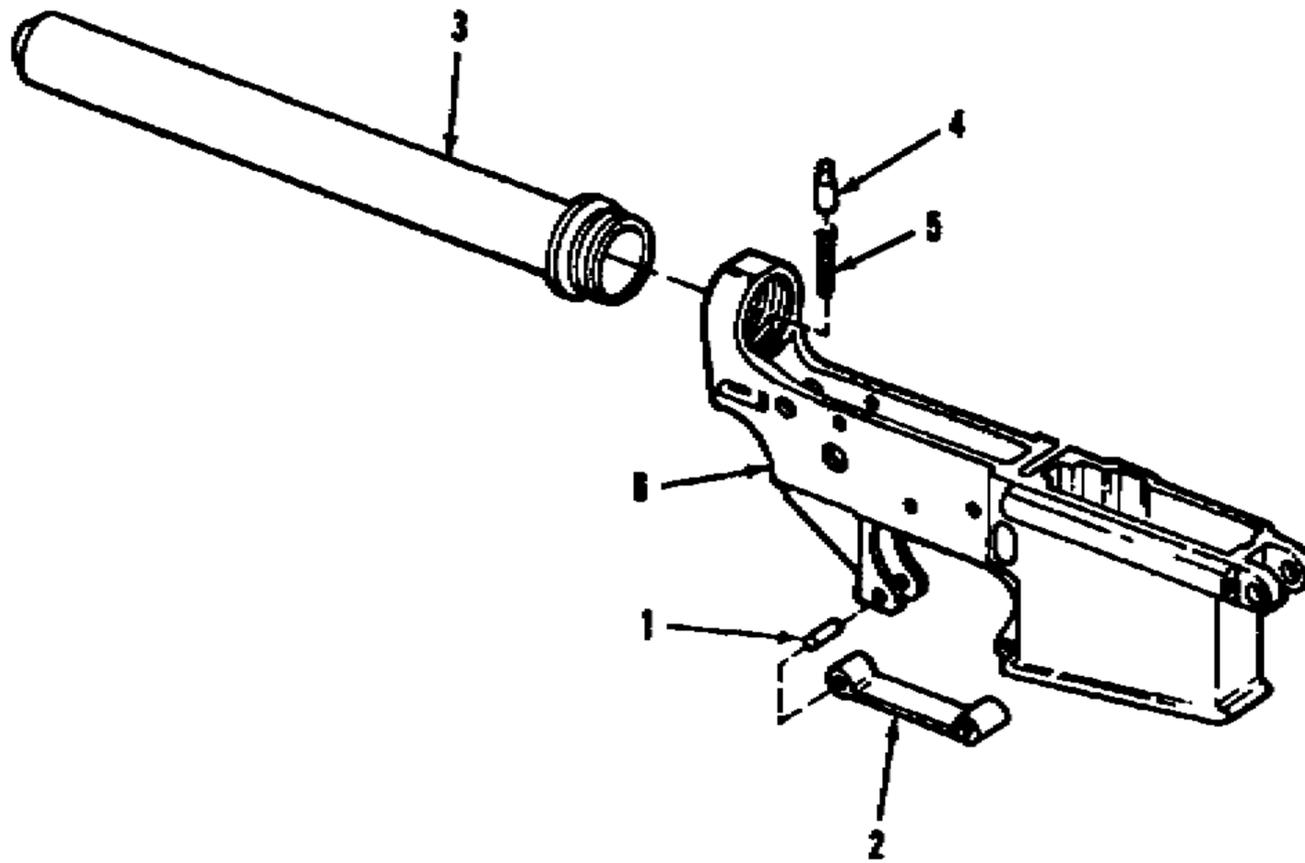
Figure C-14. Lower receiver and receiver extension assembly 9349101
