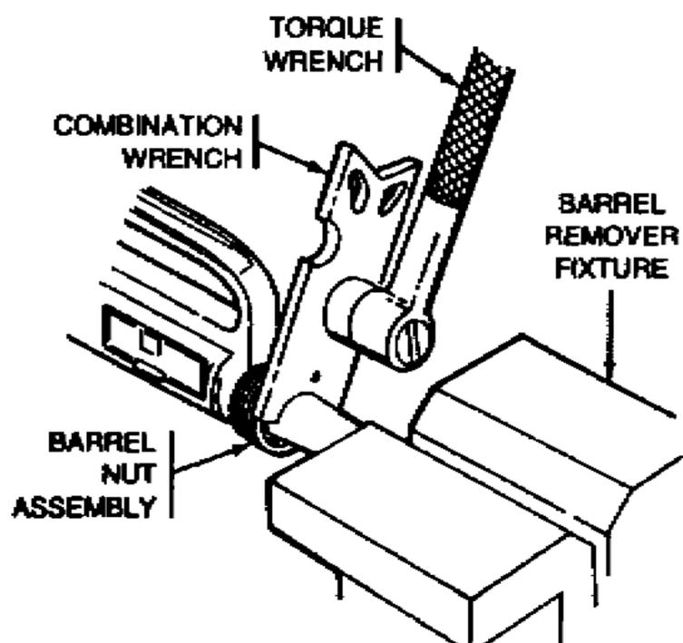
Engage threads of barrel nut assembly with upper receiver assembly.
