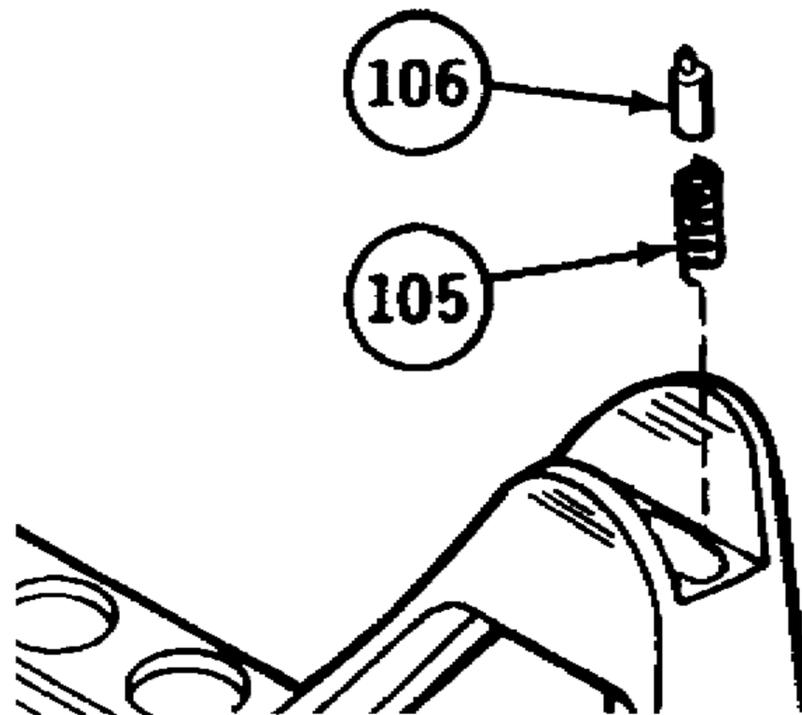
Position and depress helical spring and front sight detent with front sight detent depressor (E-1, app E).
