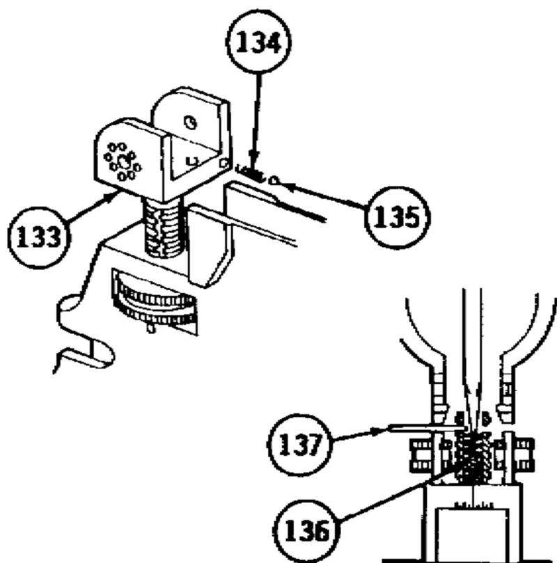
Insert helical spring (136) through underside of receiver. Install spring pin (137) while helical spring is held compressed.
