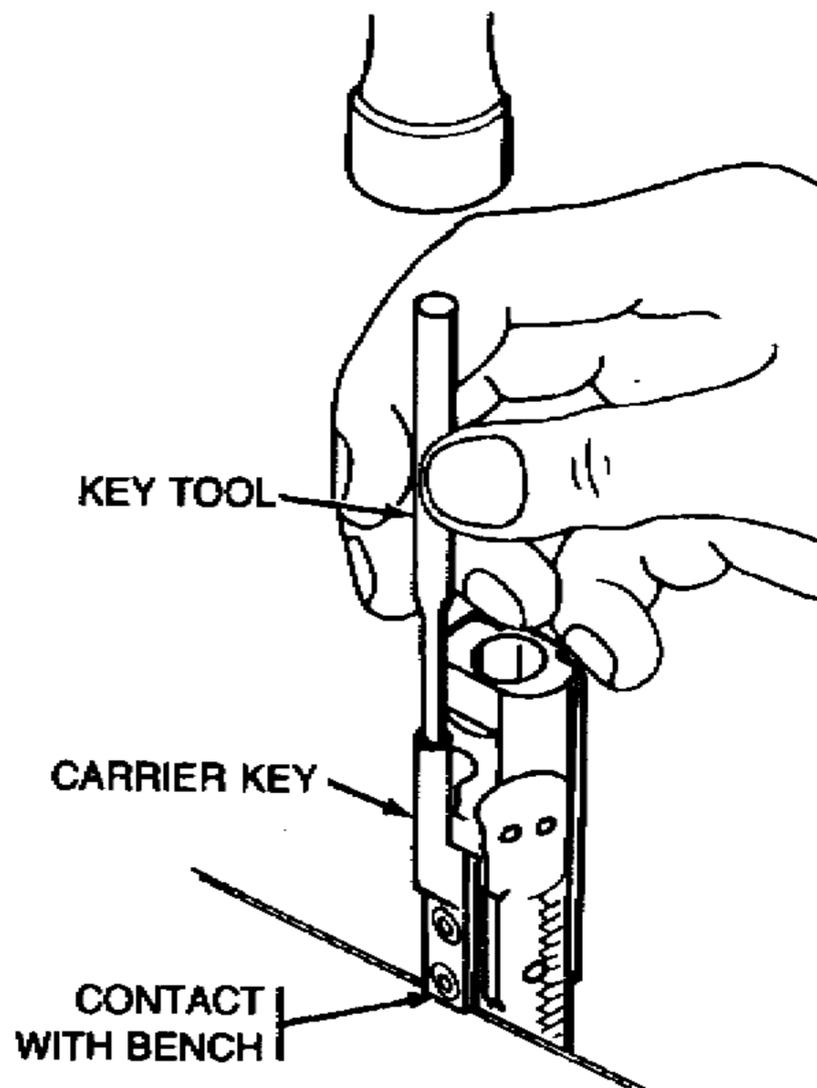
Place the key and bolt carrier assembly in a vertical position, supported so that contact is made with the rear surface of the key.
