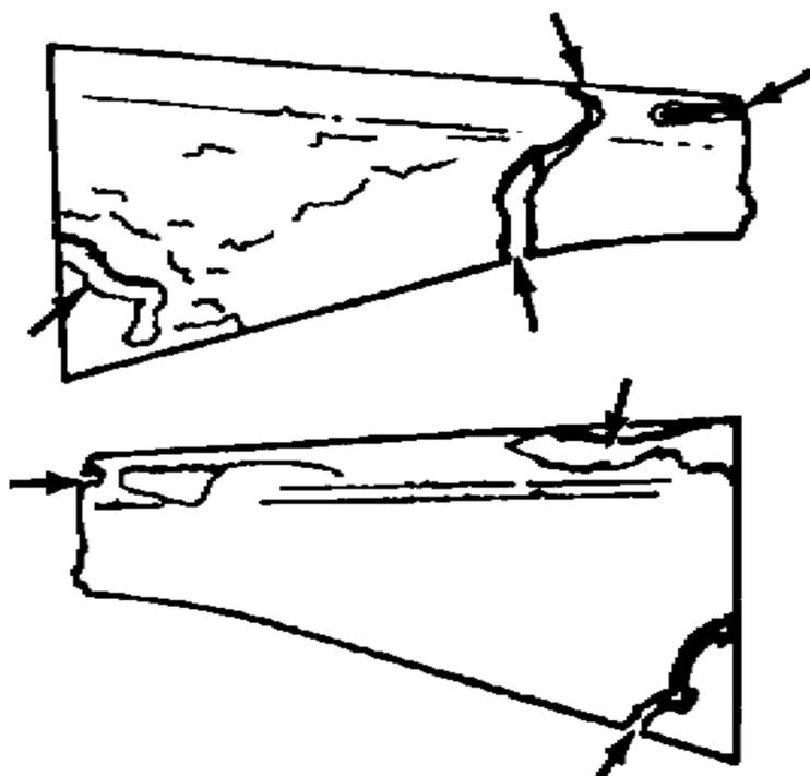
BUTTSTOCK - NONREPARABLE DAMAGE
