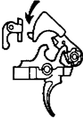
l. As the bolt carrier assembly moves to the rear, the hammer is forced back to the rear.
