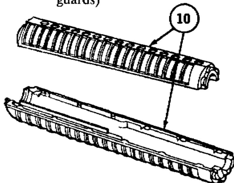
Remove and inspect handguards (10) internally and externally for cracks and/or damage. Cracks up to one inch in length are acceptable providing they do not extend into the handguard retaining flange.
