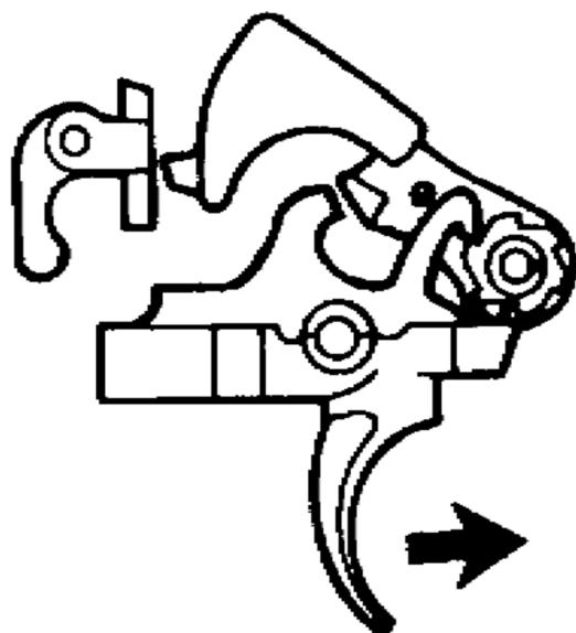
v. Once the trigger is released, the trigger nose comes up and holds the hammer back.
