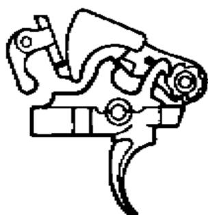
h. When hammer is fully to the rear, the automatic sear catches it.
