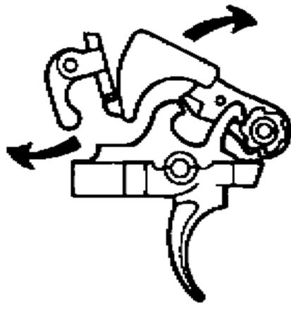
p. As the bolt carrier assembly travels forward, the automatic sear releases the hammer and the hammer falls.
