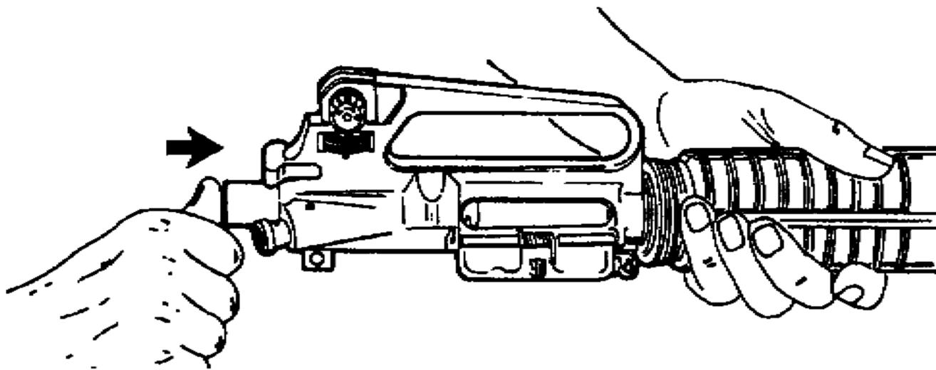
Remove bolt carrier and bolt assembly and charging handle and headspace gage.
