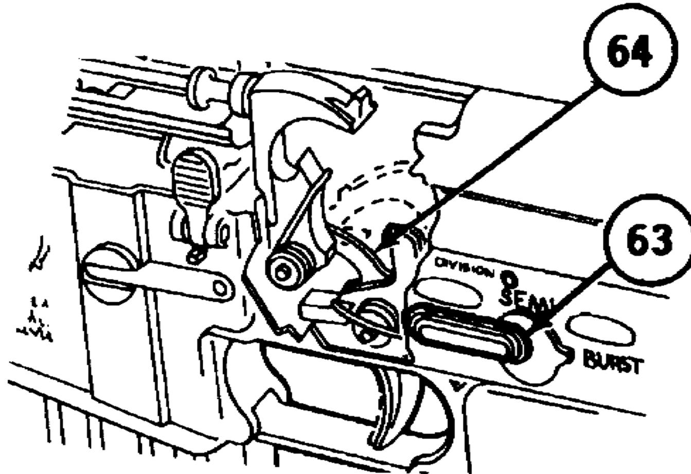
11. FIRES WITH SELECTOR LEVER (63) ON SAFE OR WHEN TRIGGER IS RELEASED WITH SELECTOR LEVER ON SEMI.
