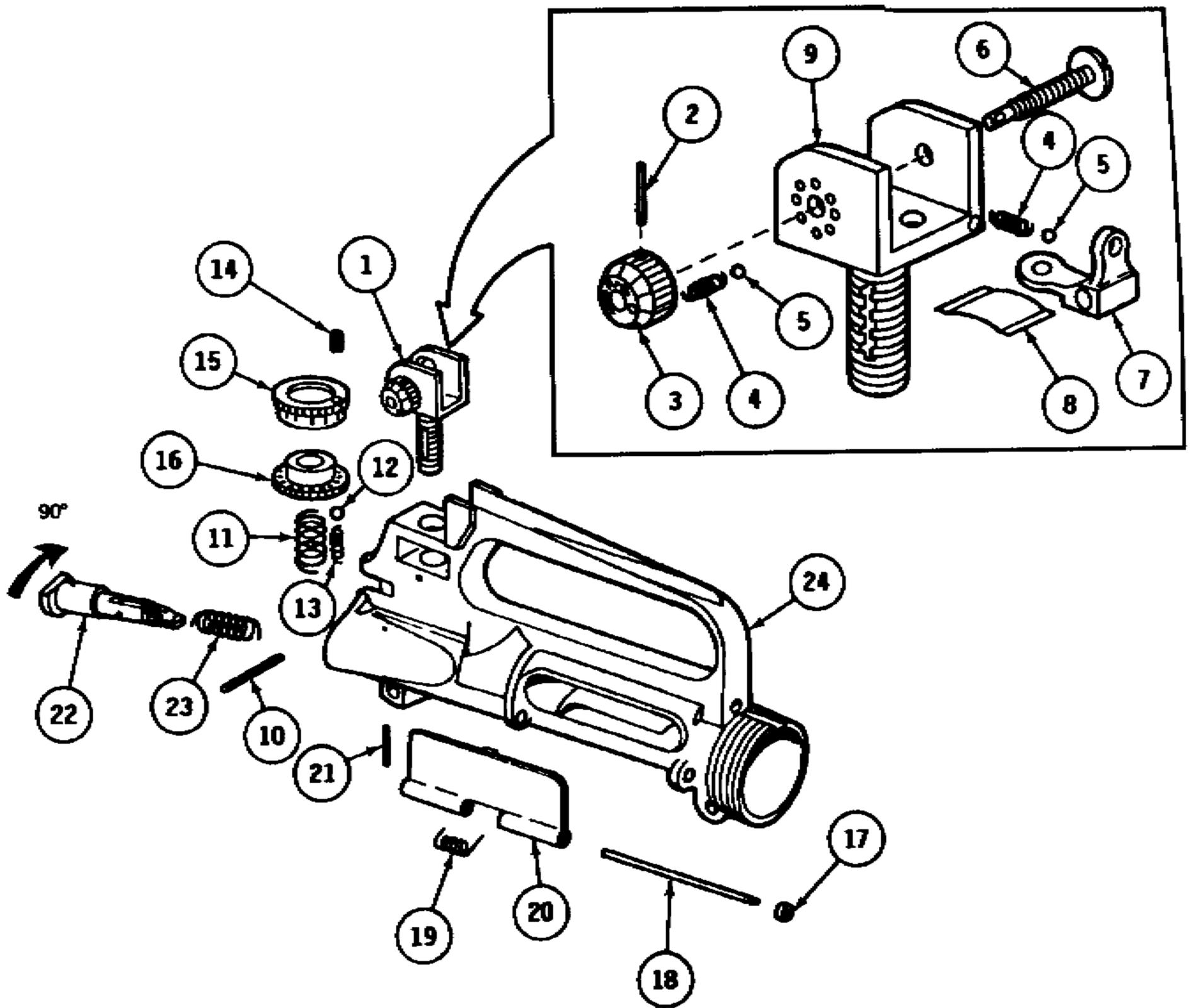
Figure C-8. Upper receiver assembly 9349062 and rear sight assembly 9349072
