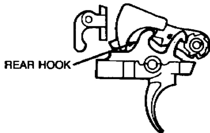
u. Because a stop notch is deeper than the others, it allows the front hook of the burst disconnector further forward than before. This allows the rear hook of the burst disconnector to latch on the rear hammer notch. This holds the hammer fully to the rear even though the trigger is still to the rear. This happens when the burst is over and the firing is stopped.
