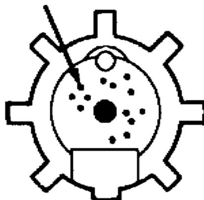
Bolts that contain very small individual pits in a scattered pattern shall not be cause for rejection.
