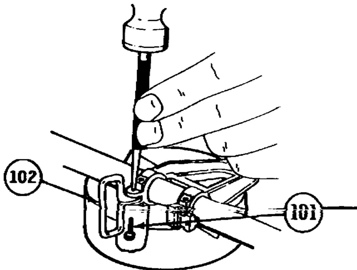
c. Tubular rivet (101) and sling swivel (102)
