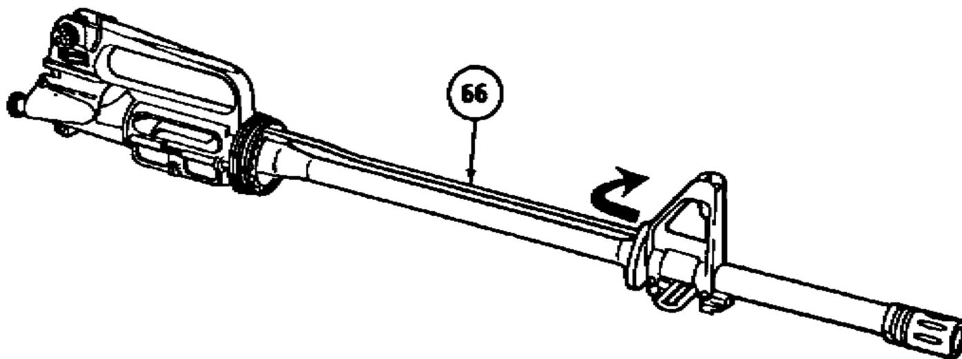
remover fixture, place upper receiver and barrel assembly in vise.
