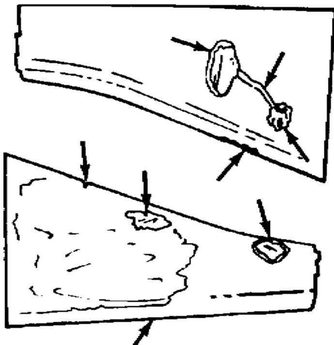
BUTTSTOCK - REPARABLE DAMAGED AREAS
