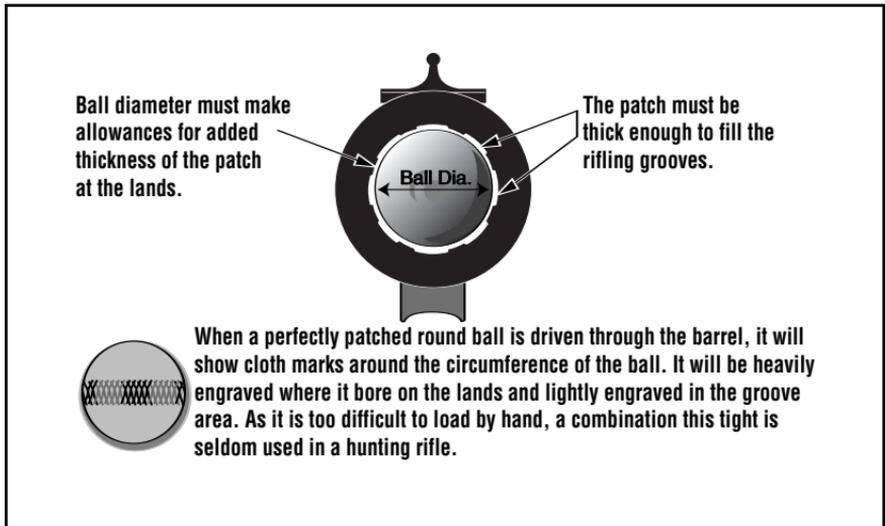
For target shooting, an extremely tight fitting combination of patch and ball is sometimes used. Often a bullet starter, shaped to the contour of the ball, is employed and a hammer is used to start the projectile. Such a combination is, naturally, too difficult to load under field conditions and, therefore, most hunting rifles use a slightly looser fit.
