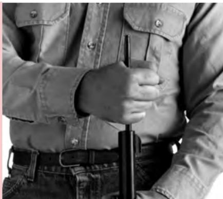
Once the ball has been loaded, it is necessary to carefully mark your ramrod at the muzzle. A reference mark on the ramrod will allow you to ensure that all the future projectiles are seated to the same depth (see Photo “D”).
