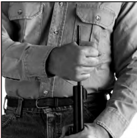
After the bullet is seated tightly against the charge, mark your ramrod in the same manner as previously instructed when loading the round ball.
