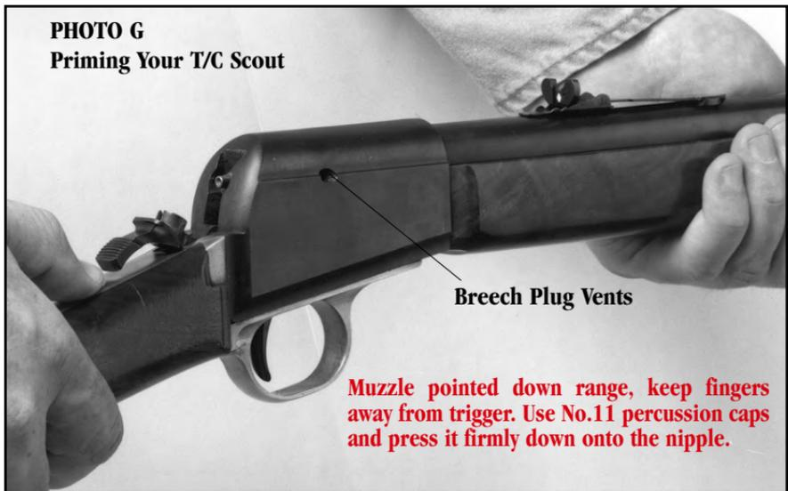
Hold the T/C Scout firmly with the muzzle pointed in a safe direction and **pull the hammer back to full-cock position**. Press the No. 11 Percussion Cap down tightly onto the nipple and the rifle is ready to fire. **RAISE THE T/C SCOUT AND FIRE THE SHOT!**
