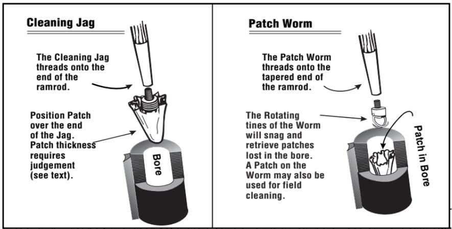
The worm is an extremely important muzzleloading tool and every shooter should carry one in his implement bag. While its prime purpose is to retrieve "lost patches", it can also be used for field cleaning. To do so you simply catch the cleaning patch on the tines of the worm and push it into the bore in the conventional manner.
