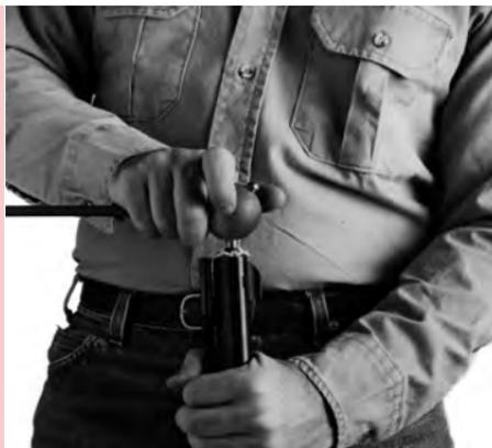
Once the ball is started, reverse the bullet starter, as shown in Photo “B”, and place the rod end on the top of the ball. With a sharp blow of the hand, drive the ball down about four inches into the barrel. The ball and patch have now been formed to the rifling and will (if the bore is not fouled) load easily from this point.
