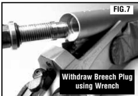
Withdraw Breech Plug using Wrench
