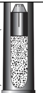
**WARNING: WHEN LOADING T/C'S MAG EXPRESS SABOTS, MAKE SURE THAT YOUR GUN IS UNPRIMED, AND THAT YOUR SABOT HAS BEEN PROPERLY ASSEMBLED. FAILURE TO ASSEMBLE AND LOAD YOUR SABOT CORRECTLY COULD RESULT IN THE BULLET DISENGAGING FROM THE SABOT. THIS COULD RESULT IN AN AIR SPACE BETWEEN THE COMPONENTS. UNDER SUCH A CONDITION, ONE OR MORE OF THE COMPONENTS MAY ACT AS A BARREL OBSTRUCTION AND FIRING COULD RESULT IN INJURY AND/OR DEATH TO THE SHOOTER OR BYSTANDERS AND DAMAGE TO PROPERTY.**
