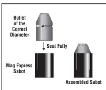
The Assembled Sabot Must Be Seated Firmly On The Powder Charge.
