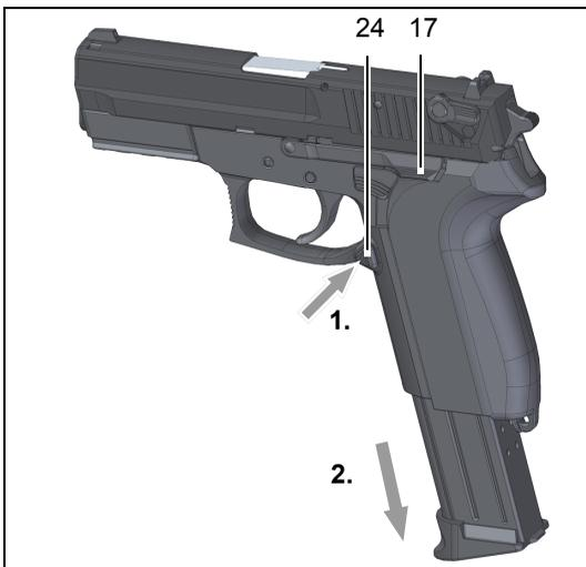
Fig. 4, Removing the magazine
