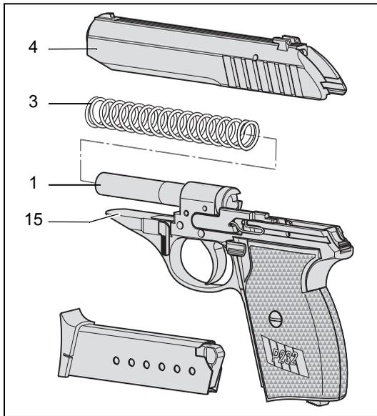
Fig. 12, stripping weapon for cleaning
