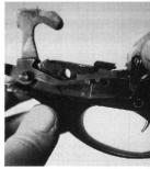
4. To replace the receiver coverplate on the underside, invert the gun and start the plate with its inner surface facing ouward. Press it inward, compressing its rear side wings; then swing it over forward until it can be snapped into its retaining orgoned.
