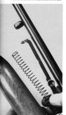
The firing pin is retained by a small cross pin in the larger rear portion of the bolt, and after removal of the pin it can be taken off upward.
