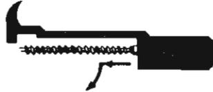
Draw recoil spring guide slightly to rear until it is disengaged from operating slide, and then pull to right and forward and withdraw guide and spring from well in receiver.
