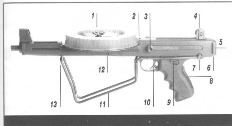
1 - drum spring mechanism, 2 - drum latch, 3 - cocking handle, 4 - adjustable rear sight, 5 - lower sub-assembly latch, 6 - safety button for lower sub-assembly latch, 7 - stock latch, 8 - automatic safety, 9 - manual safety, 10 - trigger, 11 - folding stock, 12 - barrel holder, 13 - folded stock latch. Manipulation with individual operating parts is specified in the next chapter.
