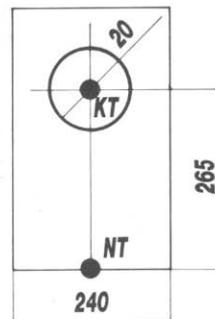
NT-the aiming point, KT- the control point
