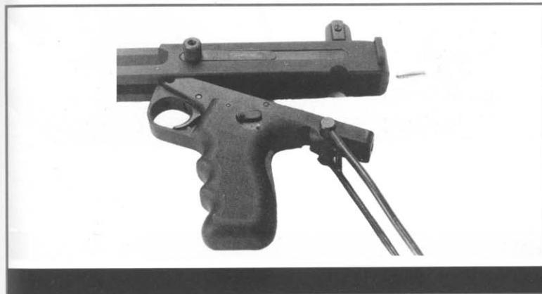
Lower sub-assembly separated from the receiver
