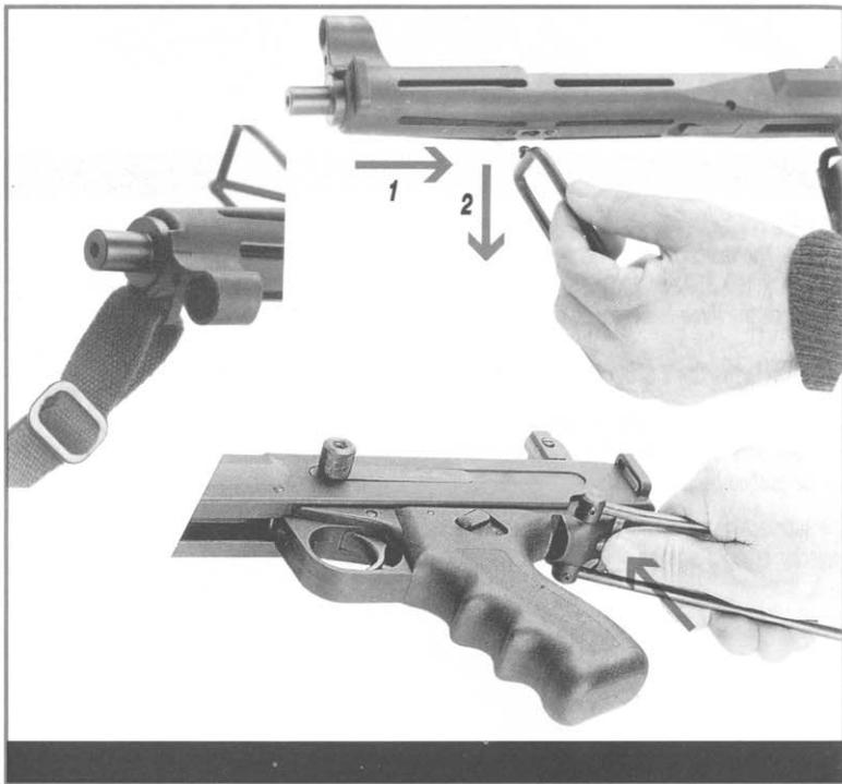
The stock is released by pulling its shoulder end back- and downwards.
