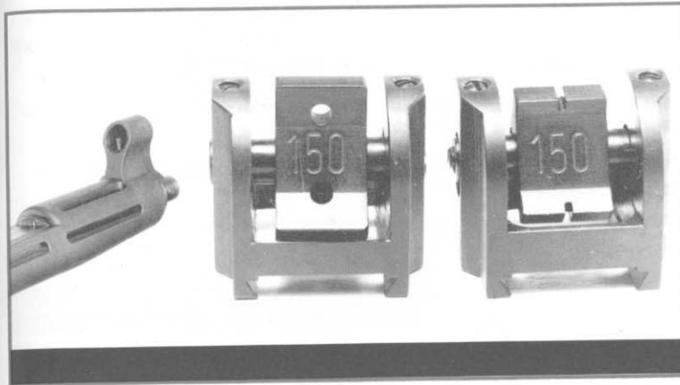
The MGV 176 has a fixed front sight with protective tunnel and the adjustable rear sight in two versions. The rear sight basic configuration has three folding leaves with notches for firing at a distance of 100, 150 and 200 m. These numbers are marked on corresponding leaves. A spring-loaded latch holds the three-leave folding piece in set position.
