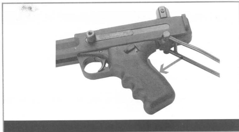
Automatic safety is formed as a squeeze-lever on the back of the grip. The shooter disengages it automatically when correctly holding the gun grip; when he abates the grip, the safety automatically puts the mechanism on "safe". This way the automatic safety prevents activating the gun when it falls down accidentally and in similar situations.
