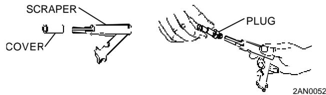
Fold scraper and press point into groove. Turn gas regulator plug clockwise to remove carbon from groove on gas regulator plug.
