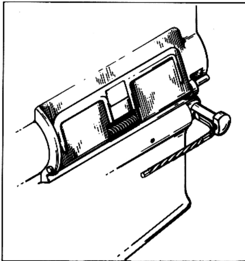
FIGURE A11. PIVOT PIN DETENT DEPRESSOR (P/N 62673).
