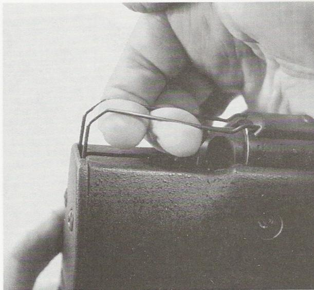
3. Pull the cocking piece guard upward slightly at the rear, just enough to snap it out of engagement with its detent.
