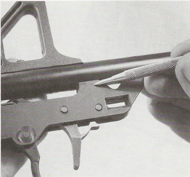
30. The other Allen screw is inside the group, at this location. For access, the safety detent pin and safety-lever pin will have to be removed. With the group removed, drifting out the trigger pin will release the trigger and trigger rod for removal.
