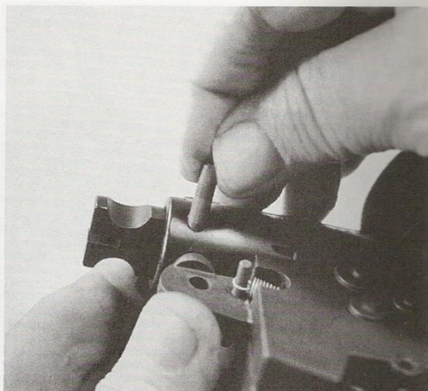
3. When the firing system is in place, remember to reinstall the bolt cross pin before the action is put back into the stock. Also, when the action is in place, remember to push the cocking piece guard back down into locked position.
