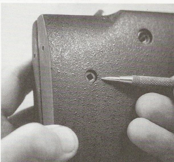
8. With the plunger slightly depressed, remove the square-bit screw that pivots and retains the recoil spring lever. **Caution:** Control the spring.
