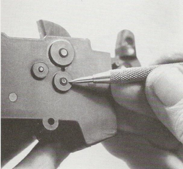
21. The firing system has steel cross pins in a polymer housing, and disassembly should be done only for repair purposes. Without removing the parts, the trigger group is retained by two Allen screws, one visible here. As with the firing system housing, the trigger group has steel pins in a polymer housing, and it should be taken apart only for repair.
