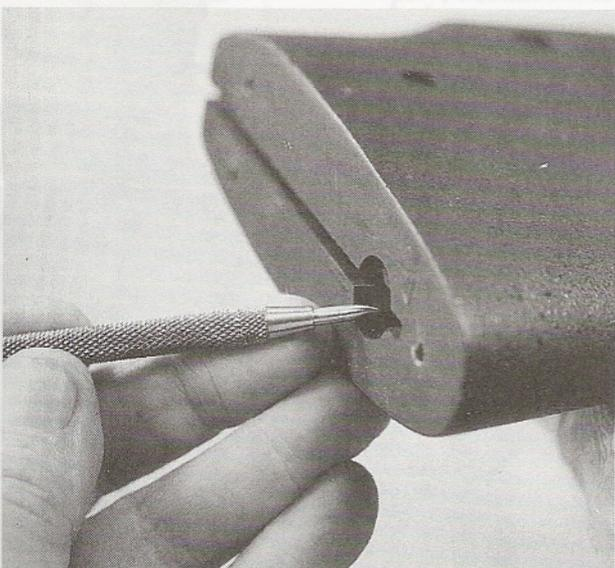
7. Removal of the buttplate will give access to the recoil spring lever, the recoil spring and its plunger. If this system is to be taken out, it will be necessary to depress and restrain the recoil spring plunger with a tool, at the point shown.
