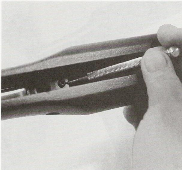
11. The trigger guard is retained on the inside of the stock by two Phillips-type screws. When these are taken out, the guard is removed upward.
