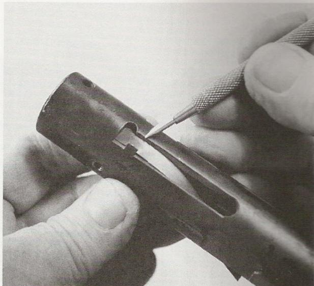
2. Re-hook the trigger rod and grip safety rod to their bars in the firing system before the system housing is swung back upward into place. The proper arrangement is shown.
