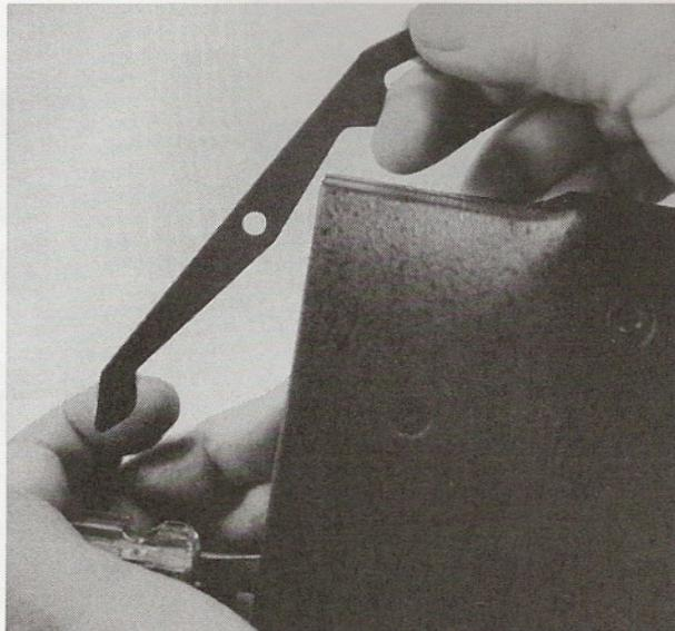
10. Ease the spring tension slowly and remove the plunger and spring toward the rear.
