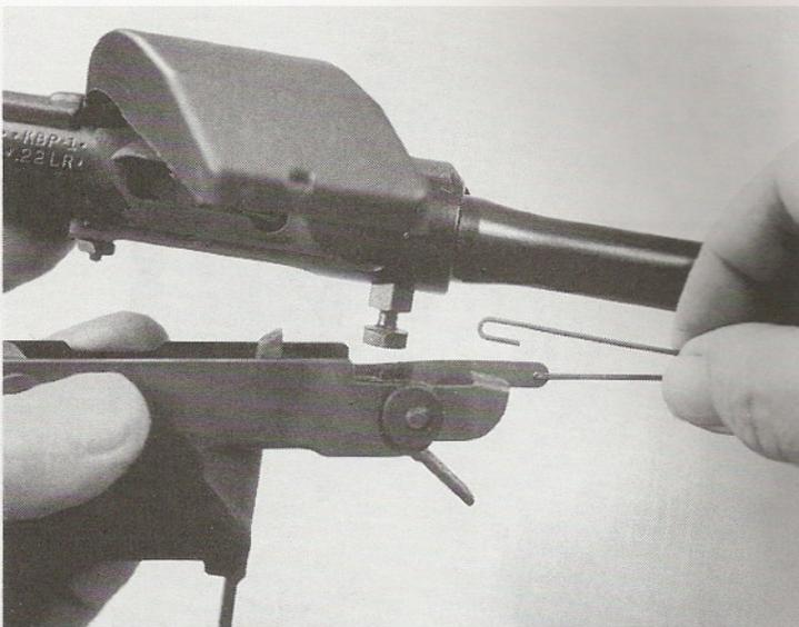
**15.** Move the system slightly forward and unhook the trigger rod from the trigger bar/disconnector.
