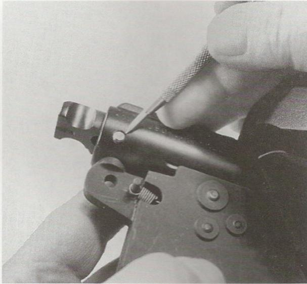
**14.** Pull the firing system housing downward at the rear, as shown.
