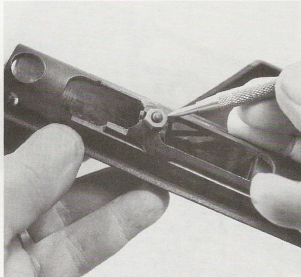
31. The combination ejector and bolt guide is retained on the underside of the receiver by a hex-nut. The part is moved inward for removal.
