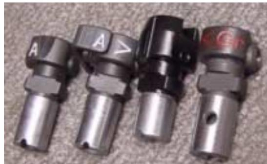
Different ammunition has different pressure curves, so you must experiment with each type of ammo you use. The higher the number (the more gas bleeding off), the less violent the recoil and the less
