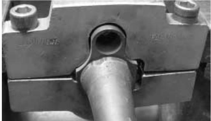
Also – turning the receiver makes it harder to see where top dead center is. If it won't turn far enough, unscrew and take more material off the shoulder. If it goes too far, remove the barrel, degrease, and peen the shoulder with a hammer all the way around. Screwing the old receiver stub part way on will give some protection to the threads if you miss with the hammer.
