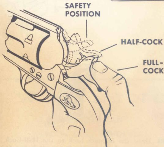
3. **FULL-COCK**—with the hammer all the way back and the revolver ready to fire.
