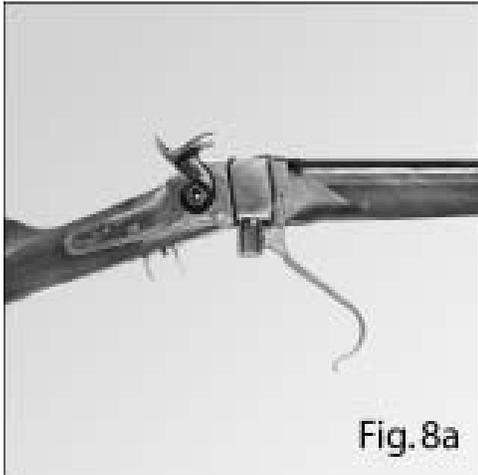
To load the rifle, first point the rifle downrange in a safe direction. Place the rifle on safe by placing the hammer in the half-cock position. **Make sure you have read, understood, and practiced the safety on procedure in the SAFETY section on this manual.** Next, extend the lever downward, fully opening the breech (Fig. 8a). Carefully insert one cartridge of correct caliber completely into the barrel chamber (Fig. 8b) and close the action. You are now ready to fire the rifle.
