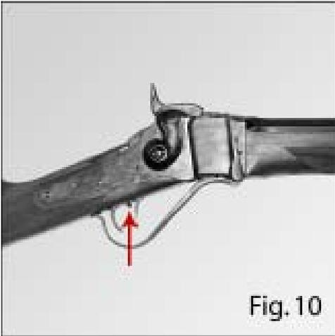
until the desired trigger pressure is obtained (Fig 10). **ALWAYS ADJUST THE SET TRIGGERS WITH AN UNLOADED RIFLE!** Use a snap cap or empty case in the chamber when adjusting, so the firing pin has something to contact when the rifle is fired. If more than 5 shots are required to adjust the triggers, use a different empty case.
