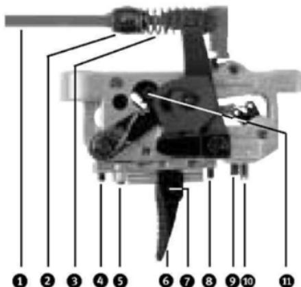
Adjustment of first stage with set screw No. 4:
