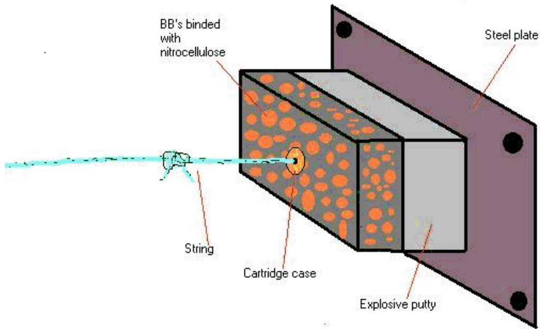
This device contains approx. 300 BB's in front of around 20 grams of explosive. As a matter of interest proper claymores contain 700 steel balls in front of 700 grams of C4.
