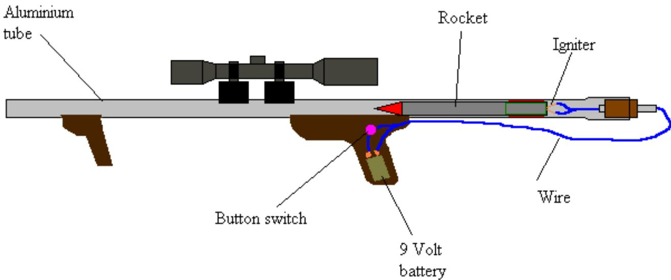
The rocket is powered by a bought estes D class engine, these can be found in most hobby shops however are rather expensive at around \$7-8 Australian per shot, trying to improvise a homemade rocket engine only increases the already high risk of an accident.
