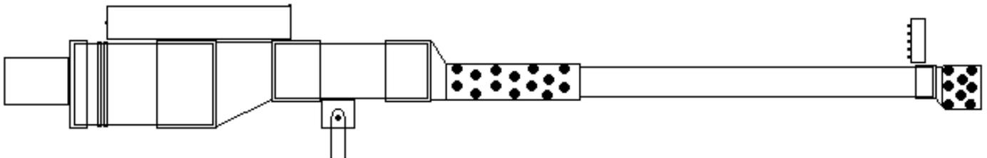
Making a sight for the gun proved more difficult, as it seemed nothing would work, i tried both a scope and conventional open sights but proved unreliable at best. What i settled on was a combination of both, it combines both the crosshairs of a scope and the sighting plain of open sights along with further horizontal crosshairs near the muzzle to choose the range. (no its not as complicated as it seems.. really)..
