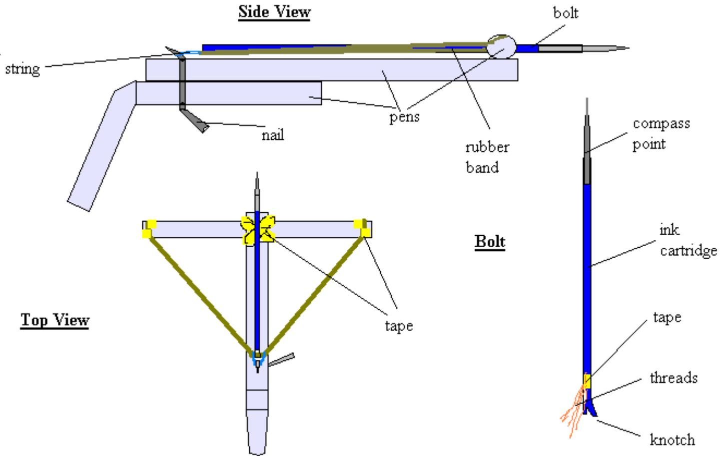
The pens are all taped together. The handle is heated over a heater until it can be bent down. To arm the weapon the rubber band is pulled back and the string loop is put around the nail, the knotch in the bolt is then pushed onto the rubber band inbetween the two knots from the string. To fire the nail is pulled back and the string slips off the top of the nail.
