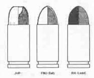
In this case, only the FMJ(Ball) round is a suitable choice. The round nose lead is just too soft, and the JHP is even worse. The .45 ball ammo is an excellent load, if one could only get it moving fast enough. This point should not be lost on those of you who have a .45 Thompson submachine gun. The muzzle velocity of the round leaving that weapon is much higher than when it leaves the .45 handgun.
