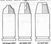
The answer here is the .38 Super SWC, and the .45 ACP WC. The hollow point on the .40 S&W JHP will cause this round to smooth out like a pat of butter when encountering Kevlar armor. Now consider this series of .45 caliber bullets:
