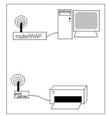
Figure 22-5: After setup, the print server can communicate wirelessly.
