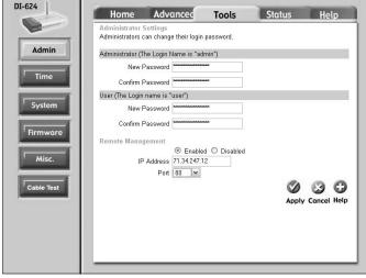
Figure 1-10: Only a computer at IP address 71.34.247.12 can access this router.
