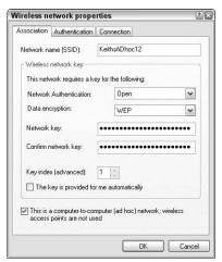
Figure 13-1: Create a SSID and WEP key for your ad hoc network.
