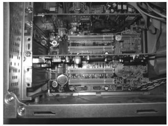
Figure 18-1: Four open PCI slots.
