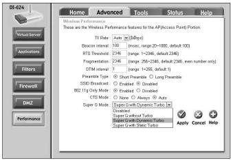
Figure 10-3: Enable the access point's accelerator technology.
