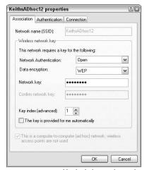
Figure 13-14: Double-check the WEP key and SSID.
