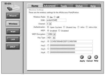
**Figure 6-7:** Enable WEP encryption.
