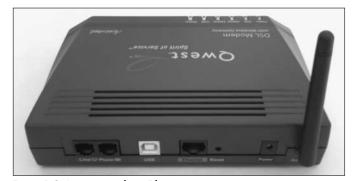
Figure 1-2: Access point with one Ethernet port.
