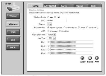
Figure 1-7: The radio and SSID controls.
