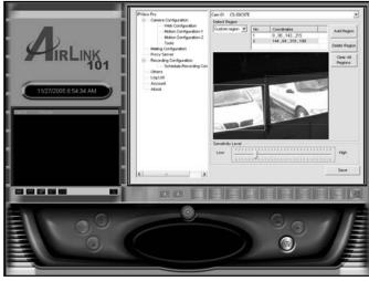
Figure 25-6: Set up motion detection on the camera.
