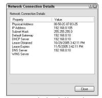
Figure 8-10: The Physical Address is this card's MAC address.
