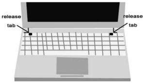
Figure 5-1: The keyboard release tabs.
