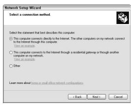
Figure 2-8: Set up ICS on the computer.
