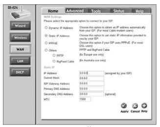
Figure 2-13: Some ISPs assign a static IP address.
