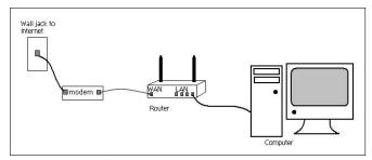
Figure 1-3: Temporarily connect the WAP to a computer.
