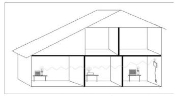
Figure 10-9: A range extender increases the range of your Wi-Fi network.
