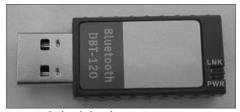
Figure 14-1: This Bluetooth adapter plugs into a USB port.
