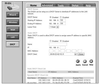
Figure 2-5: Enable the router's DHCP server.
