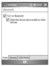
Figure 14-13: Enable the Bluetooth radio and discovery.
