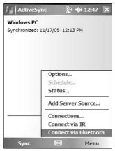
Figure 15-5: Configure ActiveSync to connect via Bluetooth.
