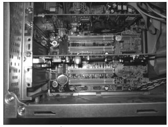
Figure 3-1: Four empty PCI slots.
