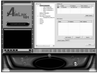
Figure 25-5: Configure the camera's recording software.
