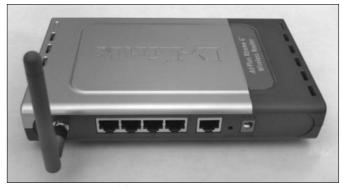
Figure 1-1: Access point with four Ethernet ports.
