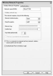
Figure 3-5: Set the SSID and network keys.
