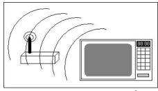
Figure 10-6: Microwave ovens cause Wi-Fi interference.
