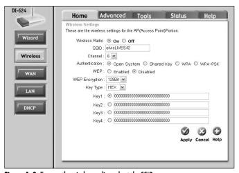
Figure 1-8: Turn on the wireless radio and set the SSID.
