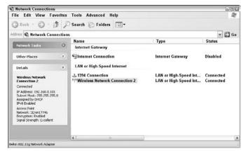
Figure 9-5: Determine a PC's IP Address.
