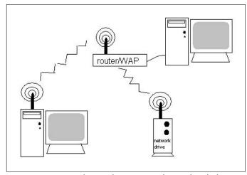
Figure 19-1: Some network storage devices connect to the network wirelessly.
