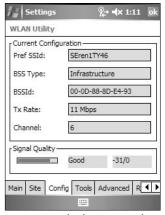
Figure 10-1: This device is networking at 802.11b speeds.
