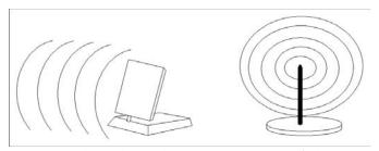
Figure 10-7: A directional antenna lets you increase range in a specific direction.
