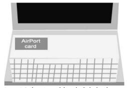
Figure 5-2: The AirPort card slot under the keyboard.
