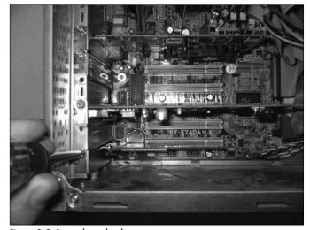
Figure 3-2: Secure the card in the case.
