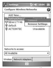
Figure 13-6: Connect to an ad hoc network from a Pocket PC.
