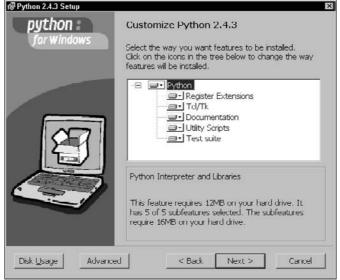
Figure 18-4: You can exclude parts of Python from the initial installation.
