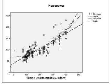
Figure 14-21: Curves generated from the relationships of engine displacement to horsepower.
