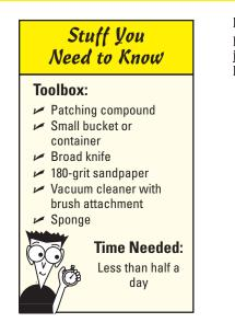
Repairing narrow cracks in drywall requires a thin mix of patching compound (look for one that you mix with water). After the application of just a few thin layers, all you have to do is sand, prime, and paint. Problem solved!
