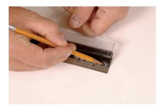
2. Lay the rubber blade of the shower squeegee against a ruler and use a pencil to mark off the placement of notches as desired for your design. You may want small notches for very fine lines, or you may want to mark wide, widely spaced notches for bolder lines.
