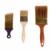
Figure 1-5: A 2-inch angled sash brush, a small chip brush, and a 3-inch flat sash brush.
