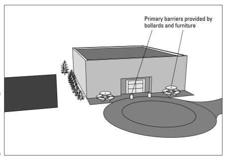
Figure B-2: Front entrance, protected by bollards and anchored furniture.
