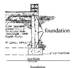
**foundation 1.** The masonry or concrete portion of a structure usually below surface grade that transmits weight (load) from the structure above. **2.** The earthen material or rock upon which a structure transmits its load and depends upon for stability.
