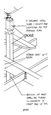
**post and board fence** A wood fence design of posts and rails spanning between them with space between the rails.
