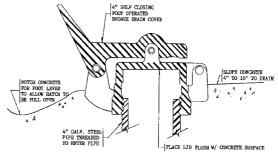
drain hatch detail
