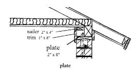
**plate bolt** A bolt that secures the **plate** on top of a foundation or wall and is usually embedded in the masonry or concrete.
