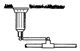
swing pipe sprinkler head installation with a funny pipe (swing pipe) connection
