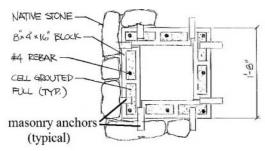
masonry column (plan view section)
